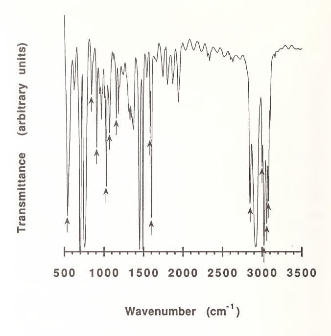
Figure 1. Spectrum of polystyrene film showing locations of certified absorption peaks.
