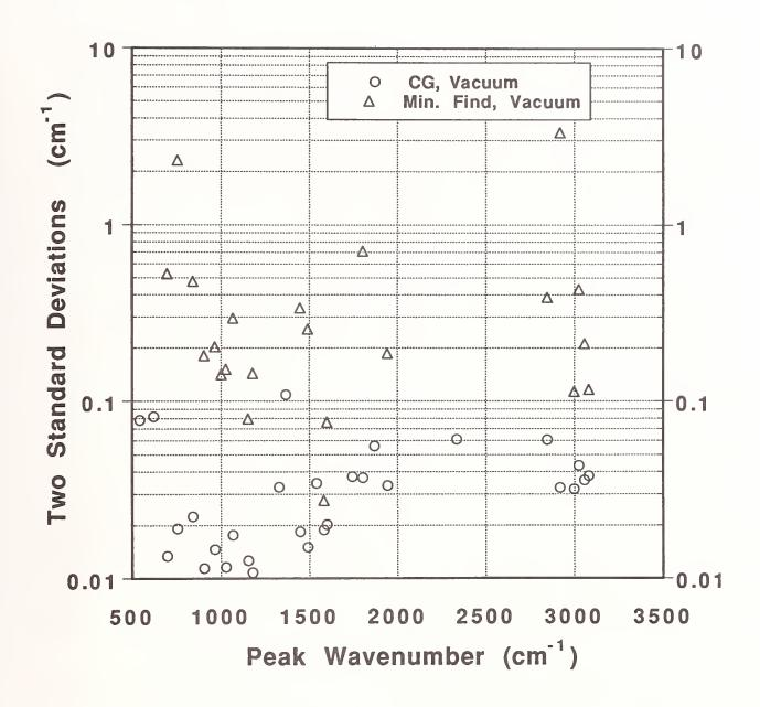
Figure 3a. Comparison of peak positions for polystyrene absorption bands, as determined by center-of-gravity and minimum-find techniques: two standard deviation values.
