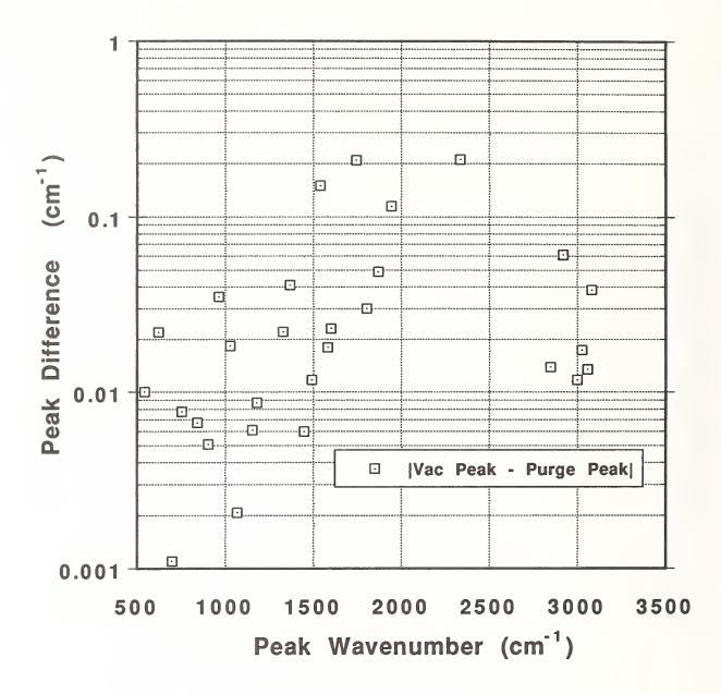
Figure 2b. Comparison of peak positions for polystyrene absorption bands, made under vacuum and purge conditions: peak position differences.
