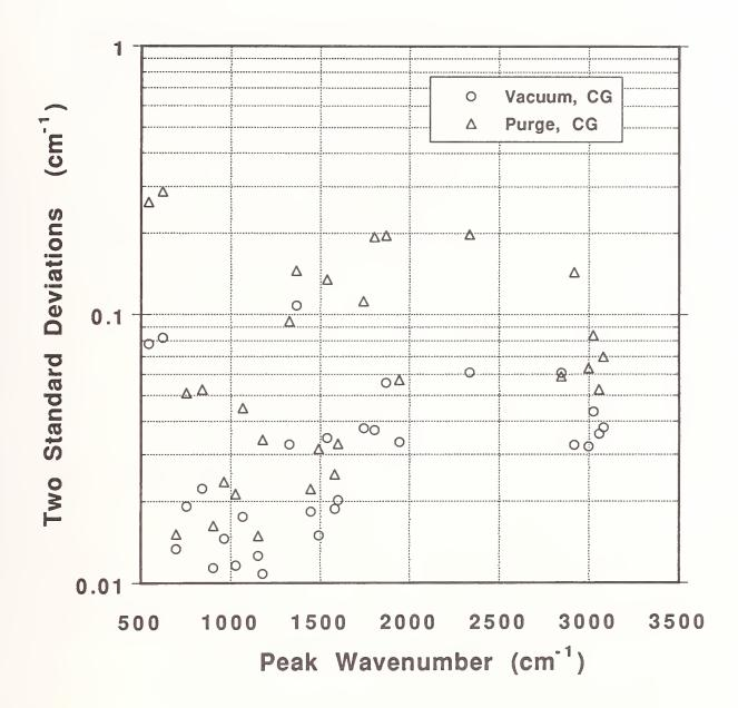
Figure 2a. Comparison of peak positions for polystyrene absorption bands, made under vacuum and purge conditions: two standard deviation values.
