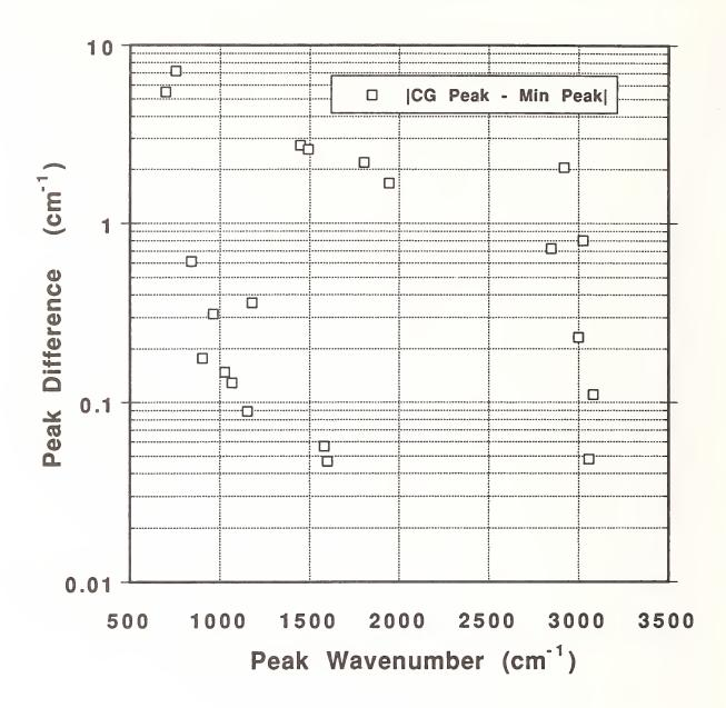
Figure 3b. Comparison of peak positions for polystyrene absorption bands, as determined by center-of-gravity and minimum-find techniques: peak position differences.
