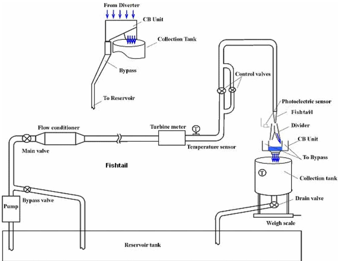
**Figure 3.** Sketch of the Arrangement of Equipment in the WFCF 3700/100 System.
