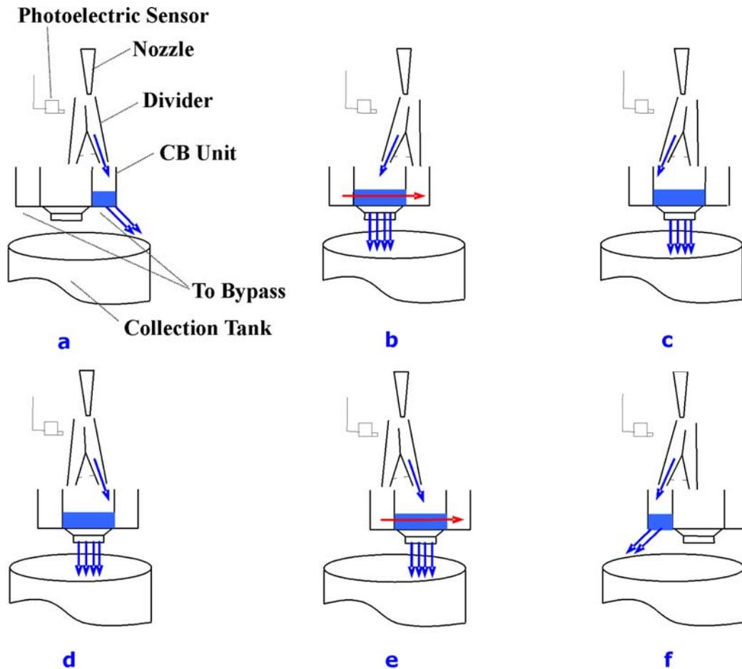
**Figure 6.** Collection-bypass Cycle.
