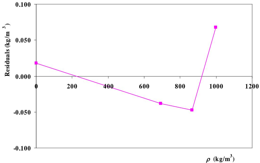
**Figure 16.** Residuals from the Densimeter Tests.
