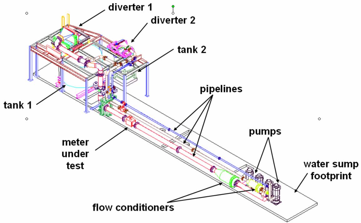
**Figure 1.** A Perspective Drawing of NIST’s Water Flow Calibration Facility.
