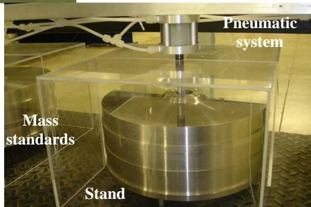
**Figure 8.** Weighing System for WFCF 3700/100 and Mass Standards
