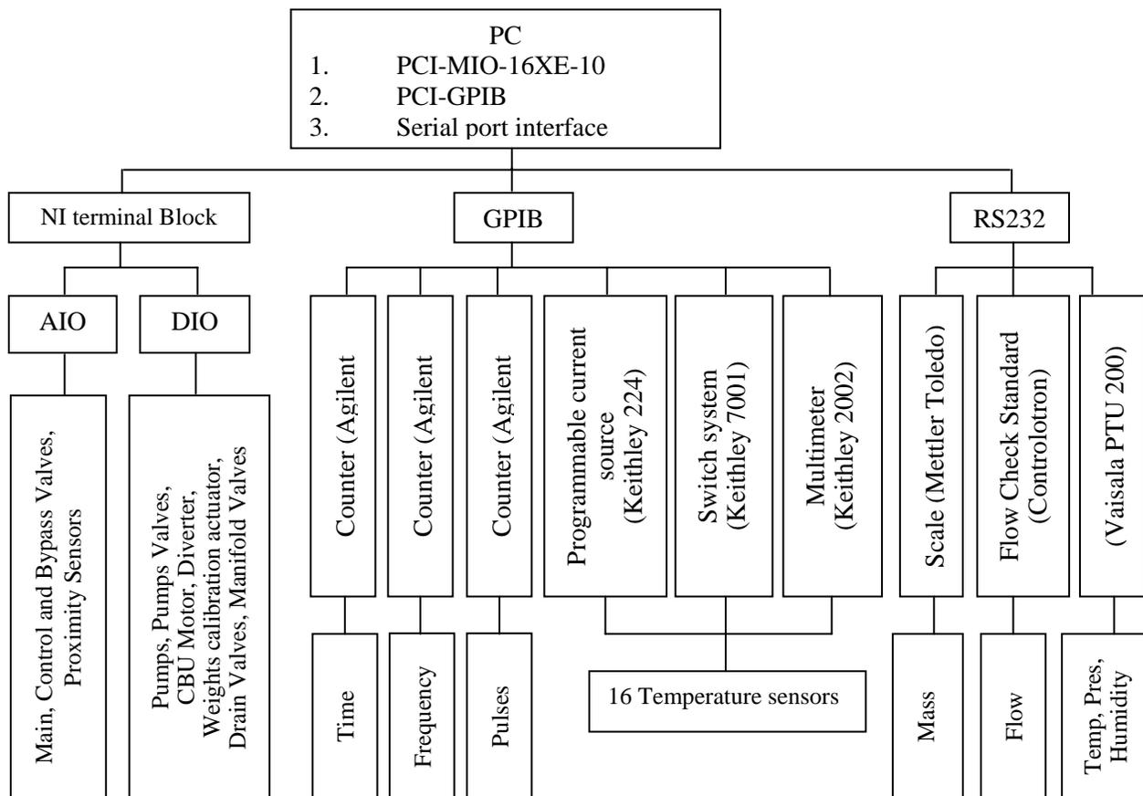
**Figure 22.** Data Acquisition Chart for the Facility
