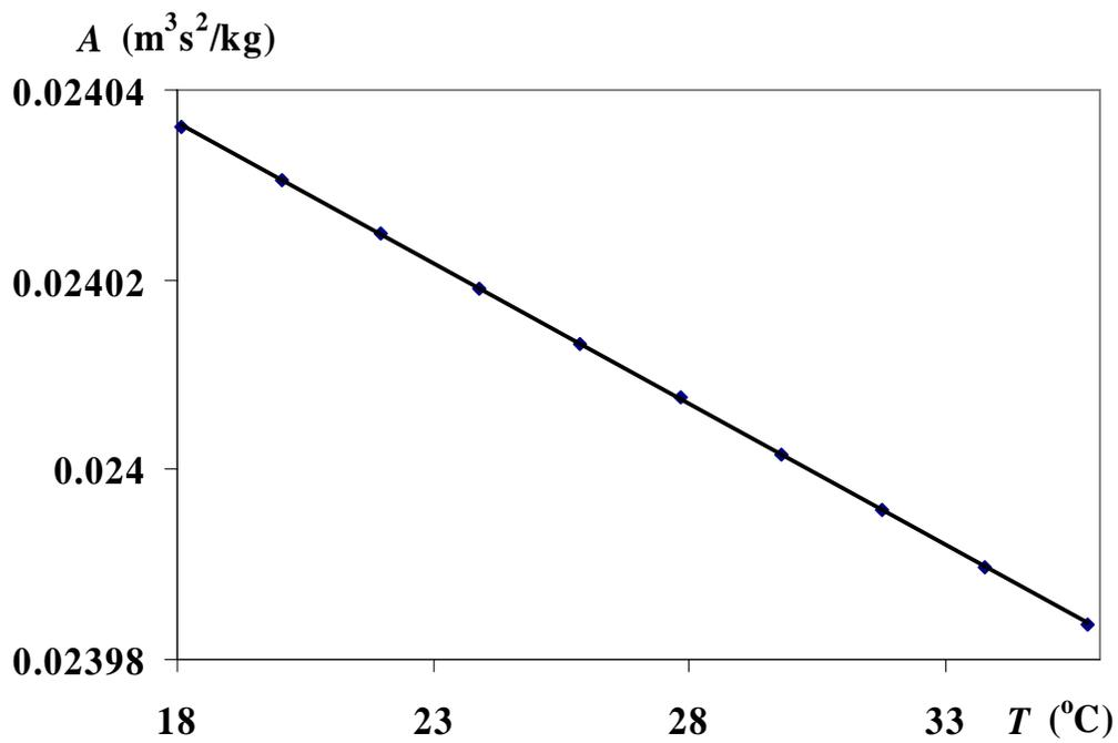
**Figure 17.** Temperature Dependence of the Coefficient,  $A$
