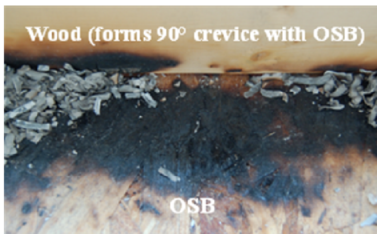
Figure 12 Images obtained (top view) for crevice filled with paper tests using 10 x 10 (2.0 mm) mesh.
