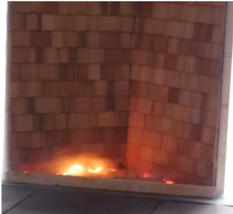
Figure 17 Images of untreated cedar shingle siding ignited under firebrand attack at a wind tunnel speed of 7 m/s.
