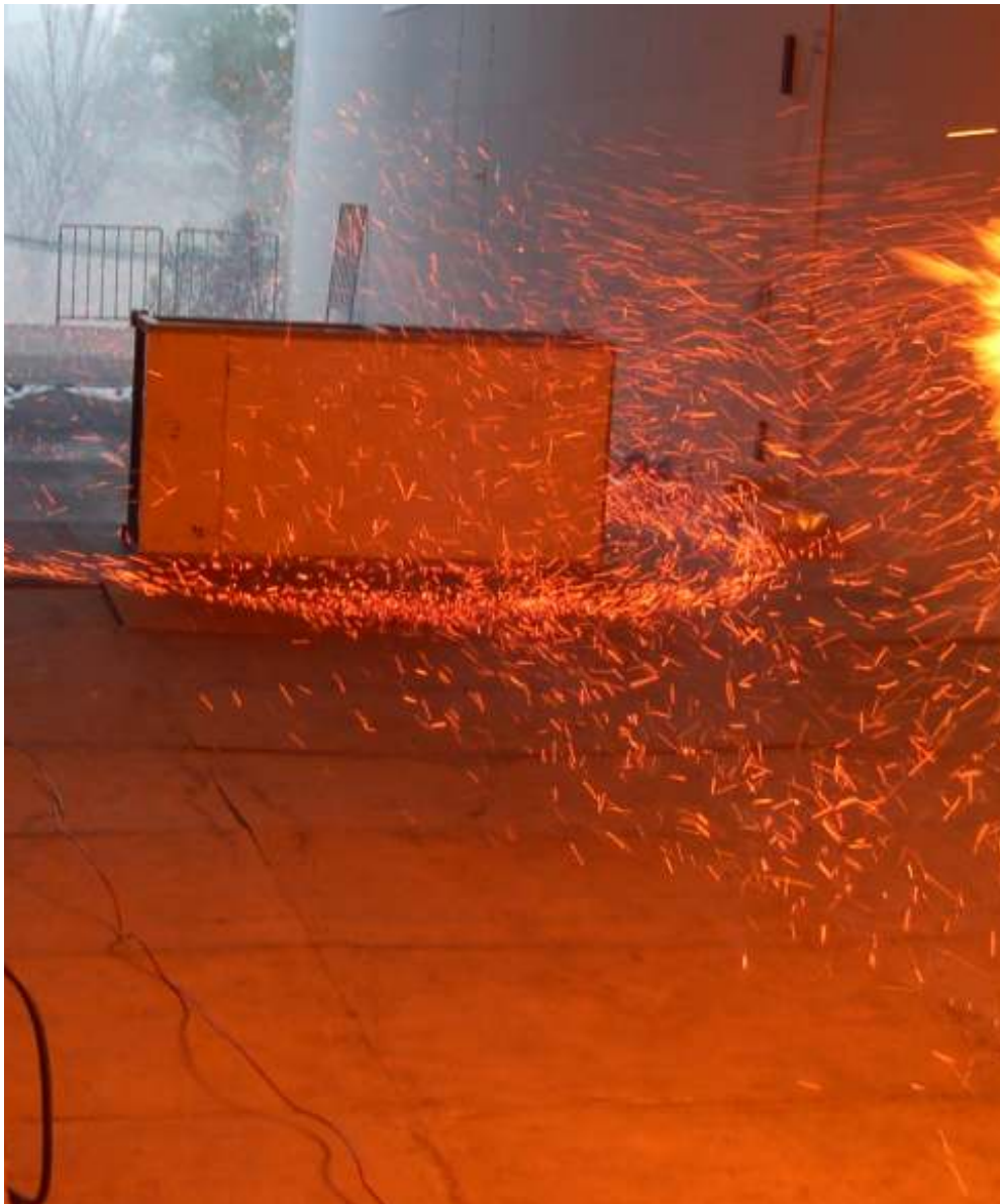
Figure 22 Image of firebrands flowing around one of the obstacles used.
