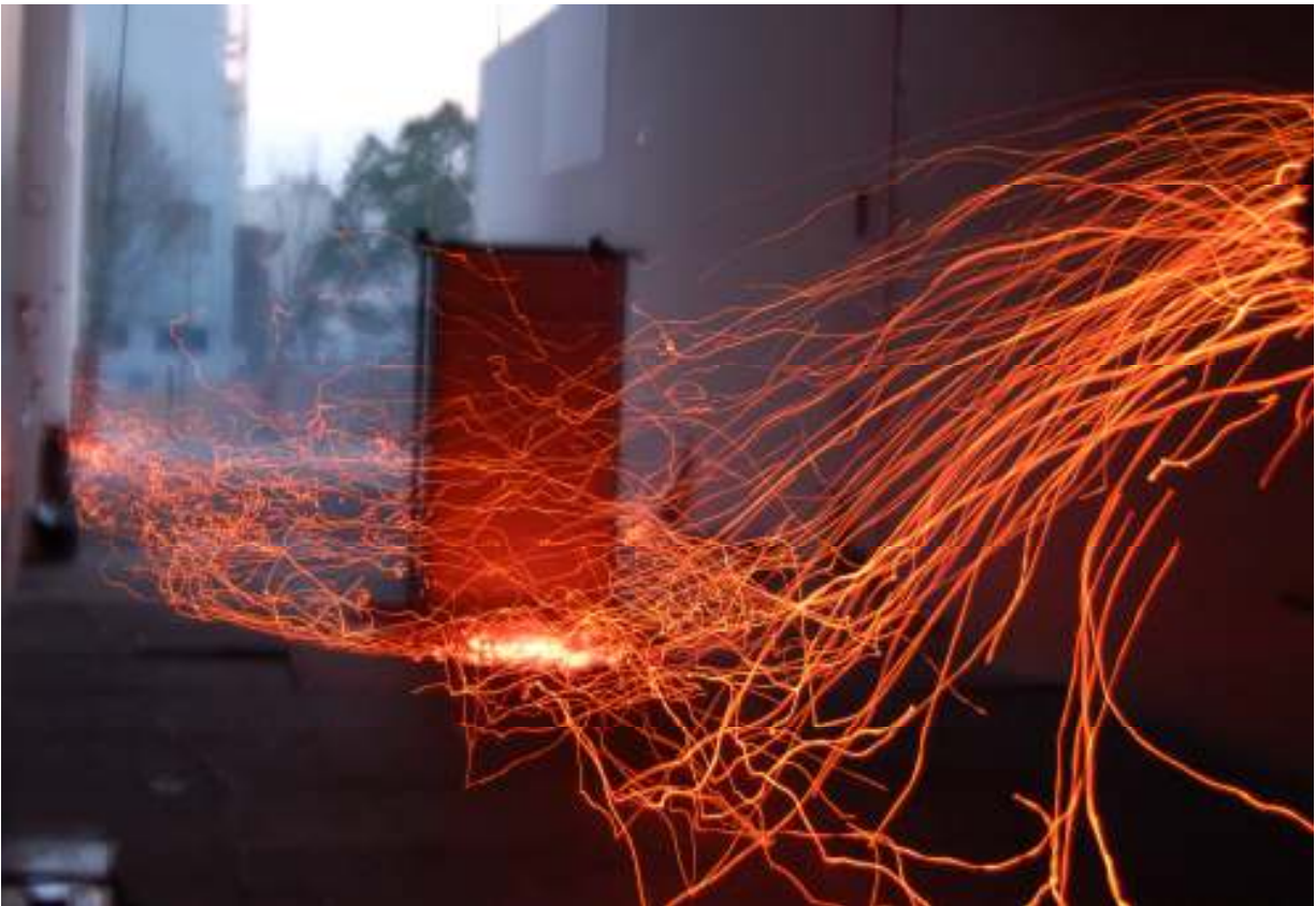
Figure 23 Photograph taken by increasing the exposure time on the camera to visualize the firebrand streaklines or flow over the obstacles.
