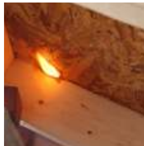
Figure 5 Images of experiments conducted using OSB/CT without bird stops installed. Intense SI was observed within the OSB base layer and eventually FI was observed. The wind tunnel speed was 7 m/s and the Firebrand Generator was located 2.0 m from the CT roofing assembly.
