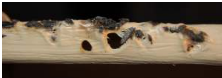
Figure 15 Image of vinyl siding (from bottom) after firebrand exposure at 7 m/s.
