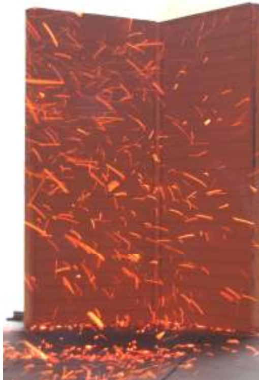
Figure 14 (b) Picture of vinyl siding corner assembly under firebrand bombardment.
