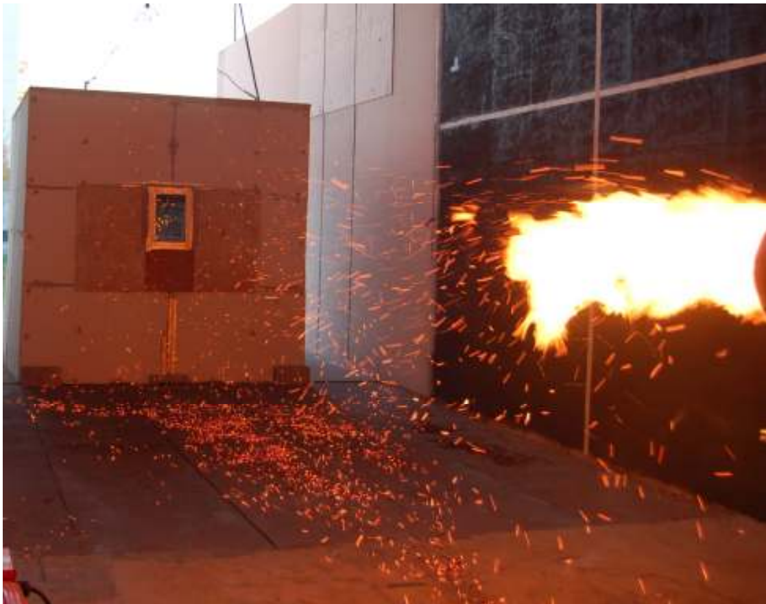
Figure 10 Typical experiment using NIST Firebrand Generator at BRI's FRWTF. The mesh installed in this experiment was 20 x 20 (1.04 mm), the wind tunnel speed was 7 m/s, and the Firebrand Generator was located 7.5 m from the structure.
