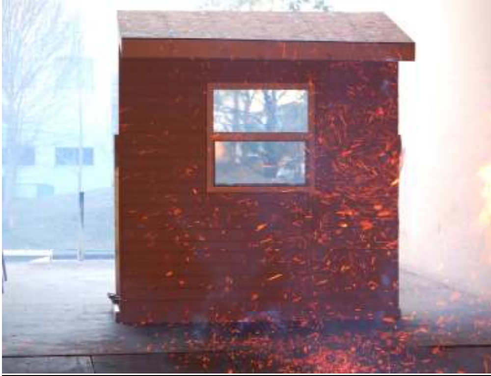
Figure 21 Picture of wall/eave assembly fitted with a vertically sliding, double hung window exposed to firebrand showers at a wind tunnel speed of 9 m/s.
