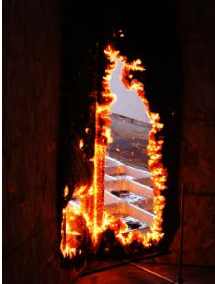
Figure 30 Firebrand generation from a burning re-entrant corner at 8 m/s applied wind. Firebrands are produced on the backside of the assembly and are collected using an array of water pans downstream.
