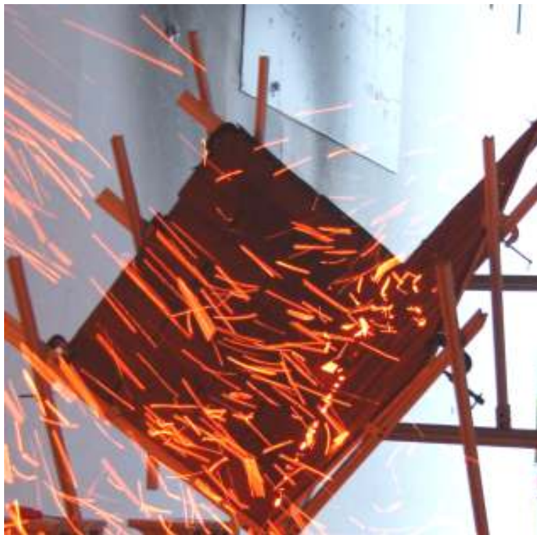
Figure 7 OSB base layer, tar paper, and asphalt shingles; Angle of 90°-no ignition observed. The wind tunnel speed was 7 m/s.
