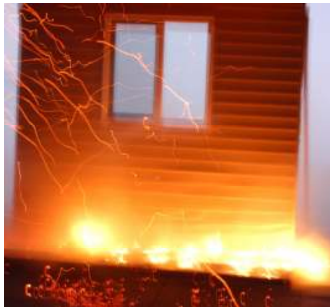
Figure 16 In the top image, firebrands have caused smoldering ignition in the mulch bed. In the bottom image, smoldering ignition has transitioned to flaming ignition and the wall assembly has ignited.
