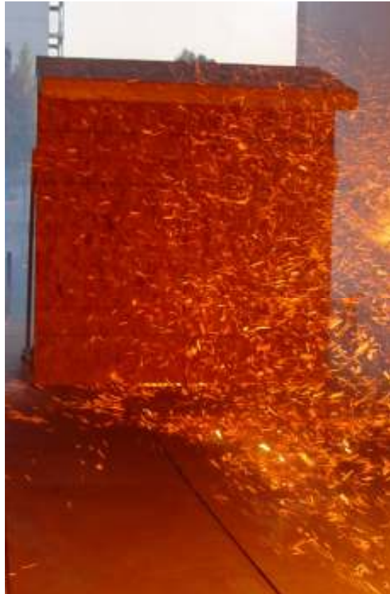
Figure 19 Image of wall fitted with eave under firebrand bombardment.
