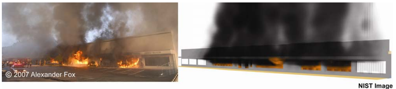
Figure K-27. Comparison between photo and rendered image from the simulation at 1884 s (7:42:17 p.m.). The view is of the front of the main and west showrooms. Photo used with permission of Alexander Fox.
