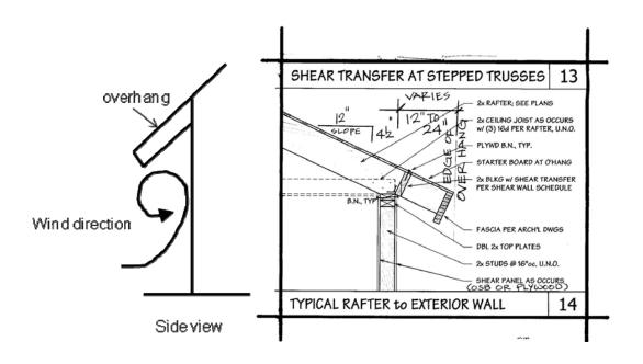
Fig. 3 Side view of standard eave assemblies.
