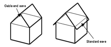
Figure 2 Schematic of eave configurations.
