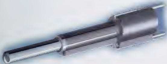
New cold source "thimble". The cold source chamber resides within the left end of this thimble, and cold neutrons pass out to the right.
