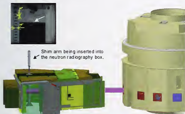
FIGURE 1: Shim arm Cadmium burnup monitored by neutron radiography. As an example of resolution, the inset radiogram shows an edge of the Cd layer.
