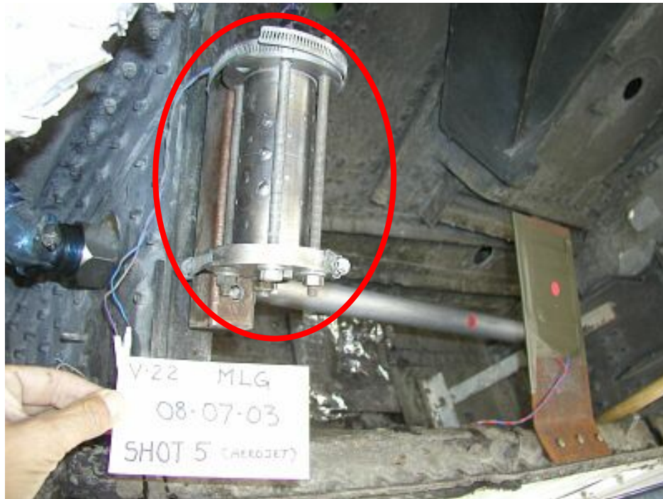
Figure 9–44. SPGG Installed in Sponson Test Article for Live-fire Demonstration. 46 (Photograph reprinted with permission of the Naval Air Systems Command.)
