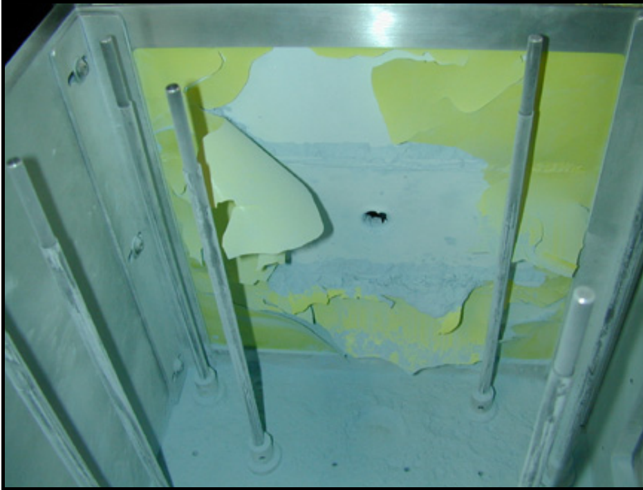
Figure 9-4. Test Example of Significant Panel Fracture and Material Loss.
