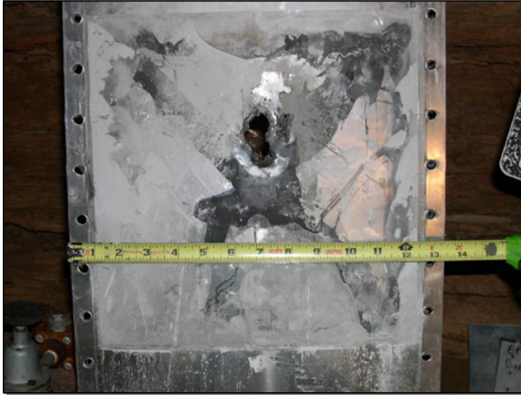
Figure 9–29. Post-Test Damage Image of EPP-06 Enhanced Powder Panel.
