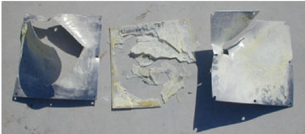
Figure 9–13. Entire Contents of Enhanced Powder Panel Released During FAA Test in Which the Fire Was Prevented.
