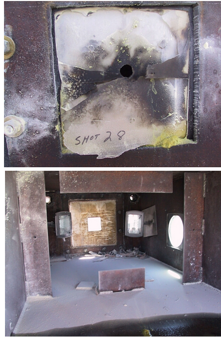
Figure 9–12. Comparison of Commercial and Enhanced Powder Panel Agent Release in JTCG/AS Dry Bay Fire Extinguishing Testing.
