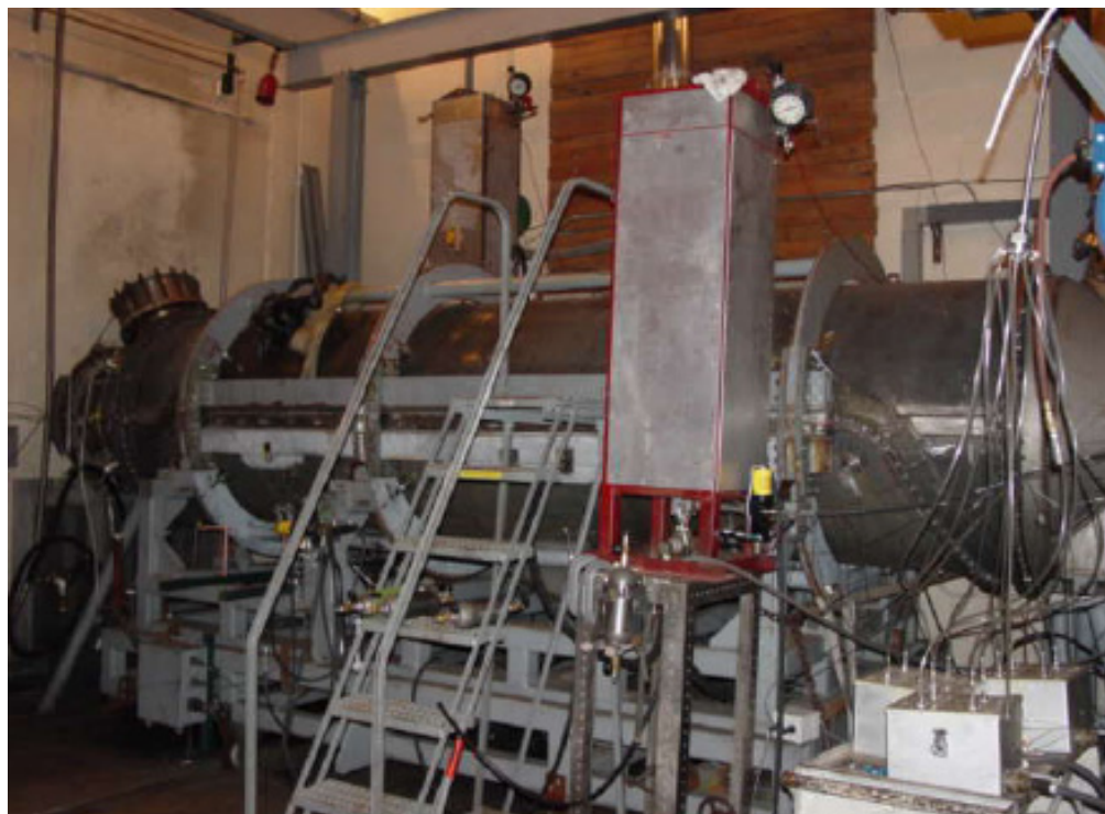
Figure 11-4. Vertical Extinguisher Unit Attached to the Nacelle Fixture.
