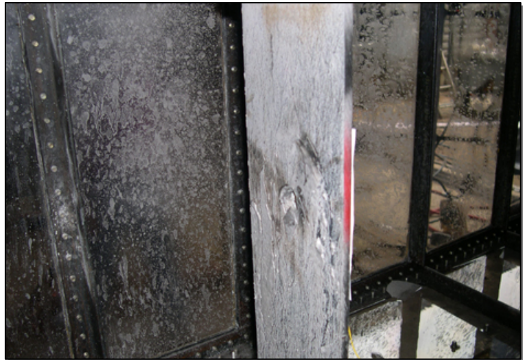
Figure 9–28. Powder Dispersion on Striker Plate and Side Lexan Panel.
