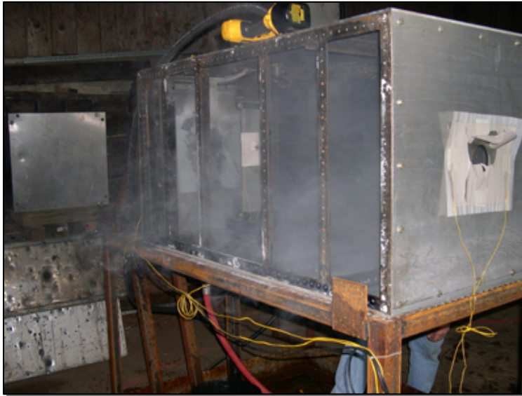
Figure 9-32. Powder Evident in Dry Bay More Than 5 min after EPP-09 Test. (Side Wall Removed)
