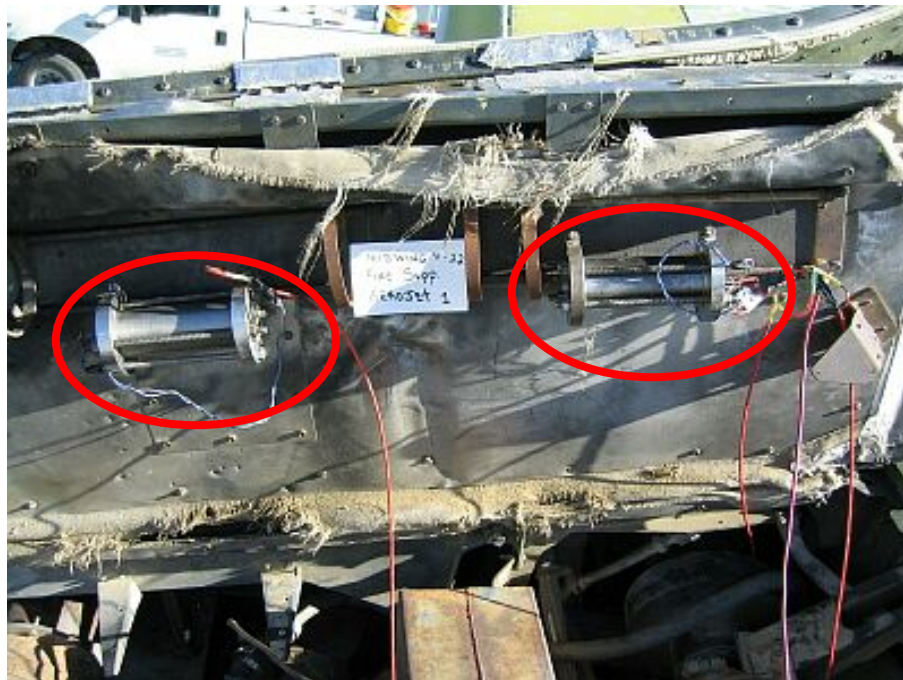
Figure 9–45. SPGGs Installed in Mid-wing Test Article for Live-fire Demonstration. 47 (Photograph reprinted with permission of the Naval Air Systems Command.)
