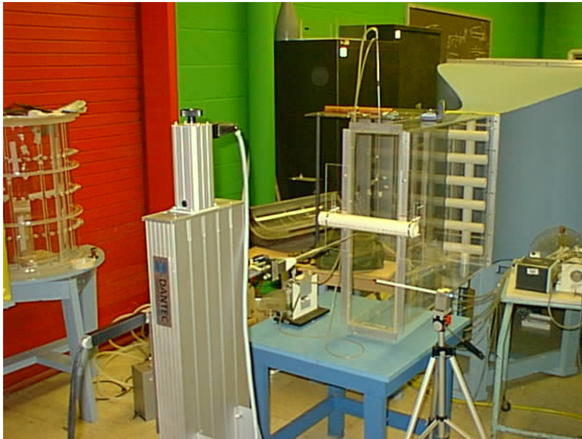
Figure 8-85. Low-speed, High-turbulence, Open Jet USNA Wind Tunnel.
