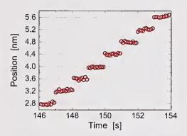
Figure 4. Individual 0.4 nm steps measured in a new differential back-focal-plane detection, optical-trapping microscope. The fact that the data points lie on lines demonstrates that 0.1 nm stability is achieved over several seconds.
