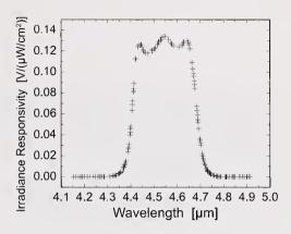
Figure 1. Spectral irradiance responsivity for an InSb radiometer measured on IR-SIRCUS.
