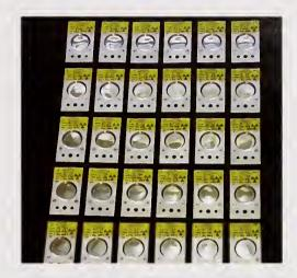
Figure 2. Radioactive test sources developed at NIST for the testing and evaluation of radiation detectors to be used by first responders.
