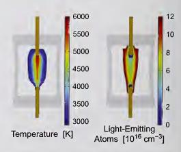
Figure 8. X-ray mapping of plasma properties in a metal-halide lamp. a) Temperature distribution from x-ray absorption imaging. b) Spatial distribution of atoms capable of emitting light from x-ray induced fluorescence.
