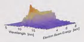
Figure 9. EUV spectra of xenon, taken on the NIST EBIT. The variation of spectral features as a function of the electron beam energy provides valuable data for benchmarking models of the atomic processes.
