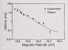
Figure 1. Lifetime of the tunable, molecular bound state of the  $^{85}$ Rb $_2$  dimer as a magnetic field B is varied near a scattering resonance at 15.2 mT. The rapid increase in lifetime is due to the dramatic increase in the size of the weakly bound atom-pair, to hundreds of nanometers, as the field gets closer to the resonance value.
