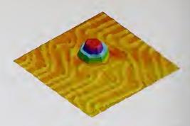
Figure 6. Scanning tunneling microscope image  $(32 \text{ nm} \times 32 \text{ nm})$  of a 9 nm mound, two atomic layers high, created by the impact of a single  $Xe^{44+}$  ion on the Au(111) surface. The mound has relaxed to a perfect hexagon, and the "herring-bone" reconstruction in the background has rearranged around the mound to minimize surface energy.
