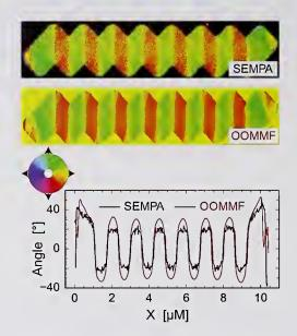
Figure 3. SEMPA image of a zigzag magnetic sensor element, compared with the OOMMF micromagnetics simulation. Line scans through the centers of the elements show the magnitude of the magnetic oscillations.
