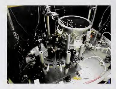
Figure 3. Vacuum goniometer for the measurement of the spectral emittance of specular samples as a function of temperature and angle.
