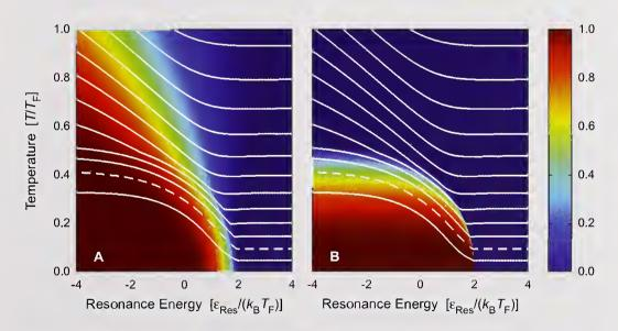
Figure 10. Phase diagrams of atom-molecule mixture showing the molecule fraction (A) and condensate fraction (B) as a function of temperature and resonance energy,  $\varepsilon_{Res}$ , in units of the Fermi temperature and Fermi energy, respectively. Lines indicate contours of constant entropy, which are the trajectories followed by the system under adiabatic variation of the threshold energy.
