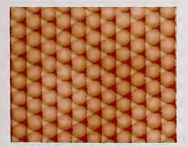
Figure 1. Binding site image for a cobalt atom on a copper (111) surface, showing three-fold symmetry.
