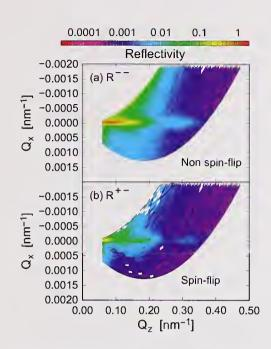
Figure 4. Polarization analysis of neutron reflection from a sample of cobalt "antidots," obtained with a <sup>3</sup>He analyzer and a position-sensitive detector.  $Q_Z$  and  $Q_X$  are the z and x components of the wavevector transfer; spin-flip scattering from magnetic domains is evident in the off-specular data.
