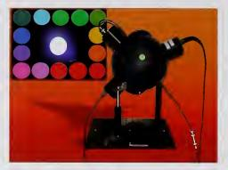
Figure 2. Solid-state integrating sphere source pumped by light emitting diodes, showing some of the different colors that can be generated by varying the input current to the individual LEDs.
