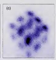
Figure 2. Images showing strontium atoms forming a "cube" as the frequency of the laser light used to manipulate them changes. (a) Atoms become visible at the eight corners of a cube. (b) Atoms also appear at the midpoints of the cube edges and begin appearing at the center of each face. (c) Atoms appear more clearly at the centers of each cube face.
