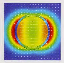
Figure 4. Field within and around a 60 nm radius gold nanoring. Enhanced fields inside the nanoring would make the nanoring a useful container for precision nanoexperiments.
