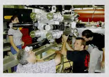
Figure 3. Pieter Mumm (second from right) and colleagues setting up a neutron decay detector for the time reversal asymmetry experiment (emiT).
