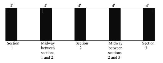
65a.2.1. Conduct at least two complete sets of section tests over each section to at least 90 % of the concentrated load capacity (CLC) of the scale. A single complete shift test is defined in steps a through d. When analyzing the return to zero, consideration must be given for the length of time the load was on the scale and possible temperature changes that may have occurred during the test.
