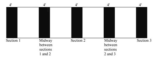
65a.2.1. Conduct at least two complete sets of <u>shift</u> section tests over each section to at least 90 % of the concentrated load capacity (CLC) of the scale. When analyzing the return to zero, consideration must be given for the length of time the load was on the scale and possible temperature changes that may have occurred during the test.
