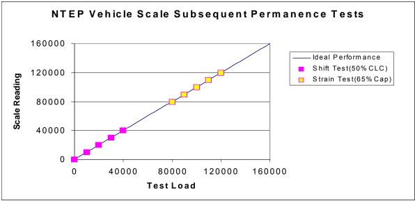
**Note:** For each X in the tables below, the evaluator shall determine actual errors at each test load and application point. Loading shall be within limits specified by the manufacturer as per scale capacity and CLC. All examples are based on the three-section scale pictured in Pub 14. Test points would be added for additional sections as necessary following the same patterns.
