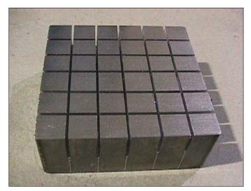
Fig. 2. The effect of microstresses is minimized by utilizing 36  $d_0$  samples in which macrostresses are relaxed by the cross-cutting technique shown.
