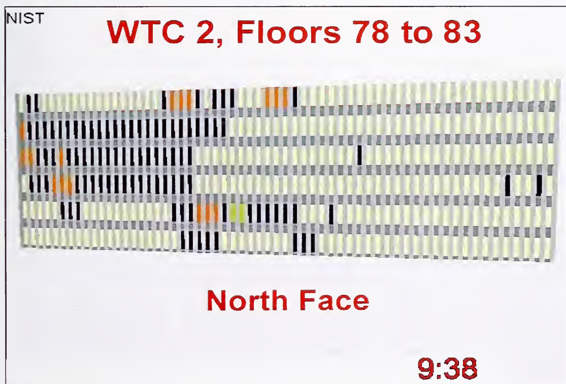
Figure H-11. A single frame from a time-dependent visualization generated by Smokeview is reproduced here. The frame is a three-dimensional representation of the condition of windows and fires on WTC 2 from the time the second tower was struck at 9:02:59 a.m. until it collapsed at 9:58:59 a.m. The color assignments are: – window in place, – missing window, – external flaming, – fire inside, and – spot fire.
