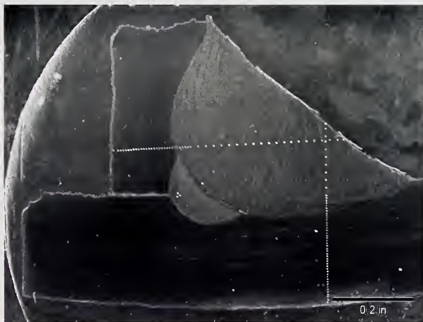
Figure C-22. Micrograph of an exterior column weld geometry.
