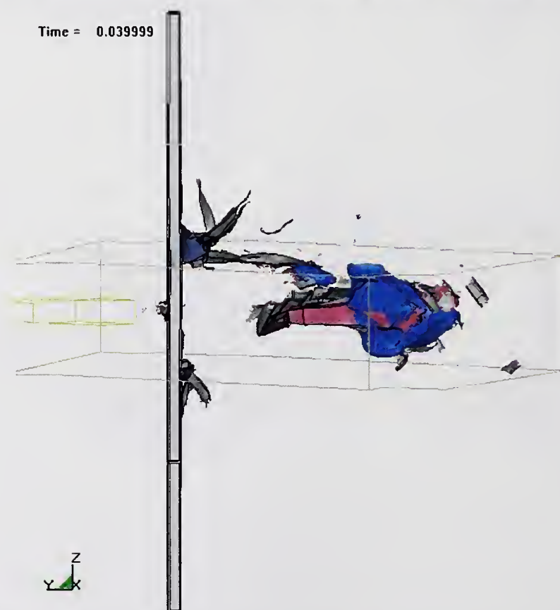
Figure C-67. ALE analysis of structural damage and fuel dispersion (side view).
