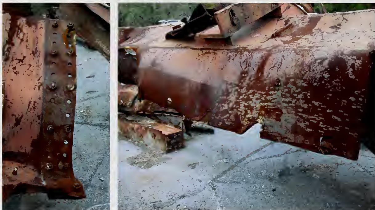
Figure C-69. Typical bolt bearing shear failures of spandrel connections.
