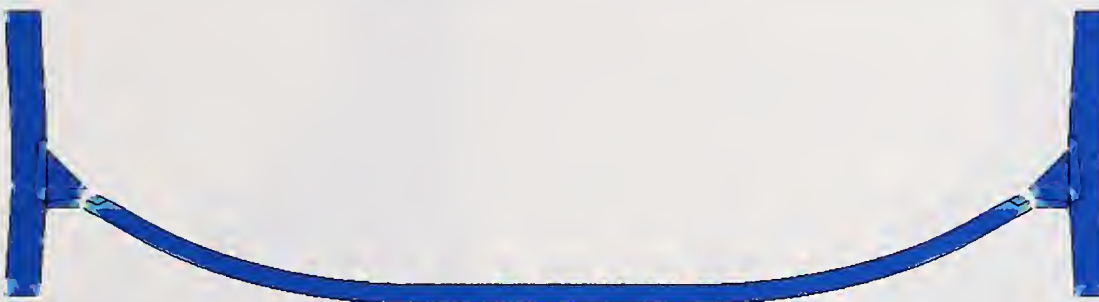
(b) Complete fracture through the web
