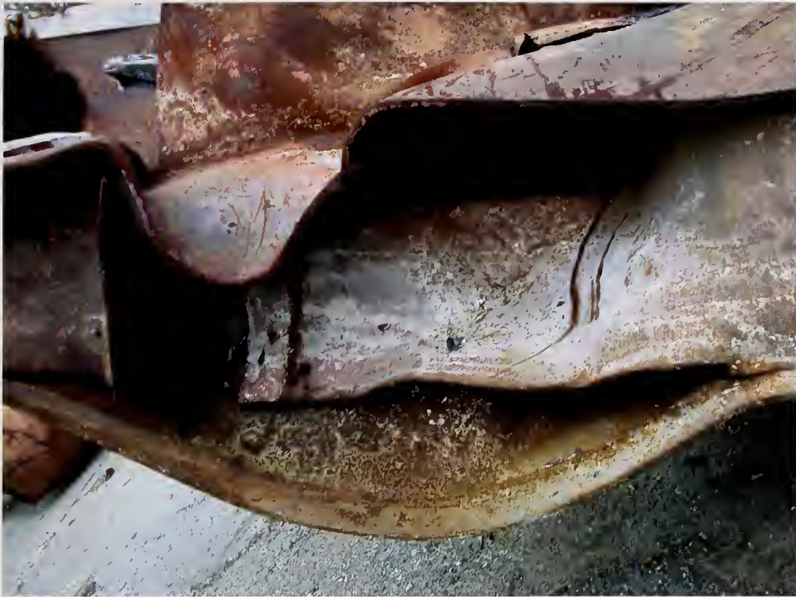
Figure C-21. Photograph of an exterior column with weld zone fractures.
