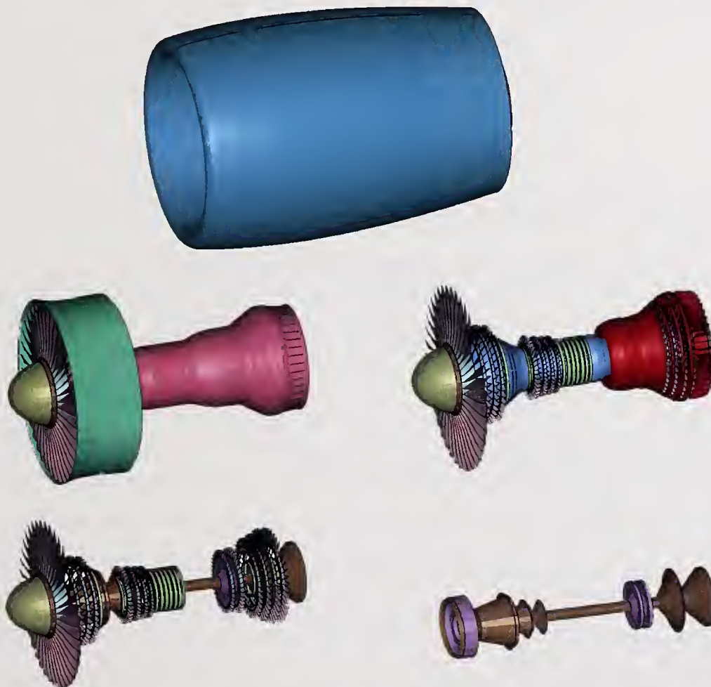
Figure C-45. Pratt and Whitney PW4000 turbofan engine model.
