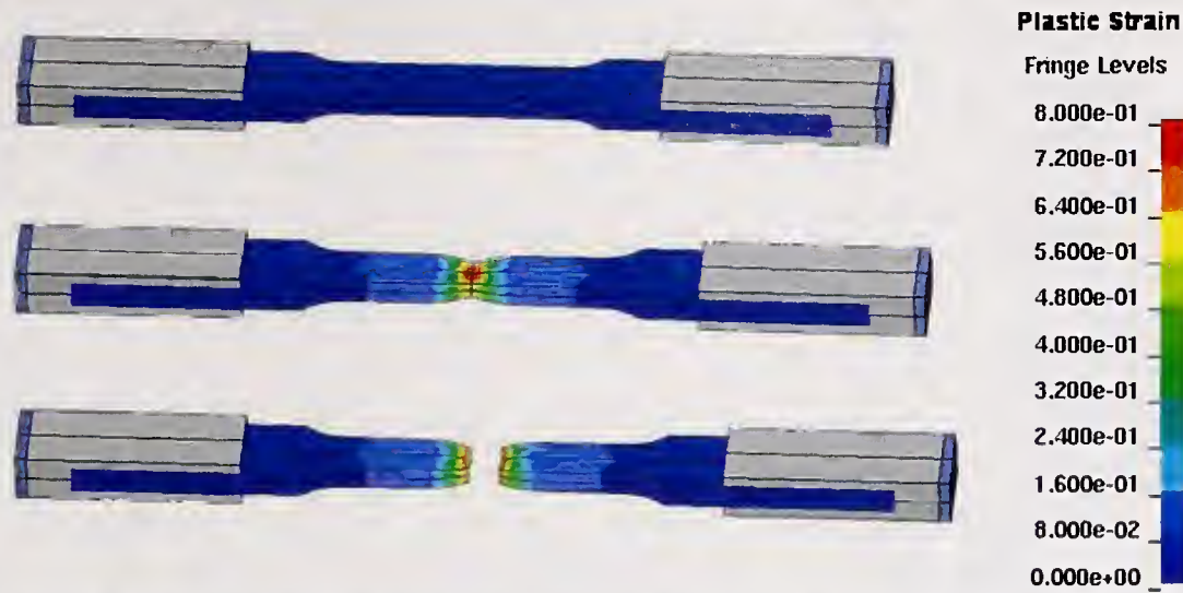
Figure C-5. Calculated tensile test response with necking for the 75 ksi steel.
