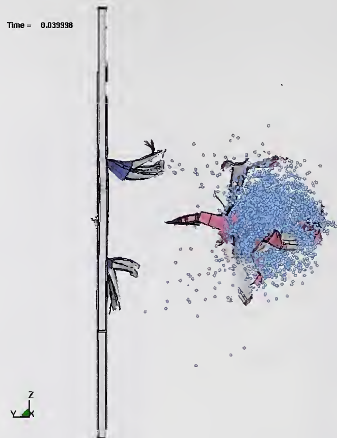
Figure C-66. SPH analysis of structural damage and fuel dispersion (side view).
