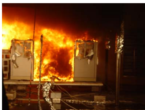
Figure 3. Full involvement of workstation fire near peak heat release rate.
