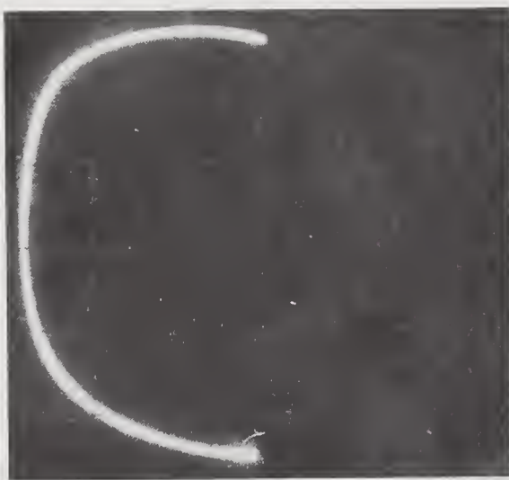
Fig. 3 - Display on s_2, s_3 Stokes parameter plane with a 180^\circ polarization phase modulation
