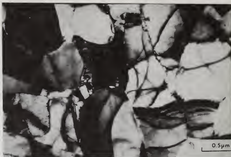
Figure 4. TEM micrograph showing the recrystallized and low defect microstructure of the laser-damaged UBAC for figure 3.
