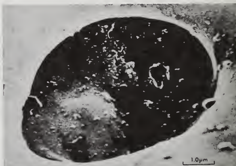
Figure 6. SEM micrograph of the bottom of the pit showing melted material and small particles.
