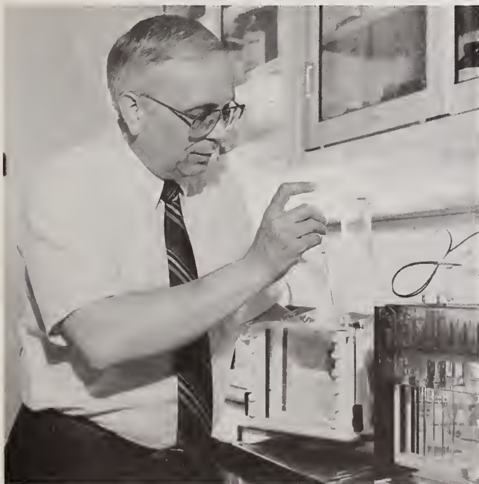
Research chemist Dennis Reeder is working to improve the accuracy of two-dimensional electrophoresis so biotechnology companies can use the technique to assess their products' purity.
