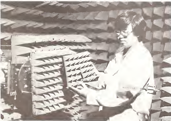
Douglas T. Tamura, an electronics technician, aligns antennas being calibrated on the extrapolation range which is part of the near-field facility.
