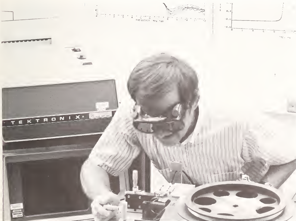
Here electrical engineer Robert Gallawa measures the bandwidth of multimode optical fibers. The measurements are done using three different techniques: frequency domain, time domain, and pulse spectrum analysis.
