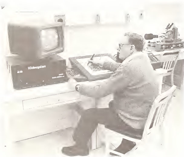
Research chemist Carl Robbins is using a computerized image analysis system to quantitatively analyze an enlarged photograph of ceramic powders.
