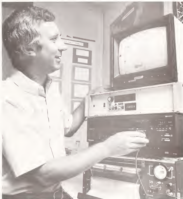
In the NBS fracture laboratory, Dr. Brian Lawn follows crack growth on a computer monitor as a ceramic specimen is tested to failure.
