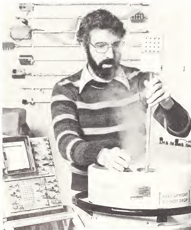
To provide a more precise voltage reference for maintaining the U.S. legal volt, NBS is exploring the use of superconducting microelectronic circuits. Here, electronics engineer Richard Kautz lowers a prototype into a liquid helium dewar for testing.
