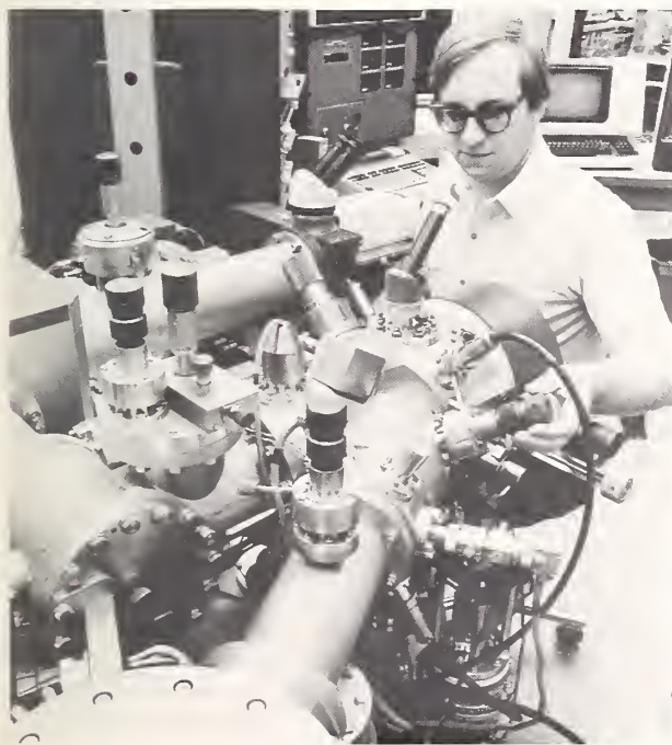
Metallurgist Dale Newbury makes an adjustment on the secondary ion mass spectrometry (SIMS) instrument. This instrument allows researchers to map the distribution of elements both on and below a sample's surface.
