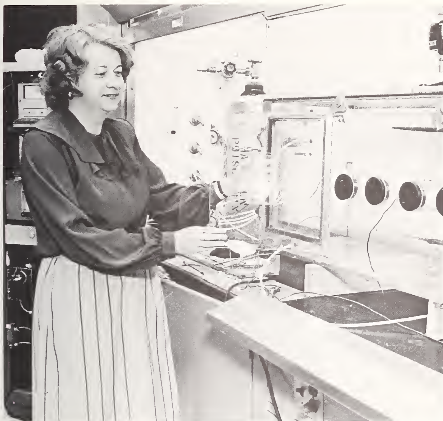
Barbara Levin, research biologist, prepares an experiment aimed at establishing in a measurable way the relative contribution of smoke toxicity to the overall hazards of fire.
