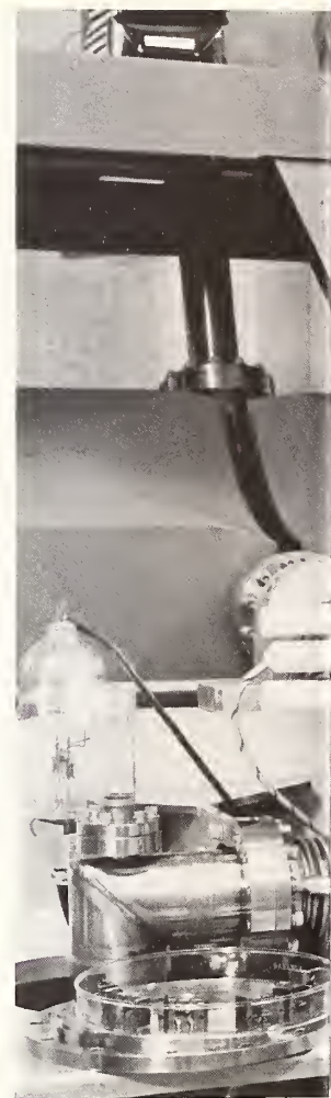
Chemist Gwen Marbury adjusts an electrochemical cell before testing a new polymer-modified electrode for analysis of organohalogen pesticides such as ethylene dibromide (EDB).
