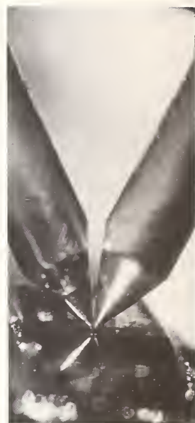
➤ Technician Mike Thomas inspects a silicon specimen through the microscope of a spreading resistance instrument. A photomicrograph (detail) shows a pair of spreading resistance probes poised just above the surface of a silicon test specimen. Reflections of the probes may also be seen in the photo. The separation between the two probes is 25 micrometers, or about 1/3 the width of a human hair.
