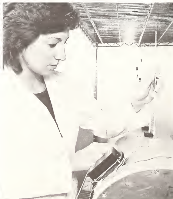
Caroline Harner, a co-op student from the University of Maryland, inserts a sample of a cement component into an isothermal calorimeter to measure the rate at which heat is released during hydration reactions.
