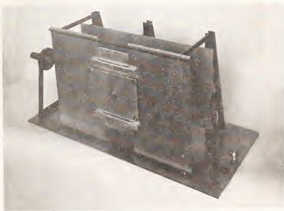
Photo No. 8. Initial standard ionization chamber plate system at NBS (1928).
