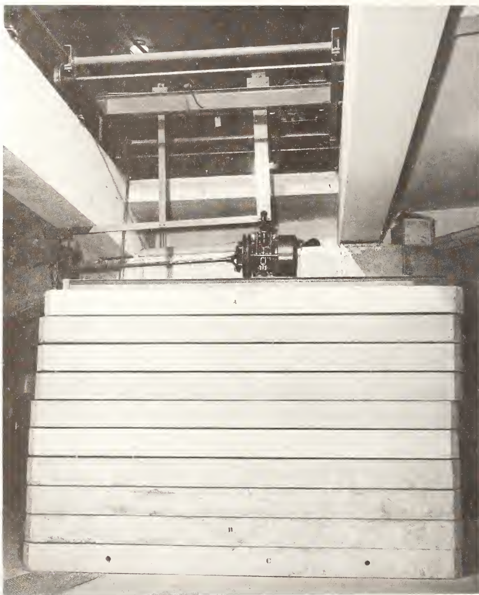
Photo No. 33. Concrete test slabs over measuring pit for broad beam attenuation studies (1950).
