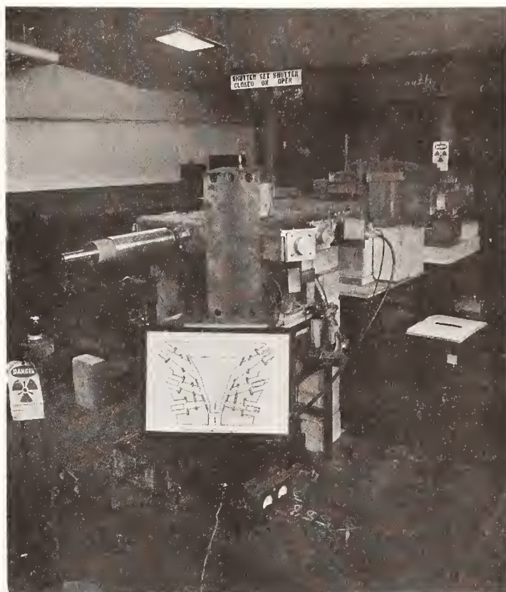
Photo No. 48. Compton magnetic spectrometer for measuring thick-target x-ray spectra (1955).
