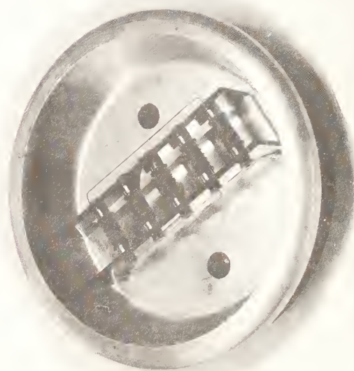
Photo No. 25. 5-kV shielded, wire-wound, high-voltage resistor unit (1930).
