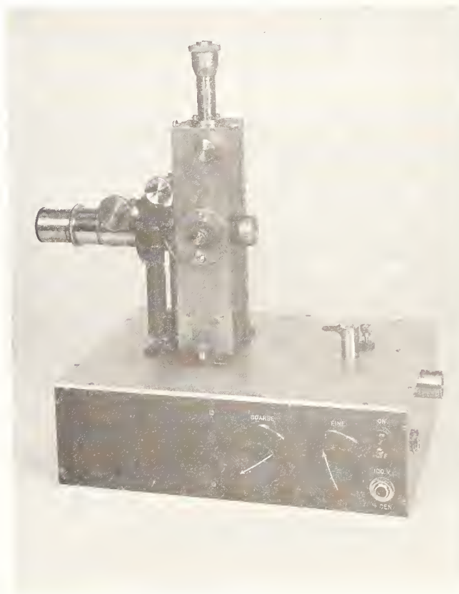
Photo No. 13. Portable, self-contained capacitance compensator for null measurement of ionization currents (1931).
