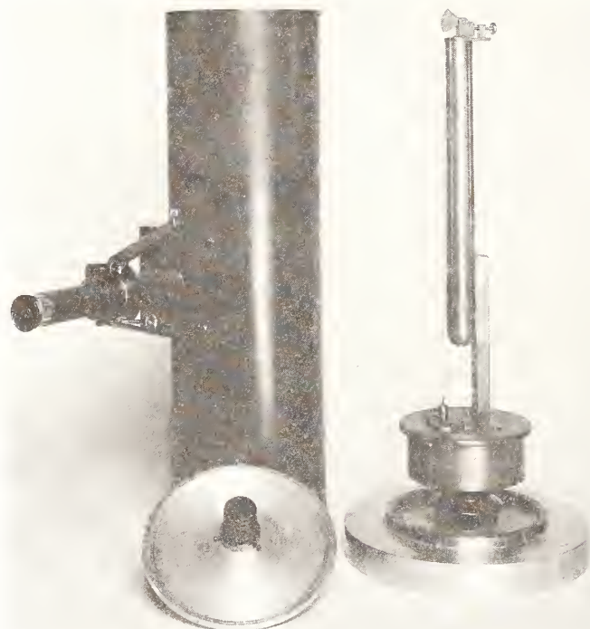
Photo No. 29. 10-kV idiostatic string electrometer-voltmeter (1931).
