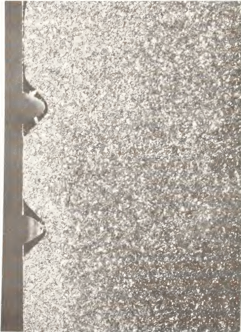
Figure 6. Chromium coated fire ring (worn out)
