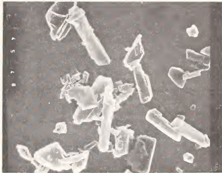
Figure 6. Ground powder form of a grunerite that is classified as a nonfibrous grunerite in the bulk sample form. (Secondary electron image, 3,000X).
