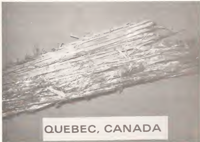
Figure 1. Chrysotile bulk sample (Quebec, Canada).
