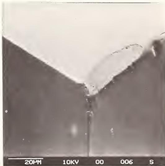
FIGURE 1. Missing volume near a corner of a density standard estimated to be less than  $2 \times 10^{-6} \text{mm}^3$ ,  $\Delta V/V \approx 10^{-10}$ ; photograph taken from a scanning electron microscope.
