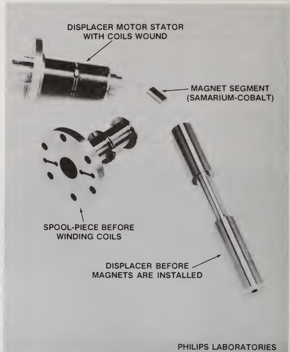
Figure 8. Displacer motor parts.
