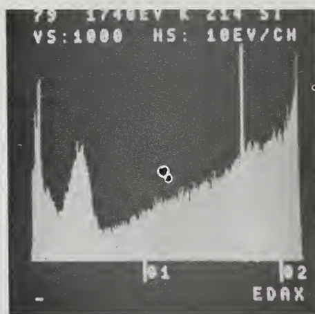
Figure 11. Sulfur "escape peak" and fluoresced silicon peak - window open.
