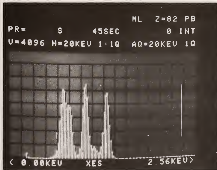
Figure 15. Anomalous peak observed in 0 - 2 keV region in an analytical electron microscope; the peak position varied with the magnification setting (magnification 9500X, 7200X, and 5000X, left to right peaks, frame time 1/s).
