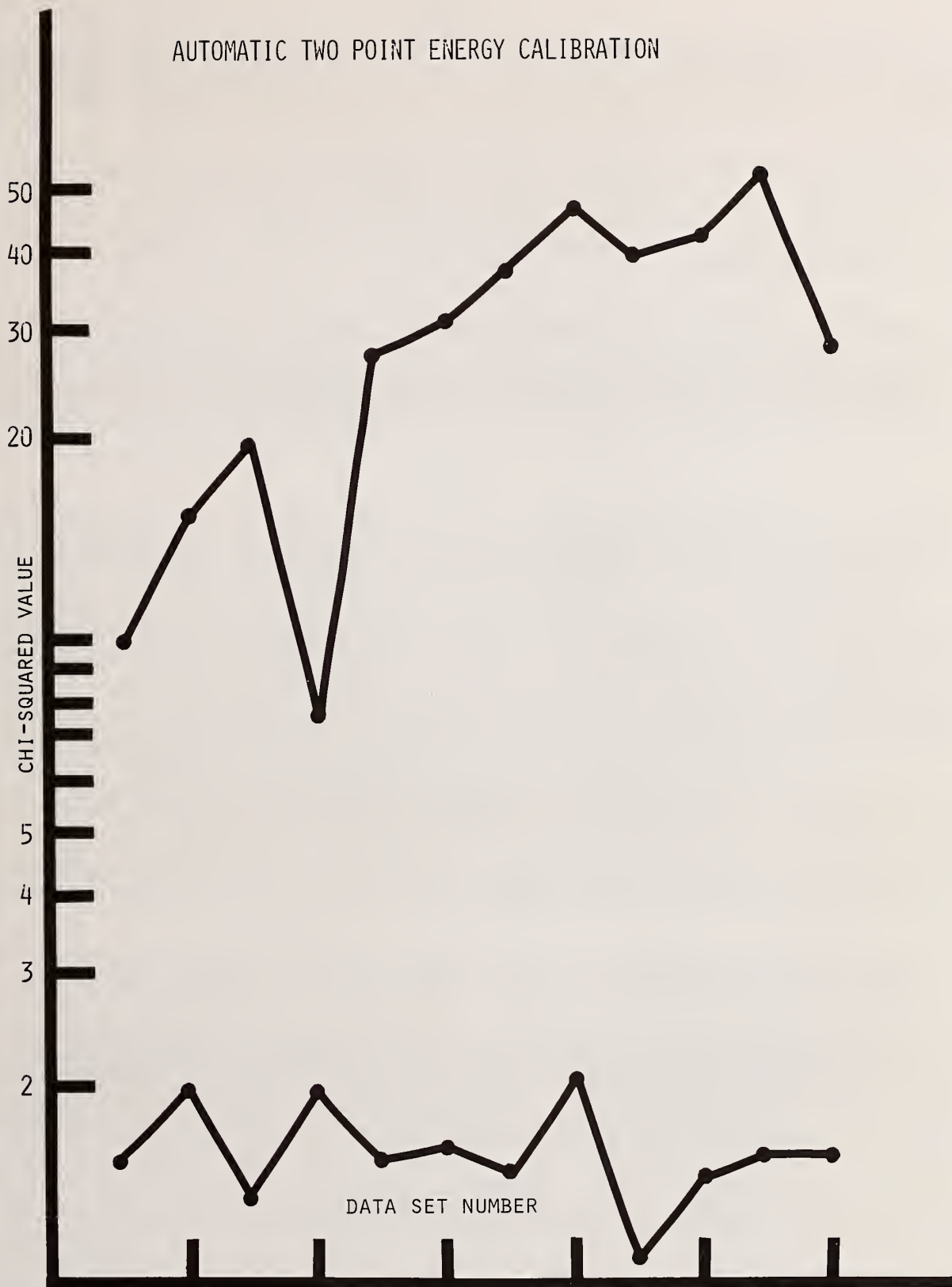
Figure 14. Illustration of the reduction of Chi-Squared by automatic two point energy calibration.
