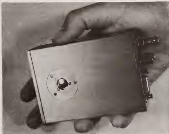
Figure 5. Front end of a prototype portable x-ray mercuric iodide room temperature spectrometer.
