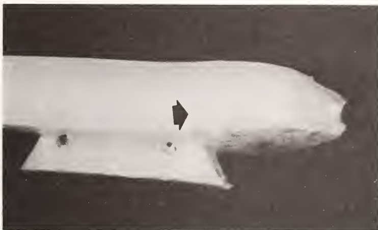
Figure 4. Freeman-Swanson type polyethylene tibial component showing partial fracture (arrow). Time implanted was 60 months.
