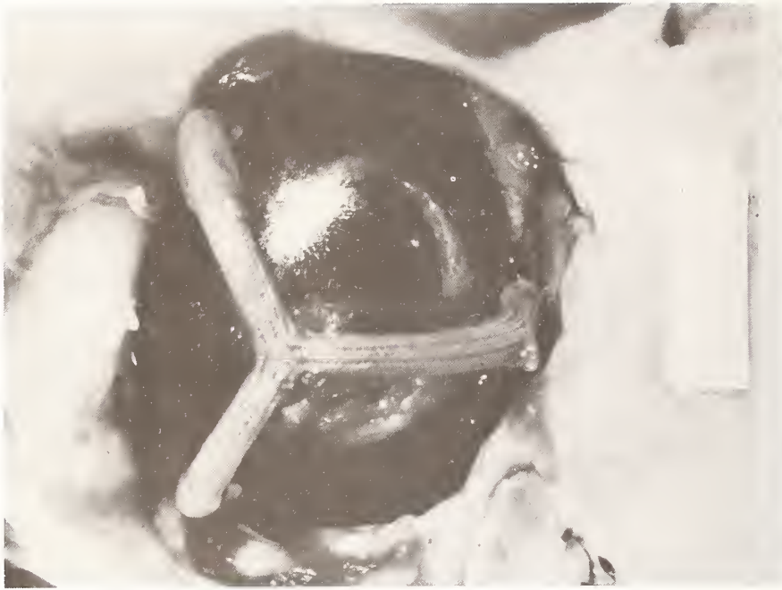
Figure 10. Recovered S-E 2320 aortic valve. Thrombus formation on apex of cage; tissue overgrowth on aortic side of sewing ring and along the base of the struts.
