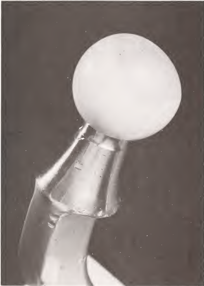
Fig. 8: Removed \text{Al}_2\text{O}_3 -ceramic hip joint prosthesis (implantation period 3 years).
