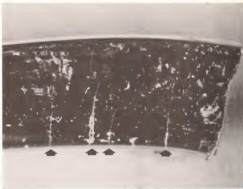
Figure 3. Multiple cracks emanating from the medial side of a fractured small stem T28 prosthesis made from stainless steel. Time implanted was 52 months.
