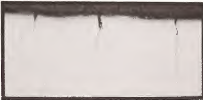
Figure 6. Photomicrograph (250X) illustrating an unetched metallographic cross section adjacent to a bone plate fracture of stainless steel (ASTM F-138) with a group of fatigue corrosion cracks adjacent to the primary fracture.
