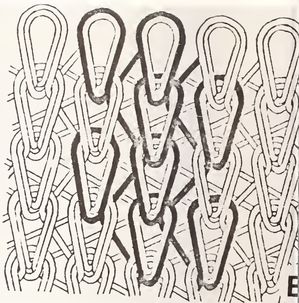
B: Two-bar "locknit" warp knit
