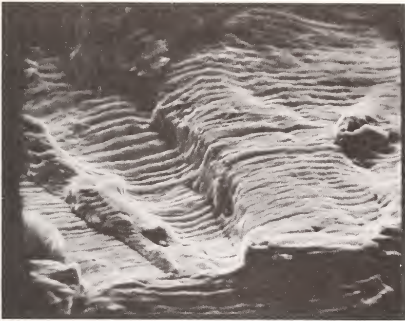
Figure 2. Scanning electron microscope photomicrograph (2100X) illustrating mechanical fatigue failure of a stainless steel (ASTM F-55) bone plate.
