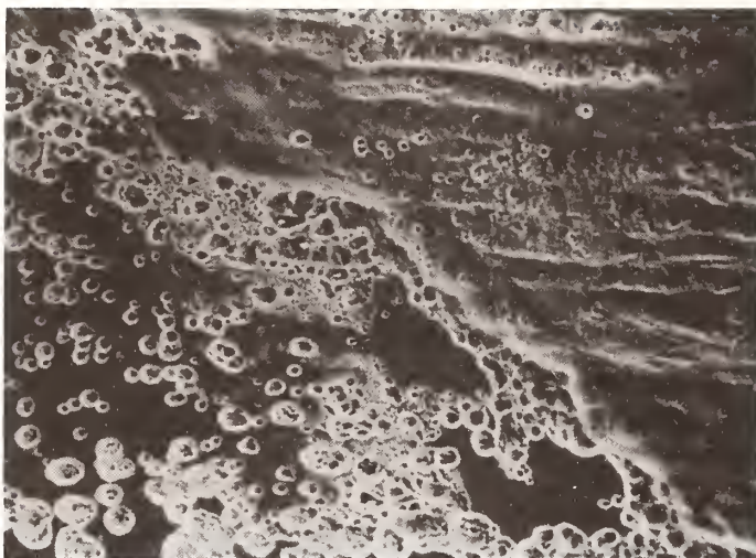
Figure 4 SEM photograph of contact area on plate position d2 from patient #10 in plate study. Contact area is in upper right, with edge running diagonally. Pitting is outside of primary contact area.
