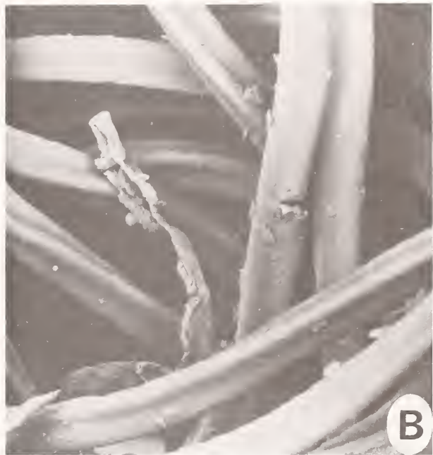
Figure 8.14 : (MO18) A. External view of Microvel prosthesis after 17 months in-vivo. B. Velour trilobal cross-section filament with isolated transverse cracks.
