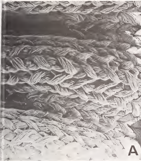
Figure 8.04 : (B55) A. External view of Knitted Cooley prosthesis explanted after 48 months. B. Internal lumen side view of filaments at the crest of a crimp showing flattened surfaces probably caused by contact of the mandrel during crimping.
