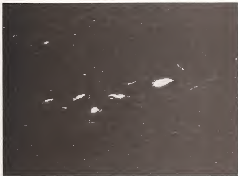
Figure 7. Microphotograph of tissue section, stained H&E, of capsular tissue surrounding a Müller total hip prosthesis after four years of function, material combination: CoCrMo-cast alloy on UHMW Polyethylene, 400 magnification, a) bright light, b) polarized light. Particles are visible by means of their birefringence.
