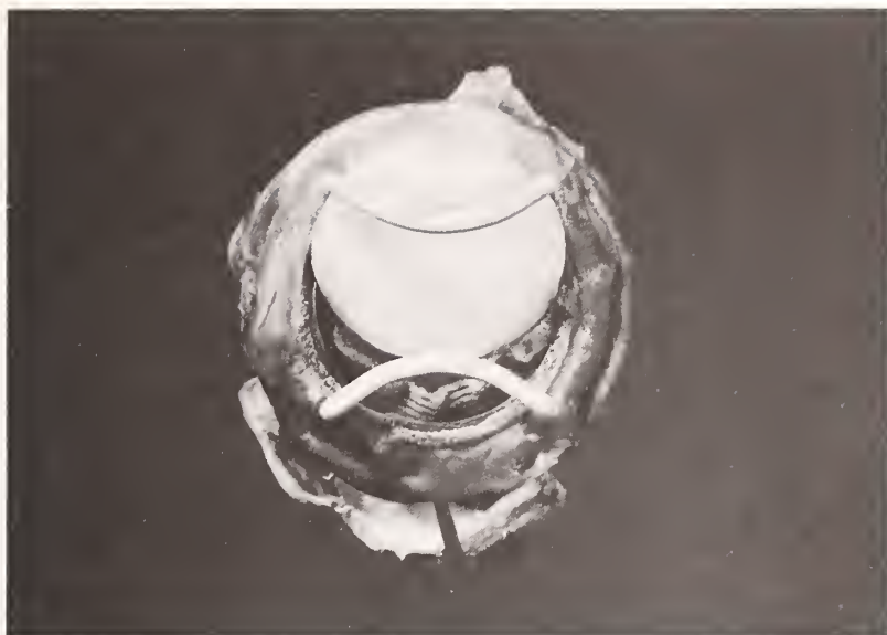
Figure 1. Ventricular view of a Beall model 104 mitral valve with marked sewing ring fabric wear. Implanted for 6.5 years, note exposed metallic frame.
