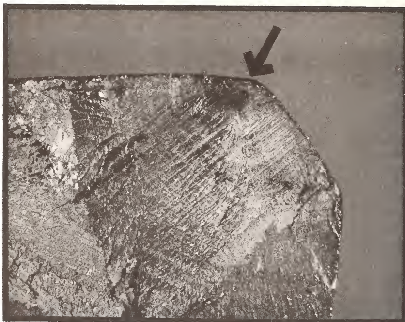
Figure 1. Photomicrograph (15X) of fatigue origin on the femoral stem portion of total hip prosthesis (ASTM F-75). The macro-fatigue striation emanates from the portion indicated by the arrow.
