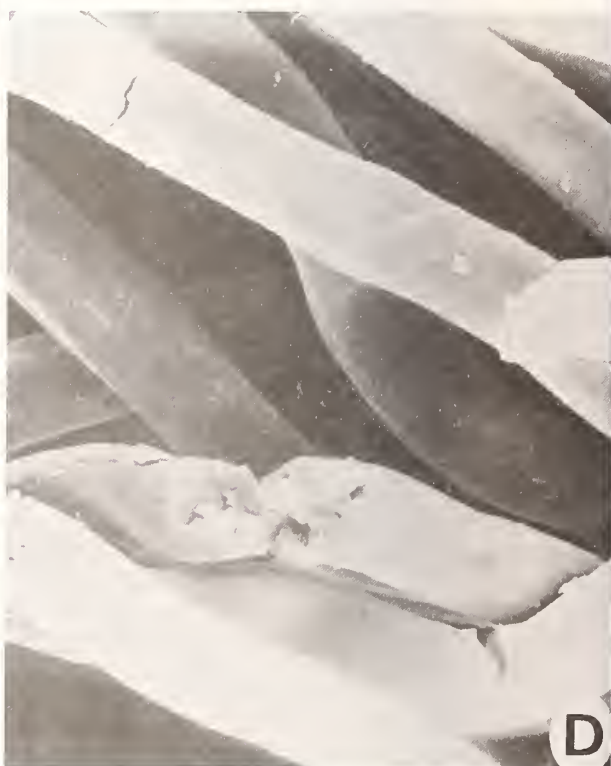
Figure 3.11 : (FP26) A. View of damaged Weavenit prosthesis after 84 months B. Yarn failure. C. Non-circular filaments deformed pressure from adjacent yarns during prosthesis manufacture. D. Transverse cracks and fracture surfaces of embrittled filaments.
