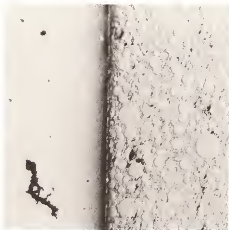
Figure 13, Cement-Prosthesis Interface: Sample A - "normal" interface x 75
