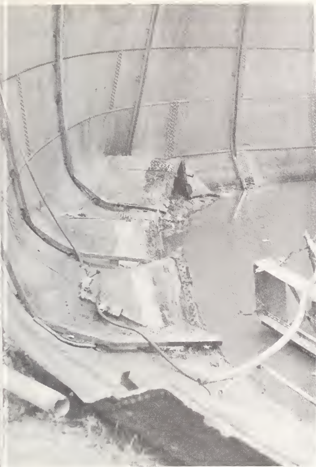
Figure 6.36 Haranomachi Plant, Sendai City Gas Bureau: a fracture of the 3/8-in. plate wall of the collapsed gas holder. The length of the fracture is approximately 1.5 m (5 ft).
