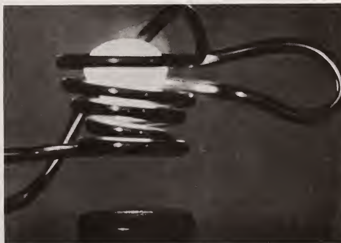
Fig. 2 Induction coil with a white-hot molten drop
