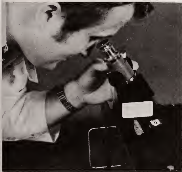
Figure 2. Inspecting the integrity of a fiber-optic seal.
