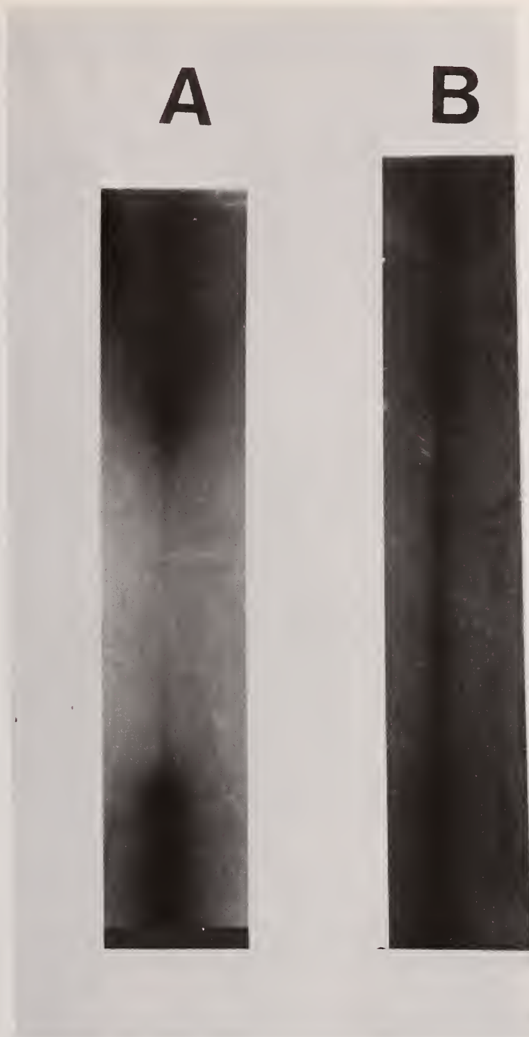
Fig. 3. At-critical Active Autoradiographs of 93%-enriched Uranium Fuel Columns With Defects A: Missing Plate B: 20% Enriched Plate
