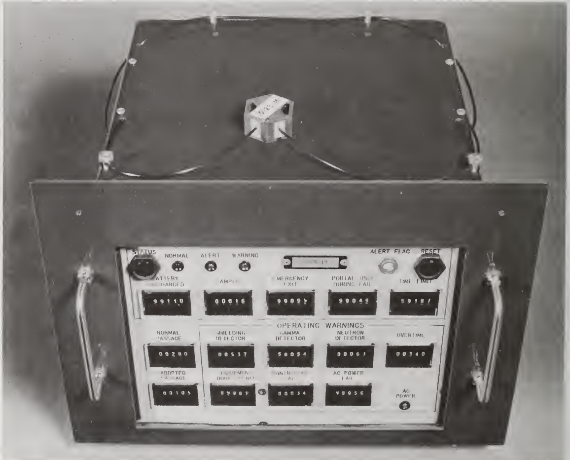
Figure 1. The Secure Counter Panel records tamper events and other operating data.
