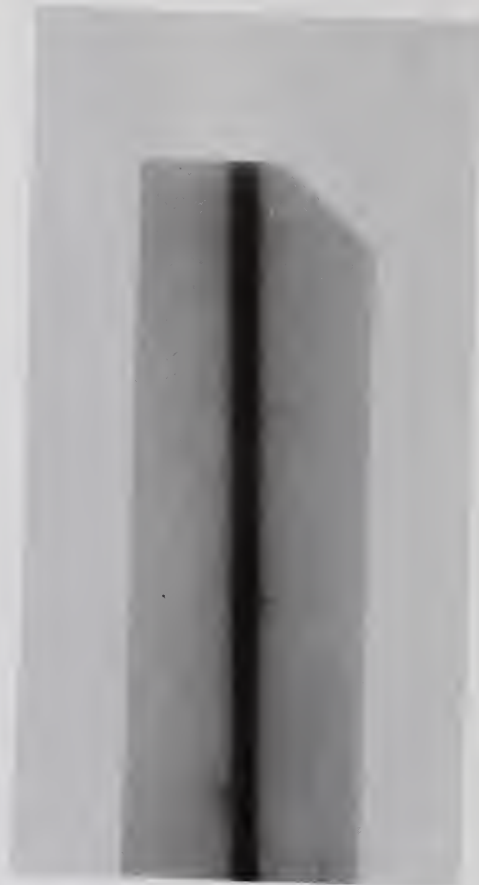
Fig. 2. At-critical Active Autoradiograph of a Highly-enriched-uranium Fuel Column
