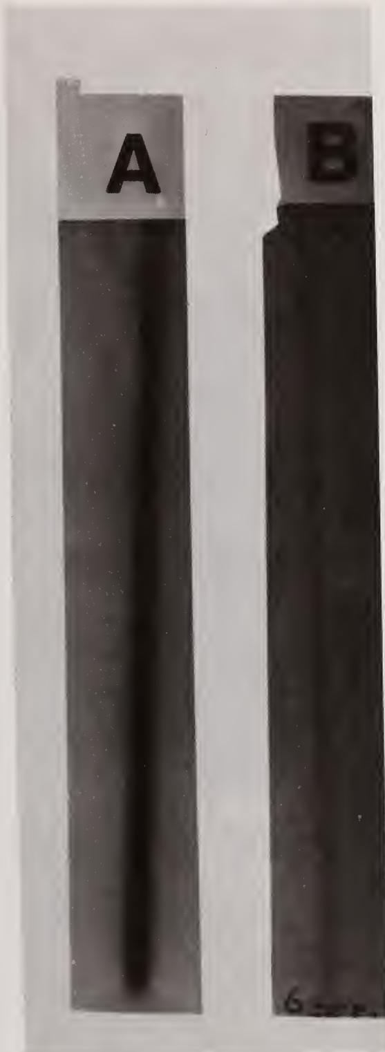
Fig. 1. A: Post-irradiation Active Autoradiograph of a Highly-enriched-uranium fuel column B: Passive Autoradiograph of Highly-enriched-uranium Fuel Column
