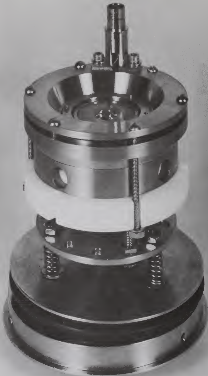
Lower Grid, Surface Barrier Detector and Sample Plate - Assembled View
