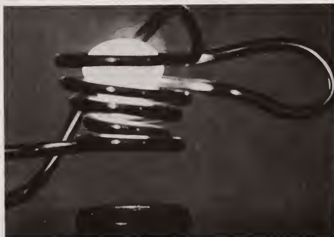
Fig. 2 Induction coil with a white-hot molten drop
