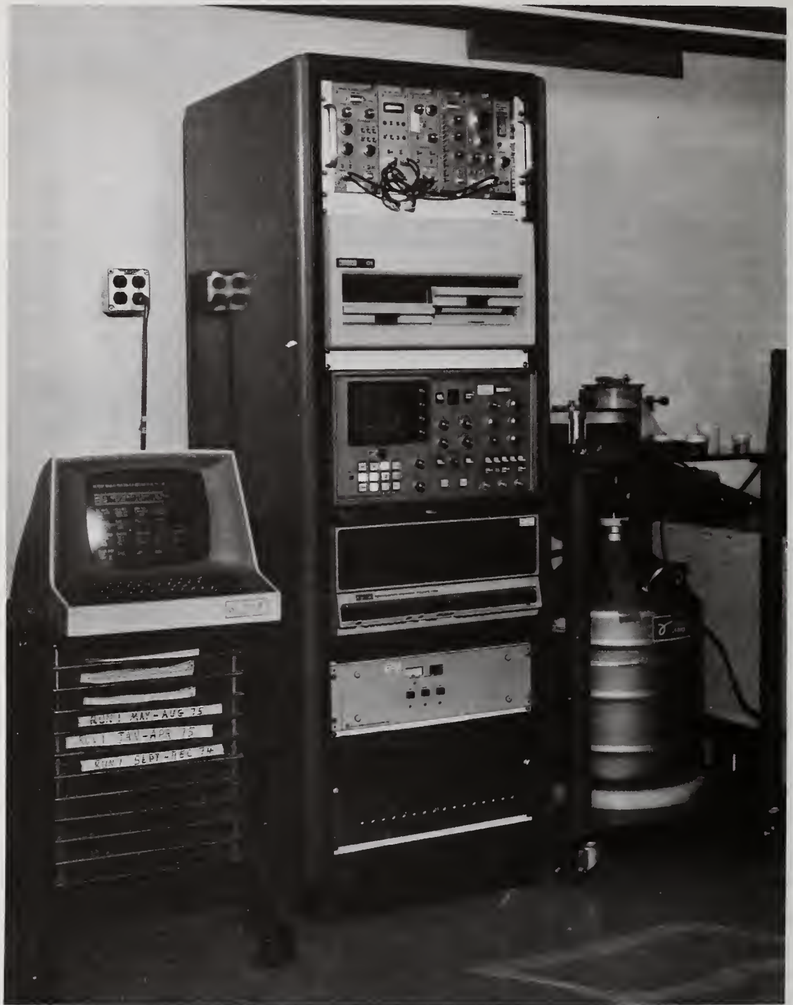
1. The Uranium Solution Assay System
