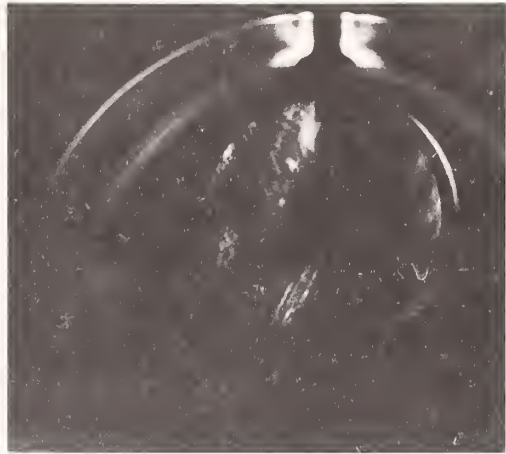
Figure 5. Stress birefringence in single-crystal \text{CaF}_2 .
