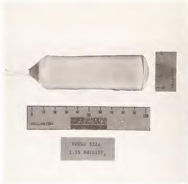
Figure 3. Single crystal Nd:YLF laser material.
