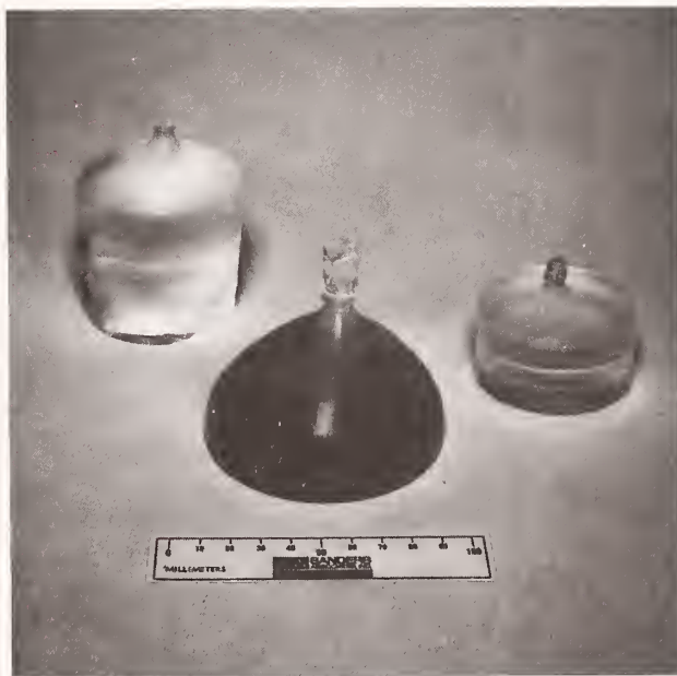
Figure 6. Single crystals of rare earth doped YLF from growth scaling experiments.
