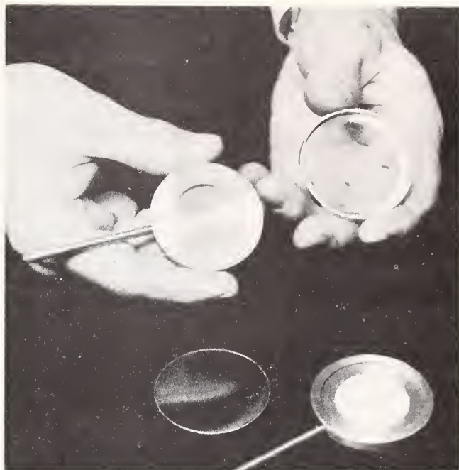
Figure 4 Powder in Holder for Determination of Color Designation.
