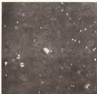
Figure 14. Low magnification scanning electron micrograph of a suspended particulate air sample. (800X)
