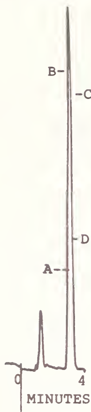
Figure 25. Absorbance ratio measurements to determine an impurity eluting with a niacinamide standard [105]. Column: 50 cm \times 2.6 mm packed with ODS-SIL-X-I. Mobile phase: water, 1 mL/min. Column temperature: 40 °C. Detection was done at 240 nm except where absorbance at other wavelengths was measured. See Table 7 for the measured values.
