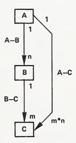
Figure 5-7. An Example of Redundant Relationships
