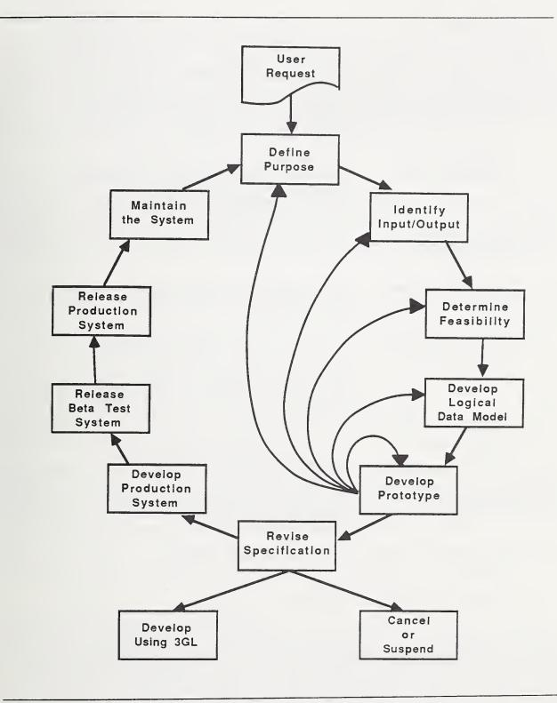
Figure 2. Software Life Cycle with Integrated Prototyping
