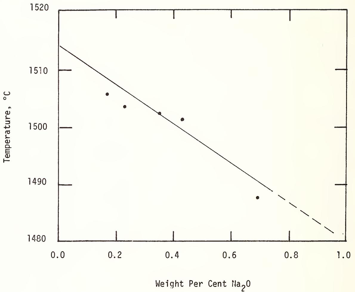
Fig. 6 The effect of Na<sub>2</sub>O on the liquidus temperature of an oxide melt having a % CaO + % MgO/% SiO<sub>2</sub> + % Al<sub>2</sub>O<sub>3</sub> ratio of 1.12.
