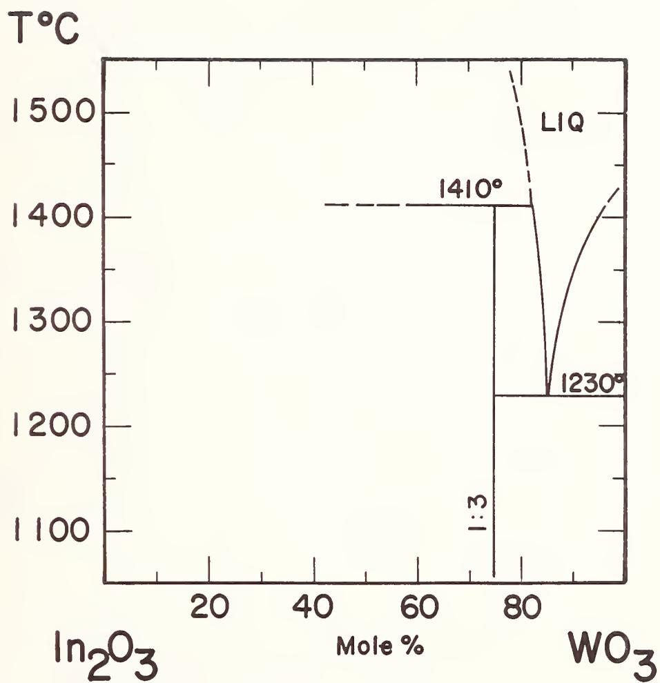
FIGURE 27. Phase relations in the system  $\text{In}_2\text{O}_3$ - $\text{WO}_3$
