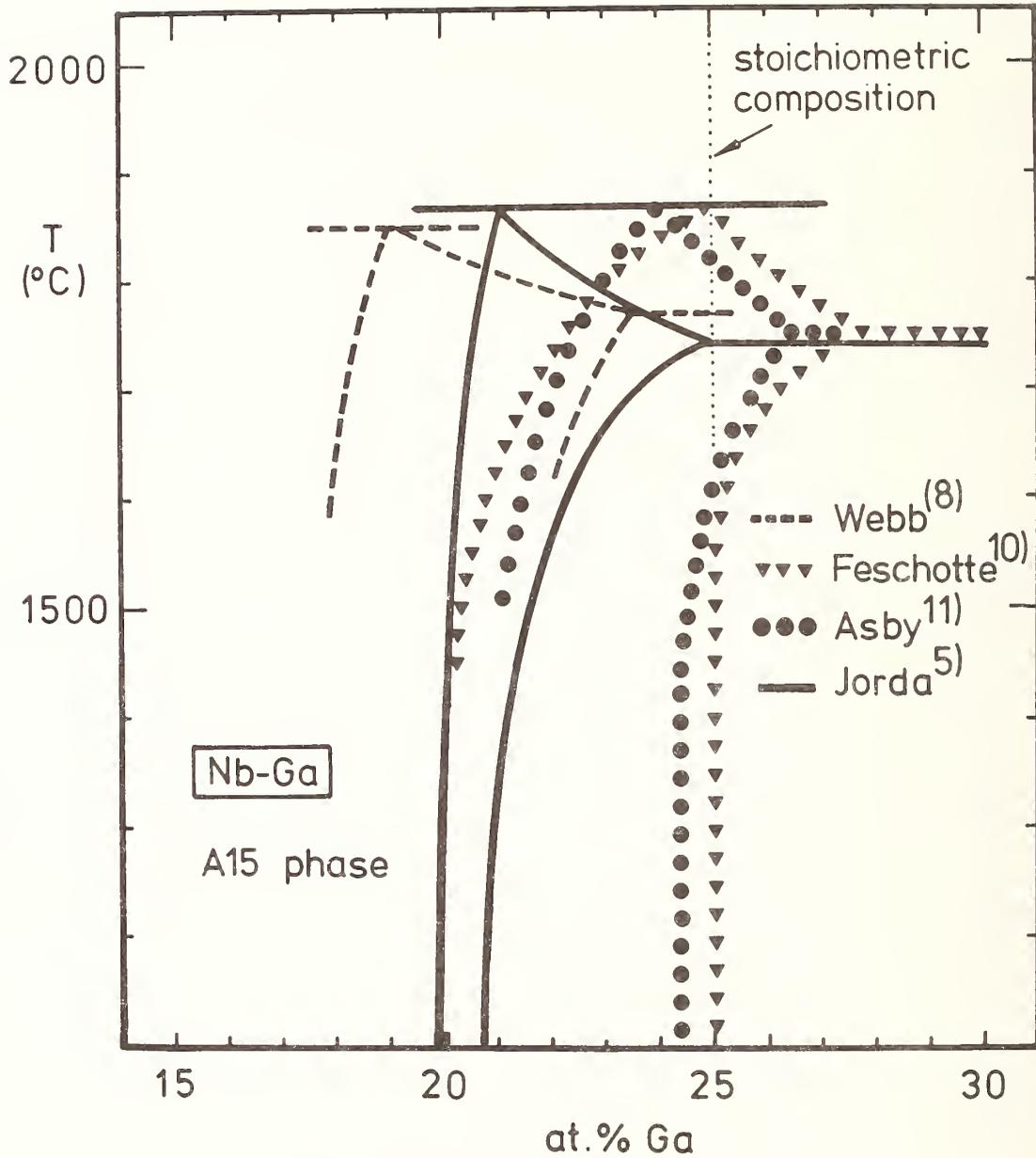
FIGURE 7. The A15 phase field in the Nb-Ga system as reported by different authors. The strong dependence of the Ga-rich limit on the temperature observed by Jorda et al. {5} was obtained using argon jet quenching at different temperatures between 1100 and 1740°C.
