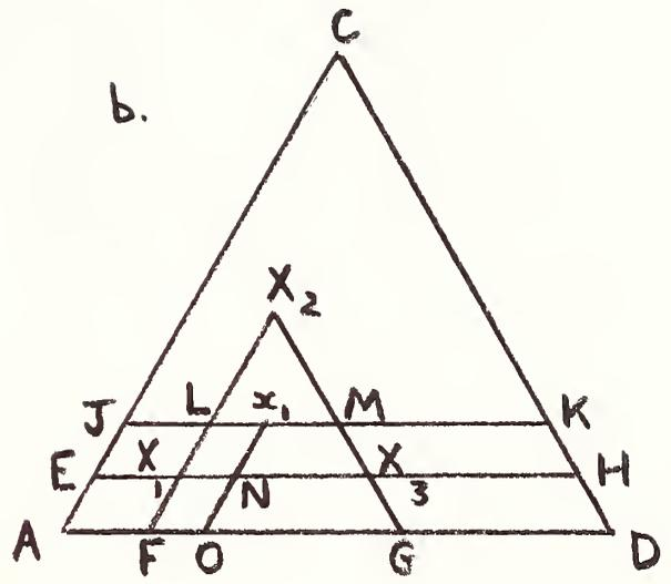
FIGURE 8. Orthogonal Parallel Projection of Quaternary Alloy X
