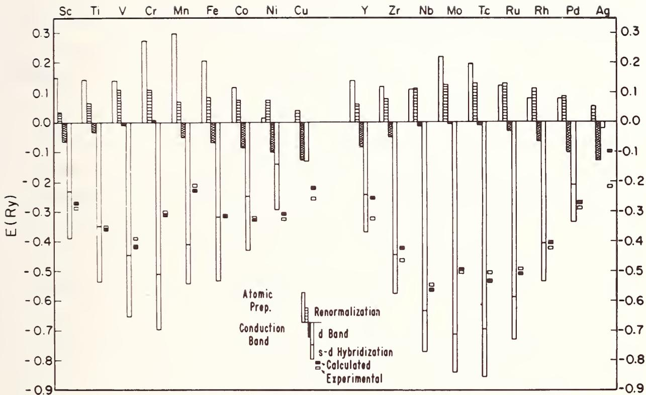
Fig. 3. Theoretical estimates of the various contributions to the cohesion of the 3d and 4d row transition metals. The breakdown of the contributions follows from Fig. 2: These are the preparation of the atom into the proper atomic configuration, renormalization to the metallic volume, conductor and d-band broadenings, and the effects of s-d hybridization. See Ref. 2 for details of the calculation.
