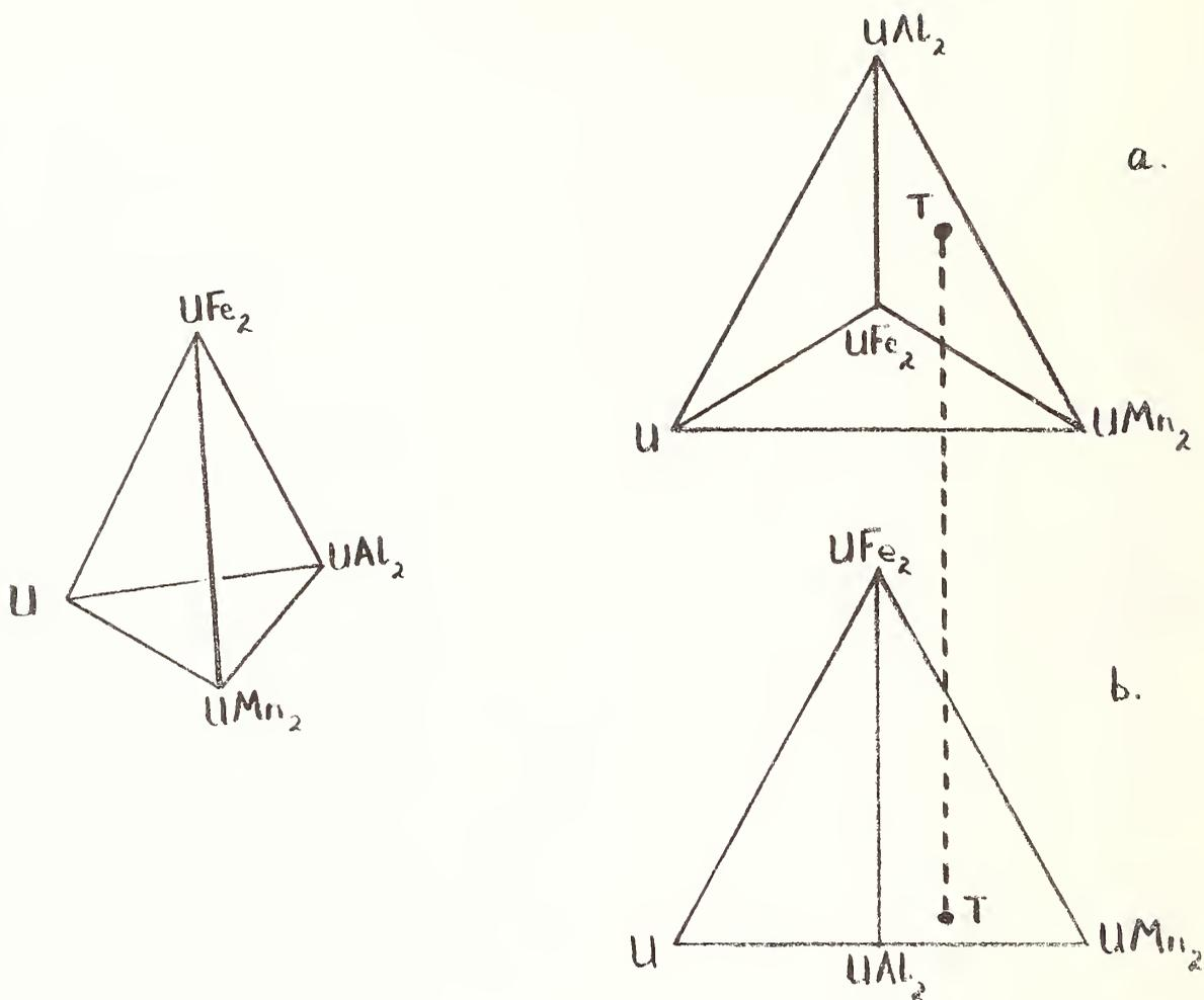
FIGURE 9. Projection of the U-UMn<sub>2</sub>-UAl<sub>2</sub>-UF<sub>e</sub><sub>2</sub> System
