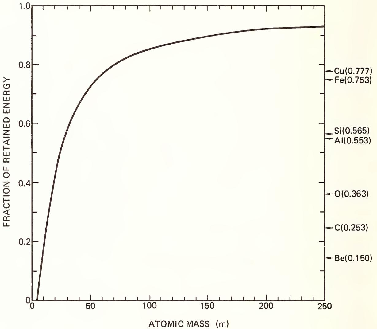
Figure 2. Relation between energy of backscattered ions and atomic mass of scattering species for backscattered angle of  $170^\circ$ . Values for several elements are listed at right.
