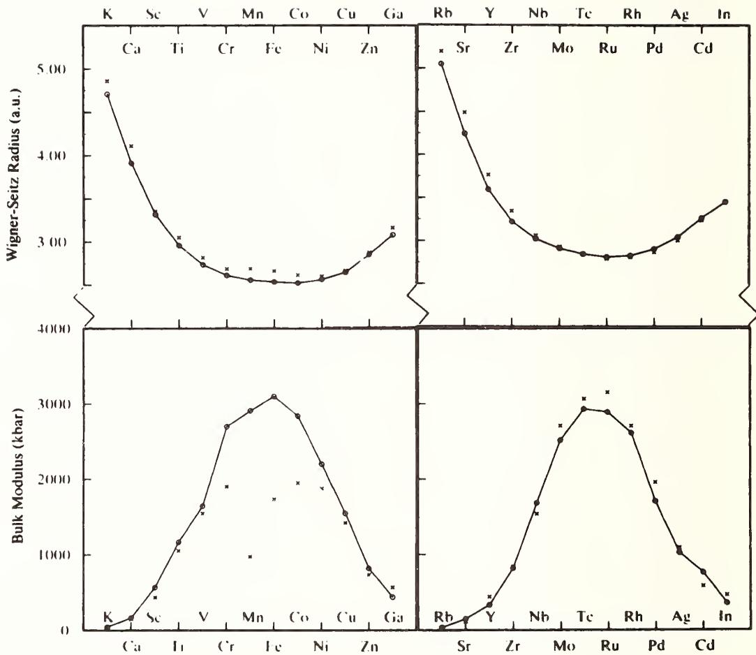
Fig. 4. Janak and Williams' band theory estimates<sup>(10)</sup> of the Wigner-Seitz radii and bulk moduli of 3d and 4d transition metals in the paramagnetic states. The crosses are experimental values. Note that there are significant deviations for Cr through Ni, which have magnetic moments.
