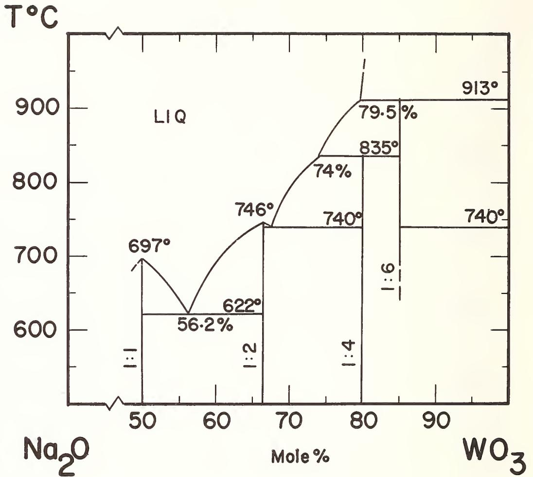
FIGURE 2. Phase relations in the system  $\text{Na}_2\text{O}\cdot\text{WO}_3-\text{WO}_3$
