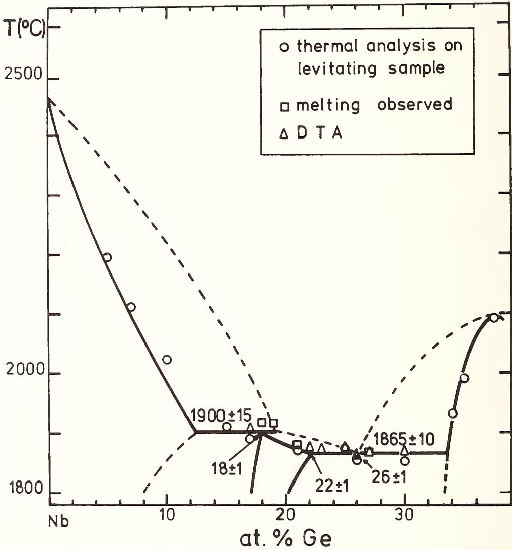
FIGURE 11. The high temperature part of the Nb-Ge phase diagram as obtained by thermal analysis on levitating samples, combined with DTA and "simultaneous stepwise heating".
