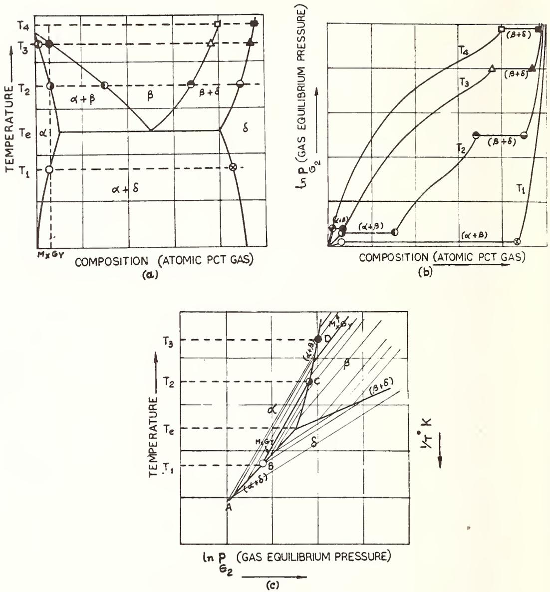
Figure 1. Phase-Diagram of Metal-Gas System (Schematic) (a) Temperature-composition Diagram (b) Pressure-Composition Isotherms (c) Pressure-Temperature Isochores
