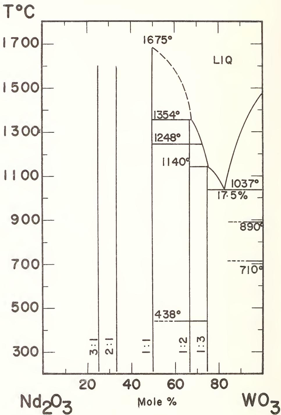
FIGURE 14. Phase relations in the system  $\text{Nd}_2\text{O}_3$ - $\text{WO}_3$
