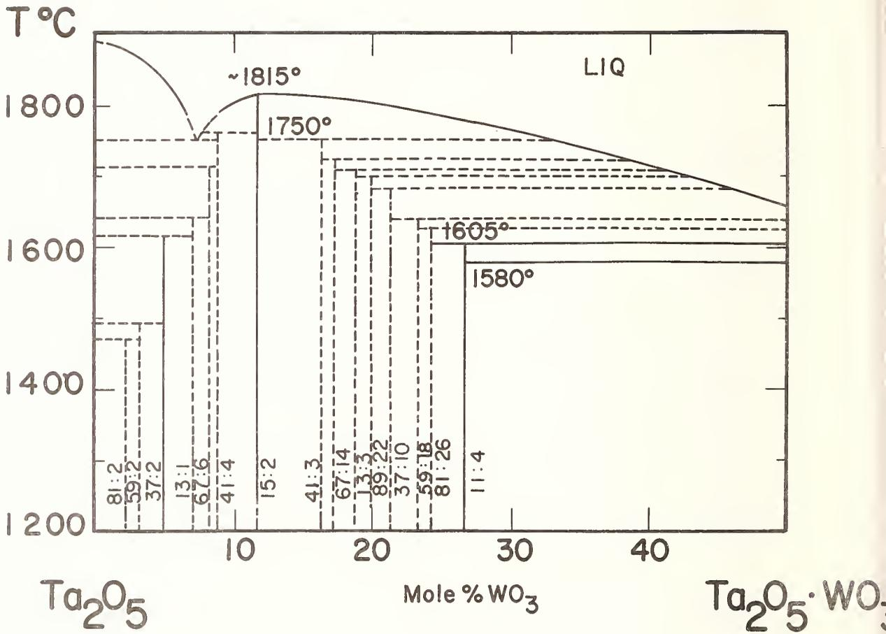
FIGURE 20. Phase relations in the system  $\text{Ta}_2\text{O}_5$ - $\text{WO}_3$
