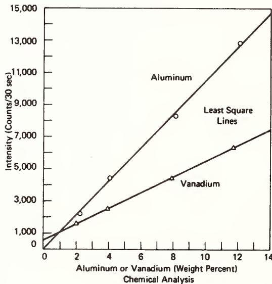
FIGURE 1. Mean Number of Counts (per 30 sec.) Versus Chemical Analysis of Aluminum and Vanadium Standards
