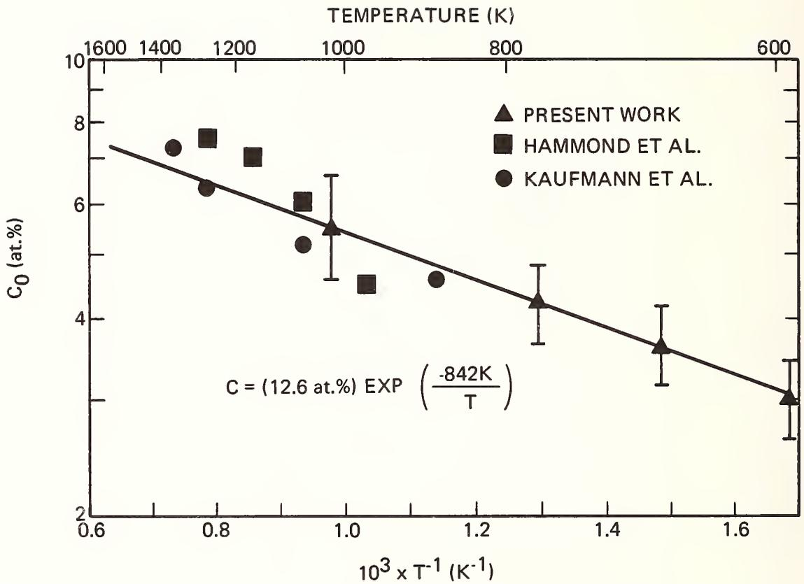
Figure 8. Solubility of copper in beryllium as a function of temperature on a log solubility versus  $T^{-1}$  plot. Plot shows data, while analytical expansion represents best fit.
