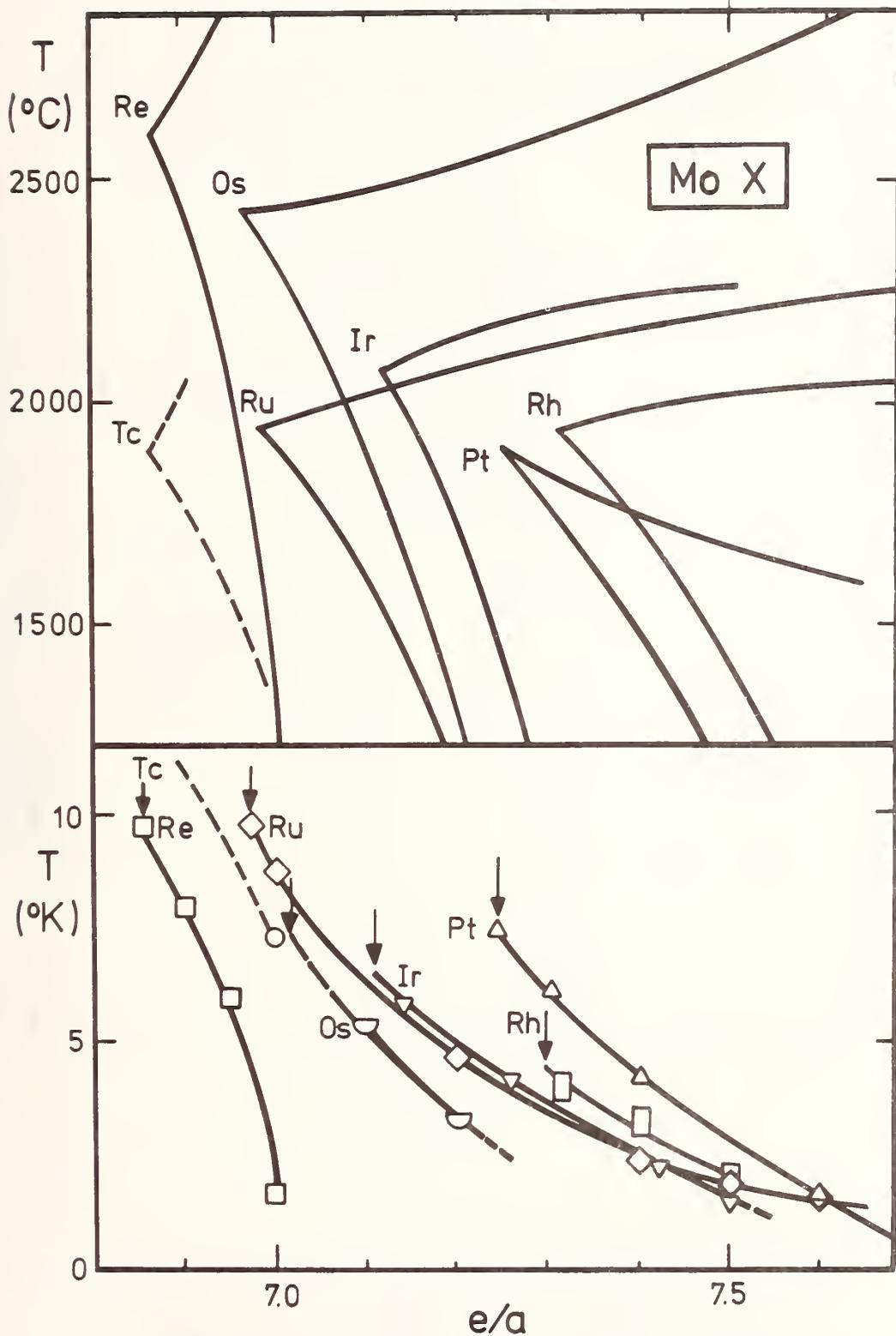
FIGURE 6. The dependence of  $T_c$  on the number of electrons per atom for several hexagonal Mo-X compounds. The arrows denote the highest value of  $T_c$  in a given system, corresponding to the extreme solubility limit of the hexagonal phase at high temperature, as it follows from the upper picture.
