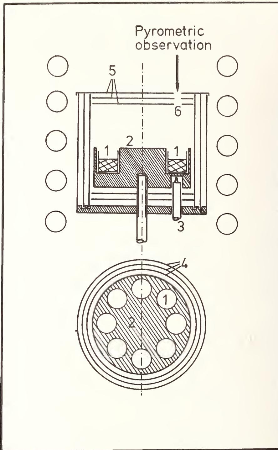
FIGURE 3. The high temperature cell for the "simultaneous stepwise heating", mounted in a HF coil. The sample temperature is measured both by thermocouples and a two-color pyrometer, allowing a "calibration" of the latter for measurements at higher temperatures. 1 : samples, 2 : Molybdenum block, 3 : Thermocouple, 4,5 : Molybdenum shields, 6 : hole for pyrometric observation.
