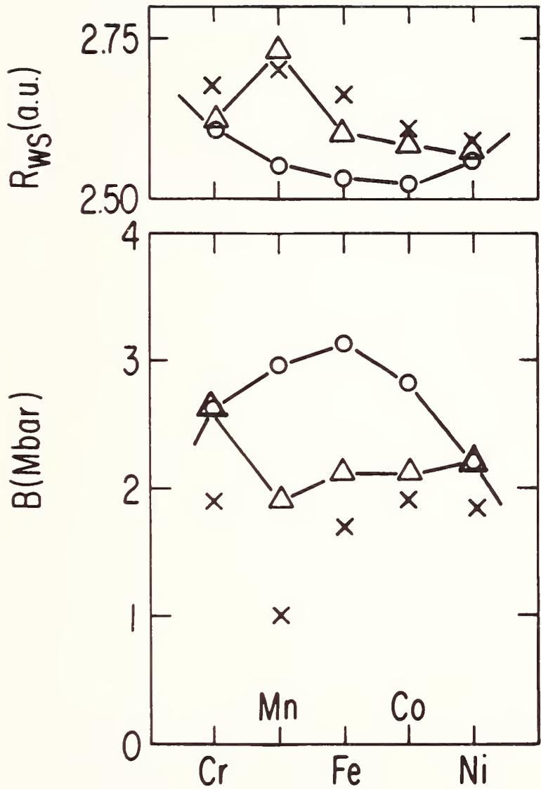
Fig. 5. Janak and Williams' estimates<sup>(10)</sup> of Wigner-Seitz radii and bulk moduli for the paramagnetic (circles) and magnetized (triangles) transition metals Cr through Ni. The crosses are the experimental values.
