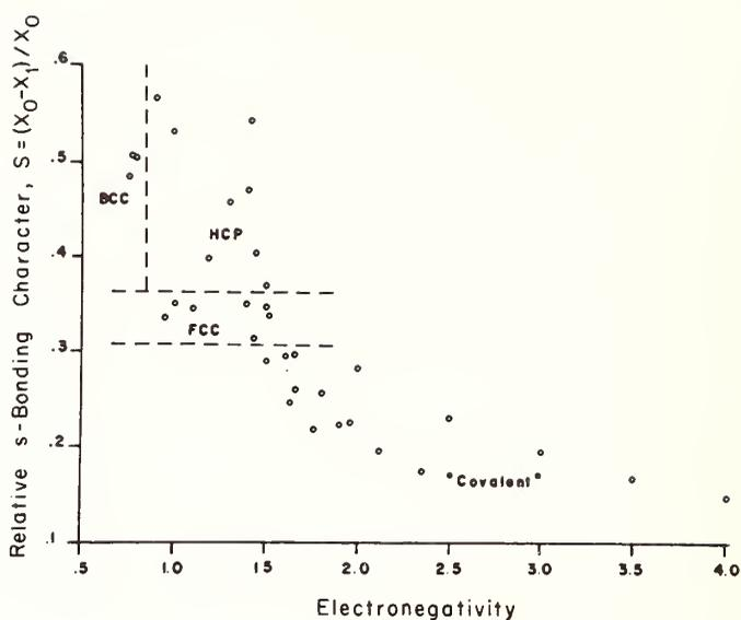
Fig. 10. Correlation of the structures of the non-transition metal elements with electronegativity and fraction of s characters in the bonding as obtained by St. John and Bloch<sup>28</sup>.
