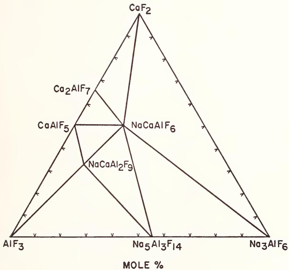
Figure 16. Subsolidus Compatibility Relationships in the System  $\text{CaF}_2\text{-AlF}_3\text{-Na}_3\text{AlF}_6$  <sup>(56)</sup>.
