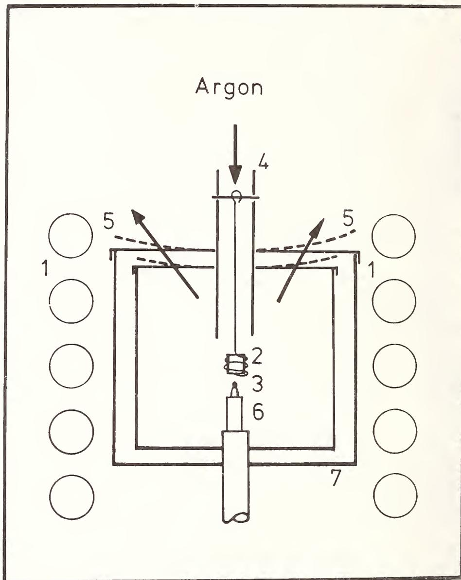
FIGURE 5. The argon jet quenching device. 1 : HF coil, 2 : sample, hanging on a tantalum wire, 3 : Thermocouple, 4 : Tantalum tube, 5 : Molybdenum lid, is blown away by the argon jet, 6 : 2 hole BeO tube for the thermocouple wires.
