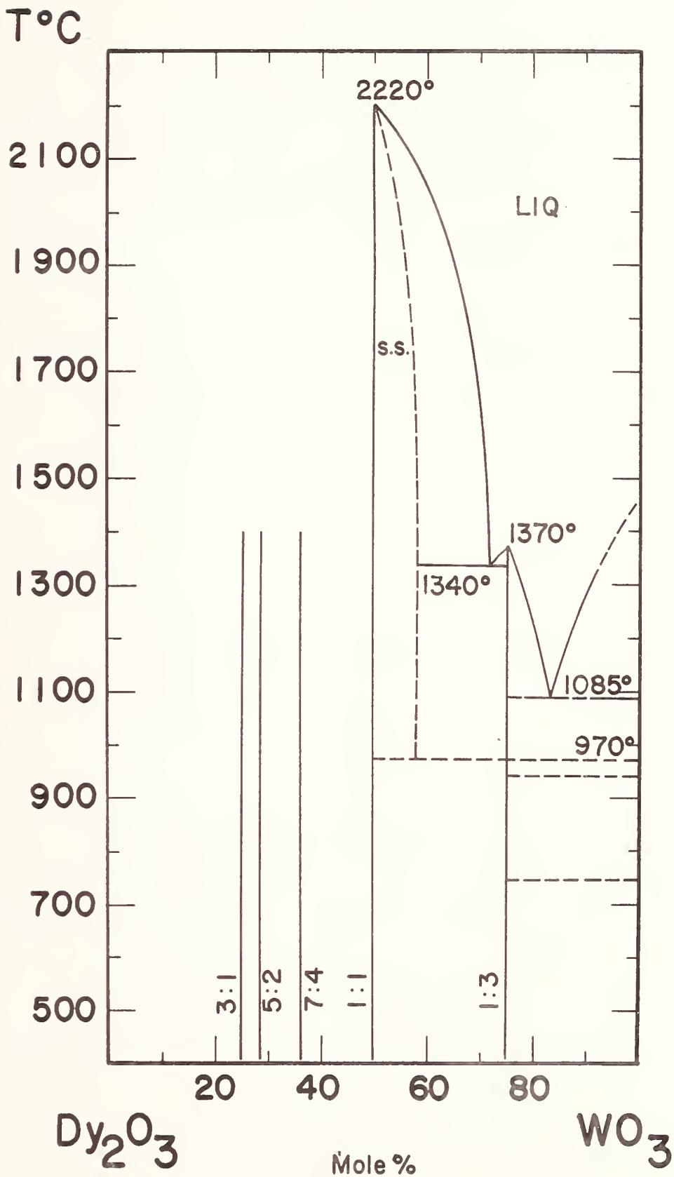
FIGURE 15. Phase relations in the system  $\text{Dy}_2\text{O}_3$ - $\text{WO}_3$
