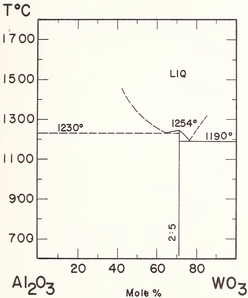
FIGURE 25. Phase relations in the system  $\text{Al}_2\text{O}_3$ - $\text{WO}_3$
