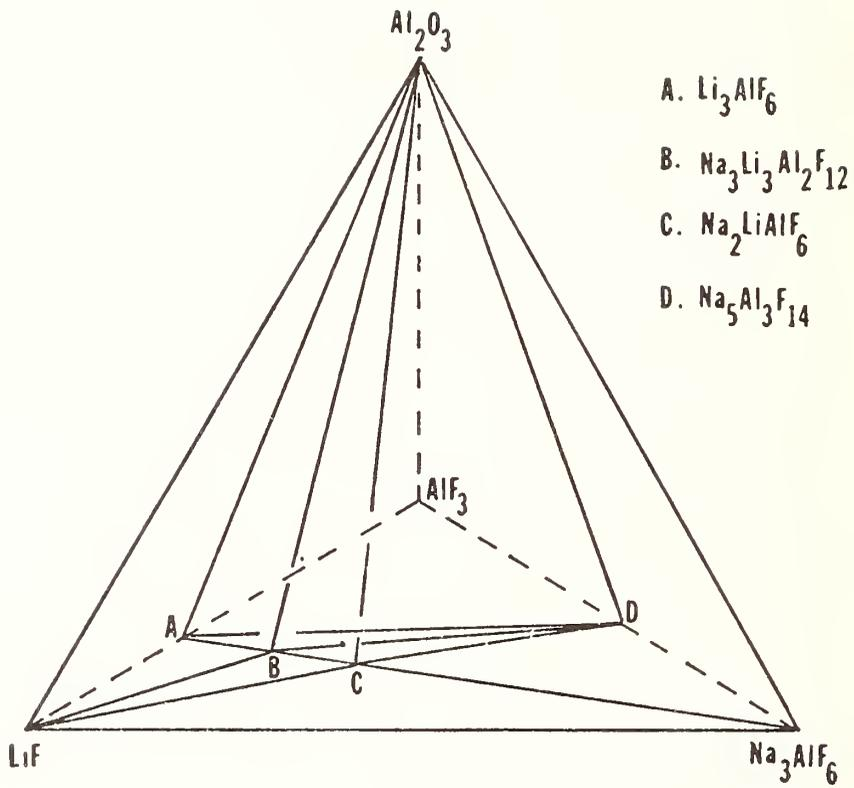
Figure 26. Possible phase diagram for the system  $\text{Na}_3\text{AlF}_6\text{-AlF}_3\text{-LiF-Al}_2\text{O}_3$ .
