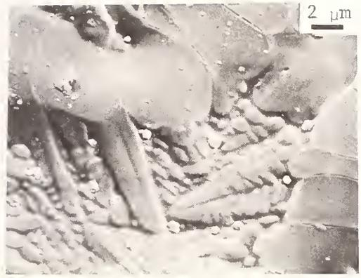
8b) High magnification detail of (a). Dendritic texture suggests growth from melt upon quench. Grains at top and right may represent solids in equilibrium with melt.
