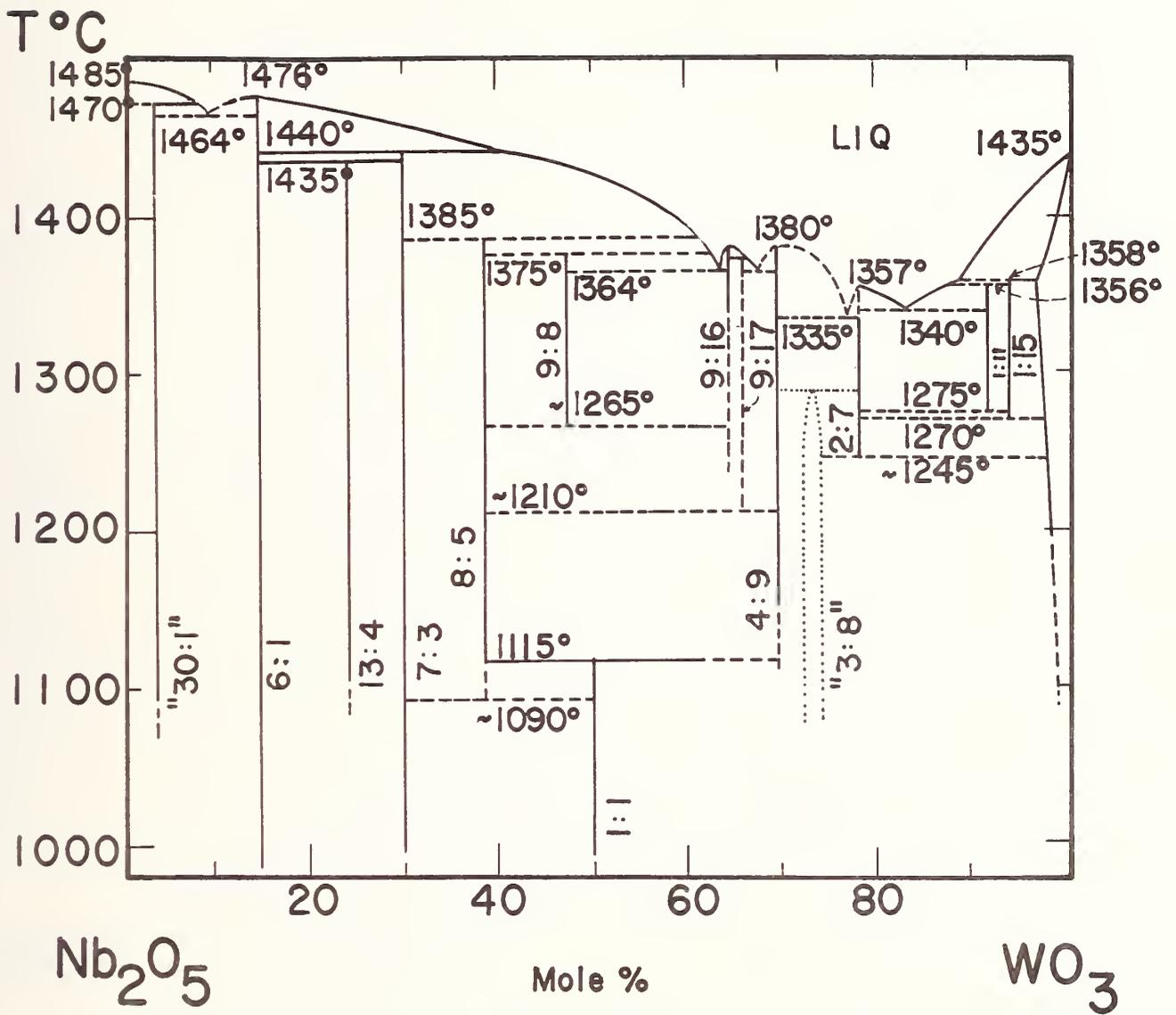
FIGURE 19. Phase relations in the system  $\text{Nb}_2\text{O}_5$ - $\text{WO}_3$
