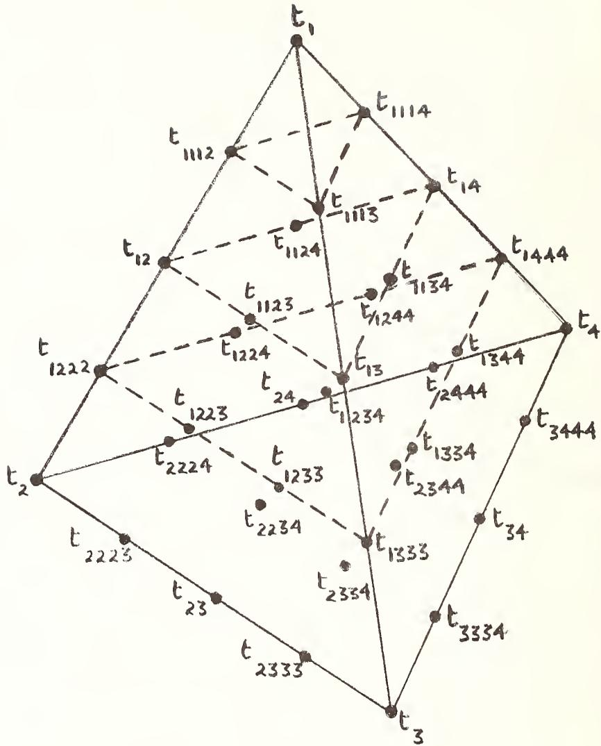
FIGURE 23. Nomenclature for Solidus Temperatures in a Quaternary System According to the Quartic Model
