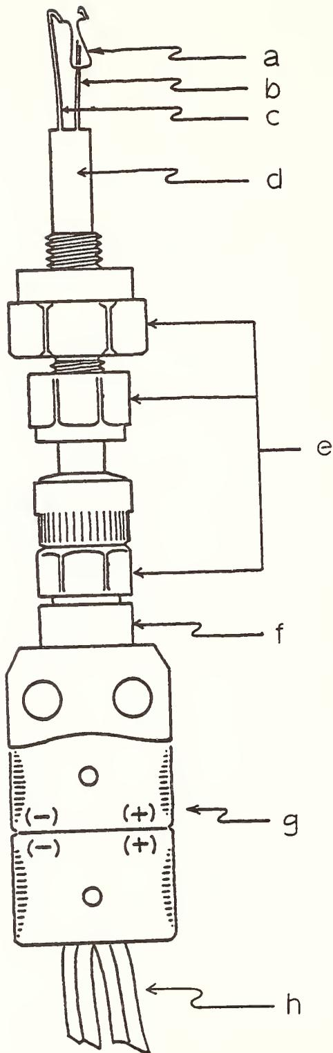
Fig. 4 Complete hot-wire assembly; (a) thermocouple, (b) Pt support and lead, (c) Pt-10% Rh support and lead, (d)  $\text{Al}_2\text{O}_3$  insulator, (e) Swage lok fittings, (f) tube clamp, (g) Omega Eng. thermocouple connector, and (h) compensating wire for Pt/Pt-10% Rh thermocouples (Modified from Ref. 22).
