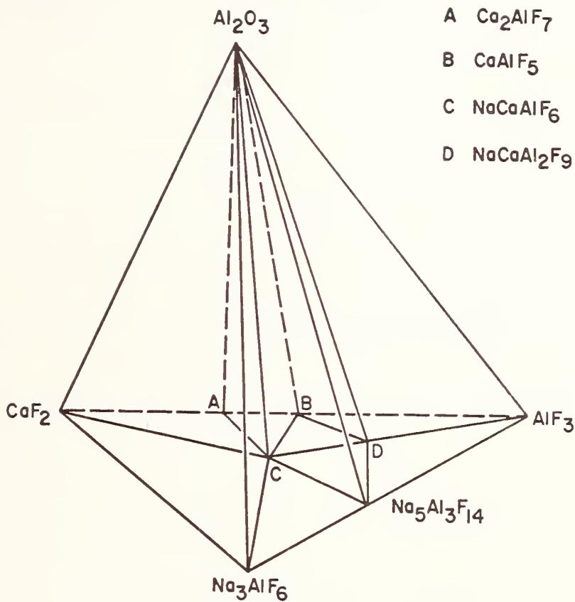
Figure 25. Subsolidus Compatibility Relationships in the system  $\text{Na}_3\text{AlF}_6$ - $\text{AlF}_3$ - $\text{CaF}_2$ - $\text{Al}_2\text{O}_3$  <sup>(56)</sup>.
