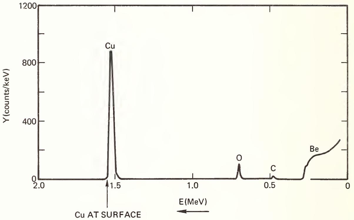
Figure 6. Actual ion backscattering spectrum of yield versus energy of backscattered ions for 2 MeV incident ions. Note that energy increases to the left.
