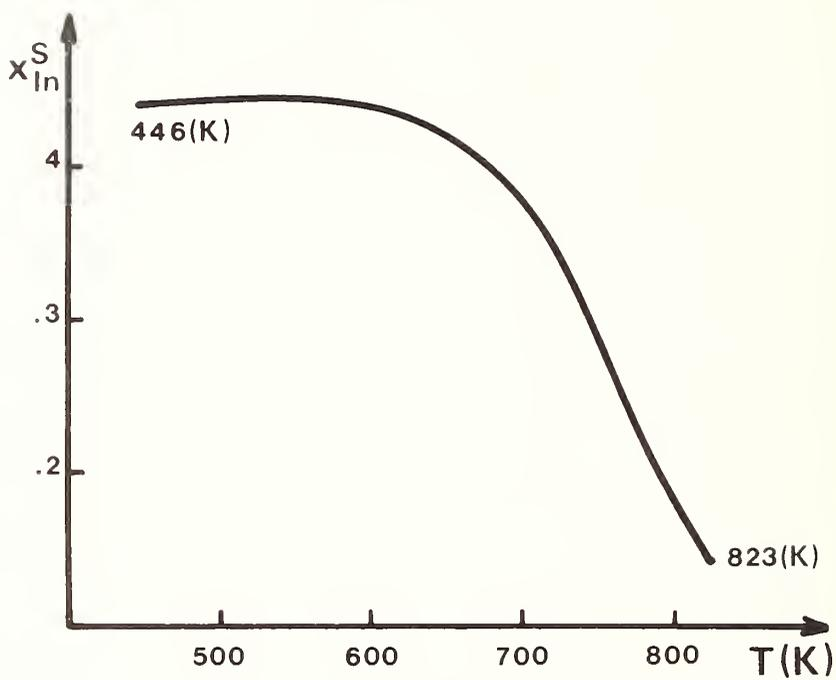
Fig. 5 : Variation of the molar fraction of In the quasi-binary solid solution with respect to temperature.
