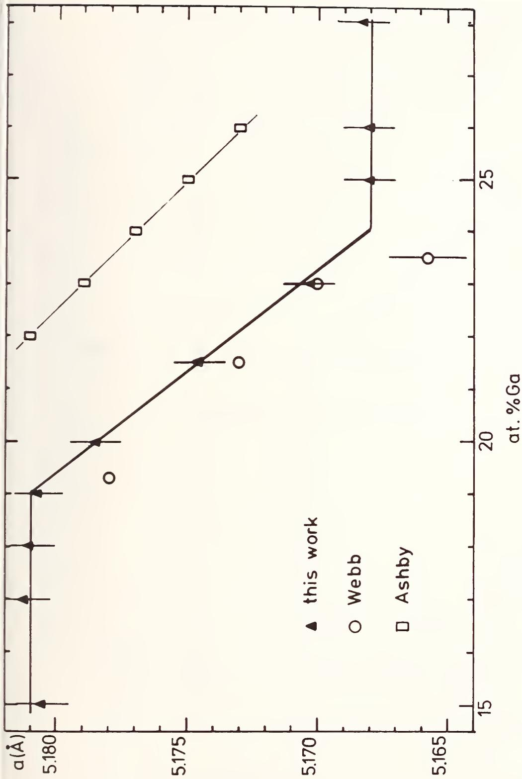
FIGURE 8. The variation of the lattice constant for the Al<sub>5</sub> phase of the Nb-Ga system. The values of Ashby et al. {11} can be brought to cover with those of Webb et al. {8} and Jorda et al. {5} by a shift of 3 at.% Ga.
