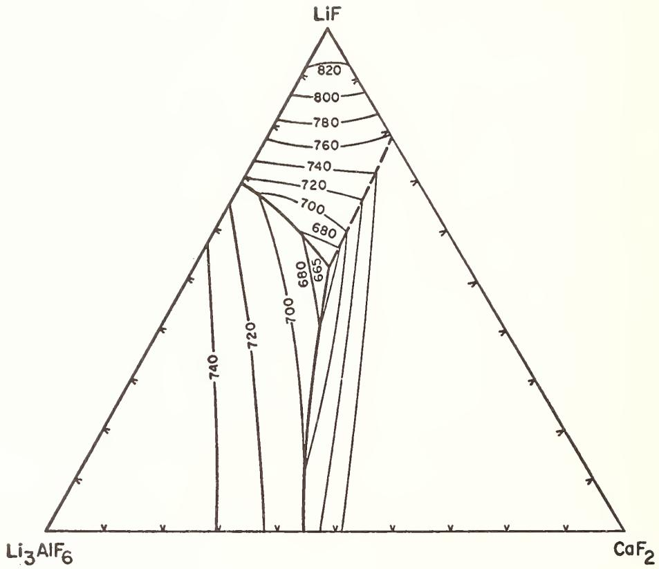
Figure 23. System  $\text{Li}_3\text{AlF}_6\text{-LiF-CaF}_2$  <sup>(99)</sup>.
