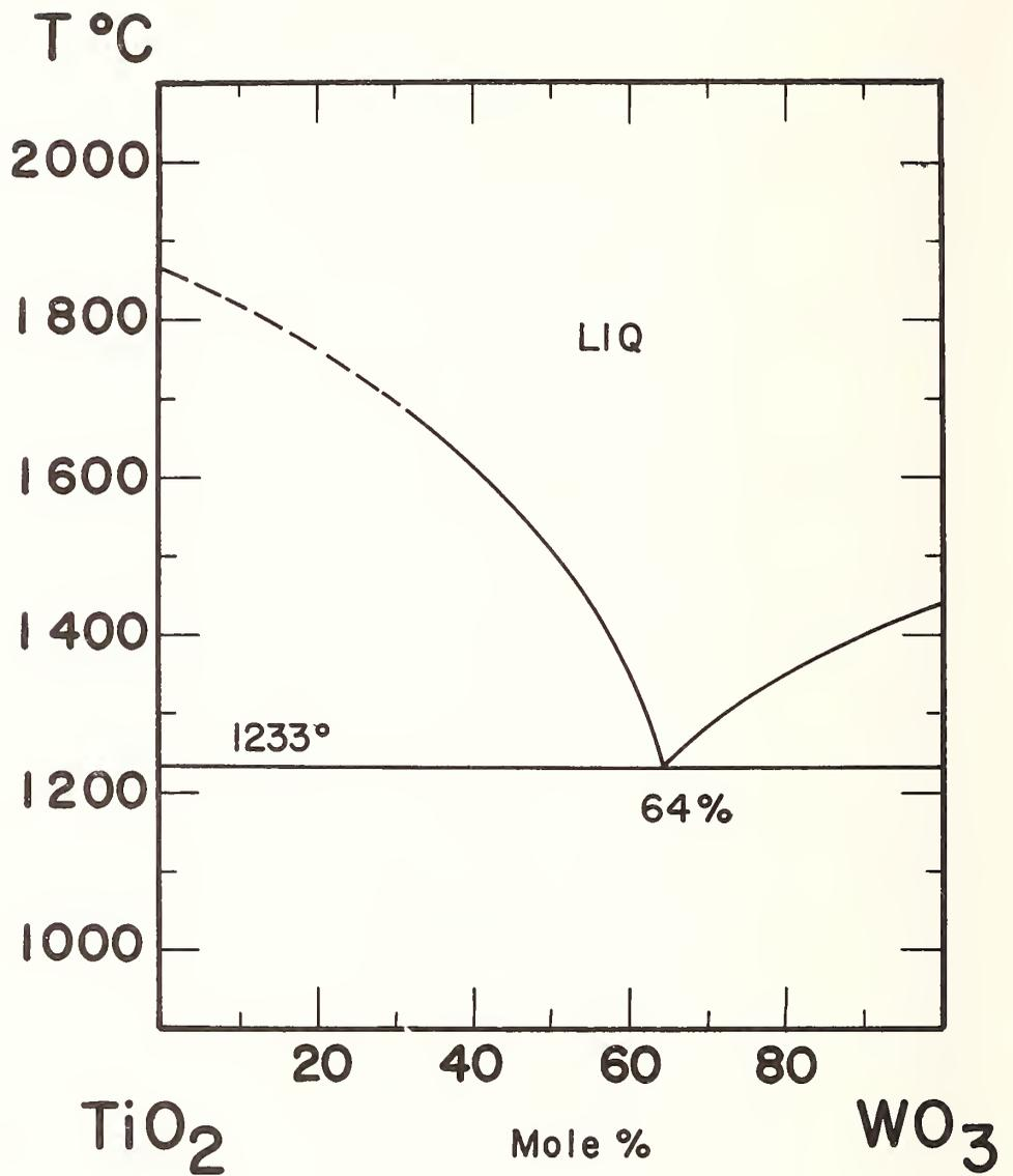
FIGURE 16. Phase relations in the system  $\text{TiO}_2$ - $\text{WO}_3$
