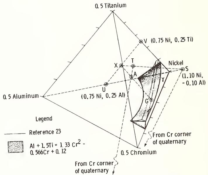
Figure 1. - Nickel-rich region of Ni-Al-Cr-Ti system at 750° C.
