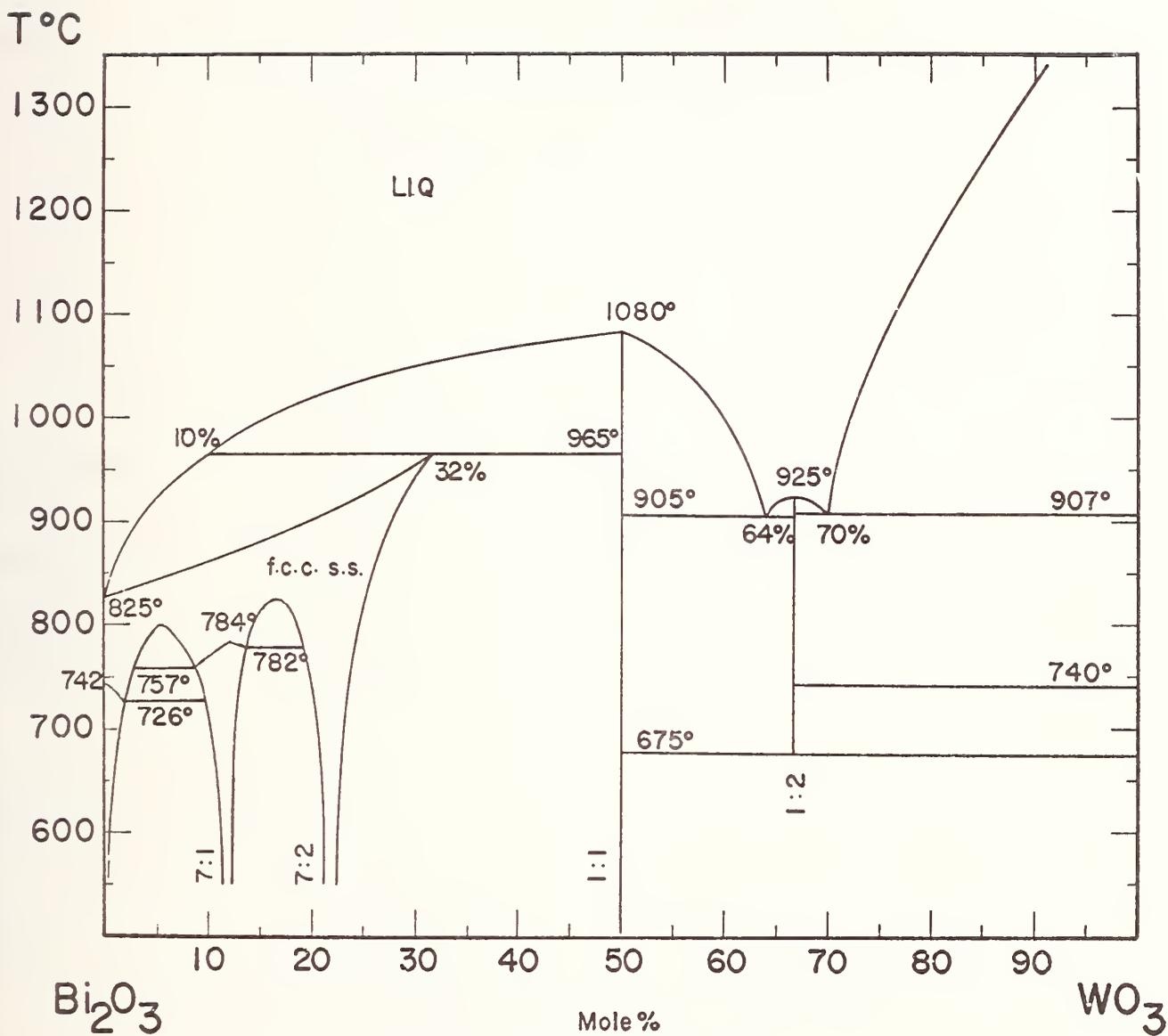
FIGURE 29. Phase relations in the system  $\text{Bi}_2\text{O}_3$ - $\text{WO}_3$
