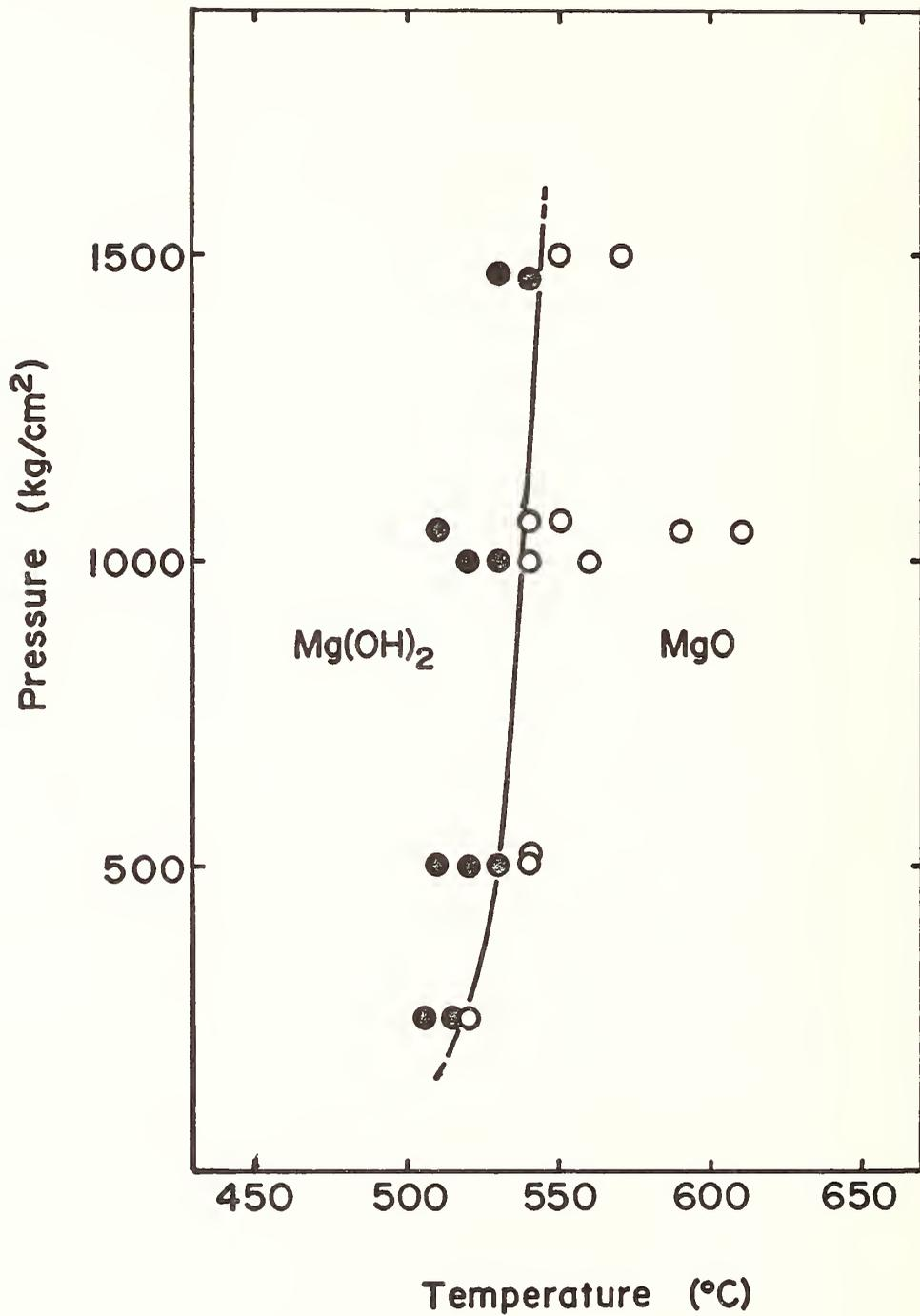
Fig.3 P-T diagram of the system MgO-Mg(OH)<sub>2</sub> in 5 mol% KCl solution.
