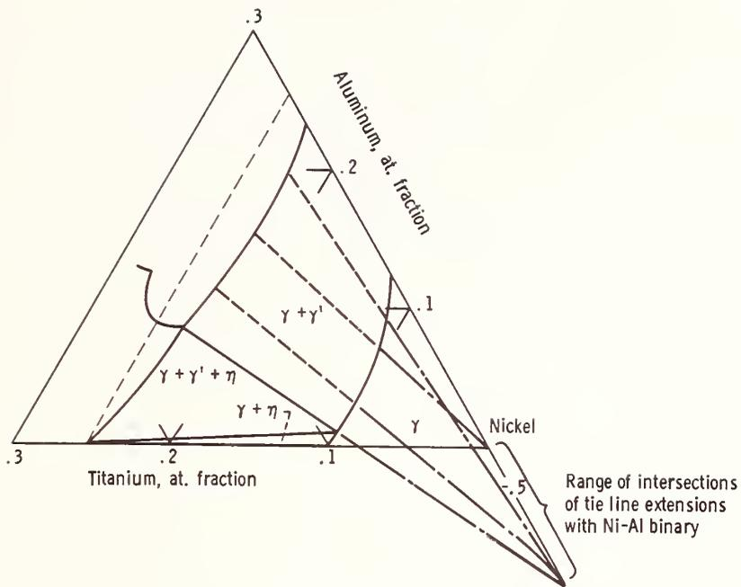
Figure 4. - Nickel-rich region of Ni-Ti-Al system at 750<sup>o</sup> C (after Taylor and Floyd (ref. 22)).
