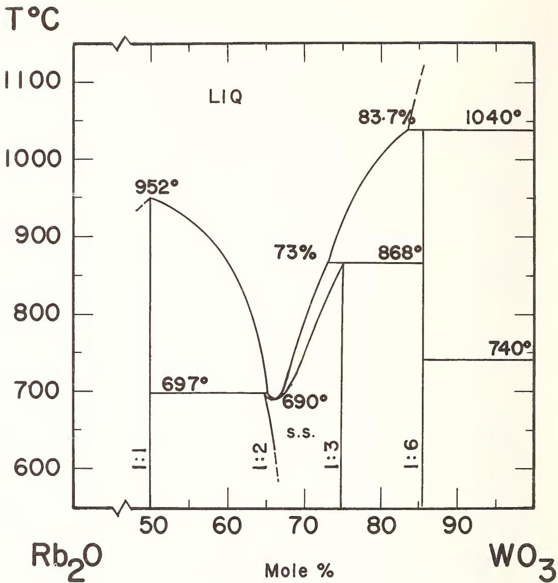
FIGURE 4. Phase relations in the system  $\text{Rb}_2\text{O}\cdot\text{WO}_3-\text{WO}_3$
