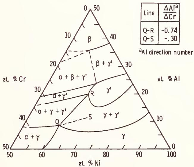
Figure 5. - The Ni-Cr-Al phase diagram at 850<sup>o</sup> C from reference 20.
