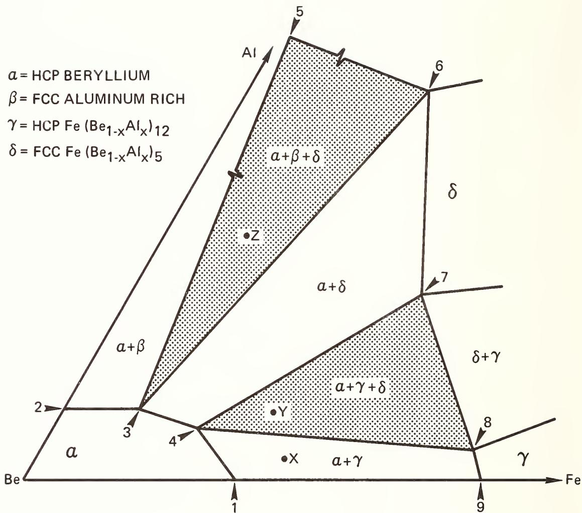
Figure 12. Schematic ternary phase diagram for Be-Fe-Al system showing relationship between two-phase and three-phase regions. Sample concentration during anneals must be in three-phase region, e.g., at points Y and Z, but not at X.
