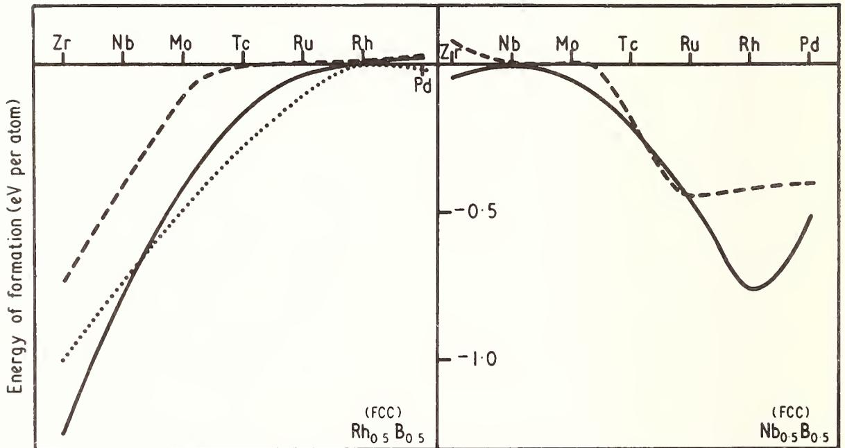
Fig. 6. van der Rest et al.'s estimates<sup>12</sup> of the energy of formation of equiconcentrational rhodium and niobium based alloys with elements of the second transition metal row having the fcc structure. The dashed lines are their standard solutions, the dotted obtained with an improved model density of states. Comparison is made with thermodynamic estimates of Kaufman (solid lines).
