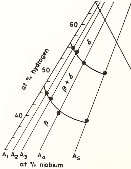
Fig. 4—Isothermal section for the ternary system Zr-Nb-H at 700°C. A<sub>1</sub>, 0.0 at. pct Nb; A<sub>2</sub>, 2.46 at. pct Nb; A<sub>3</sub>, 4.91 at. pct Nb; A<sub>4</sub>, 9.84 at. pct Nb; A<sub>5</sub>, 19.71 at. pct Nb.
