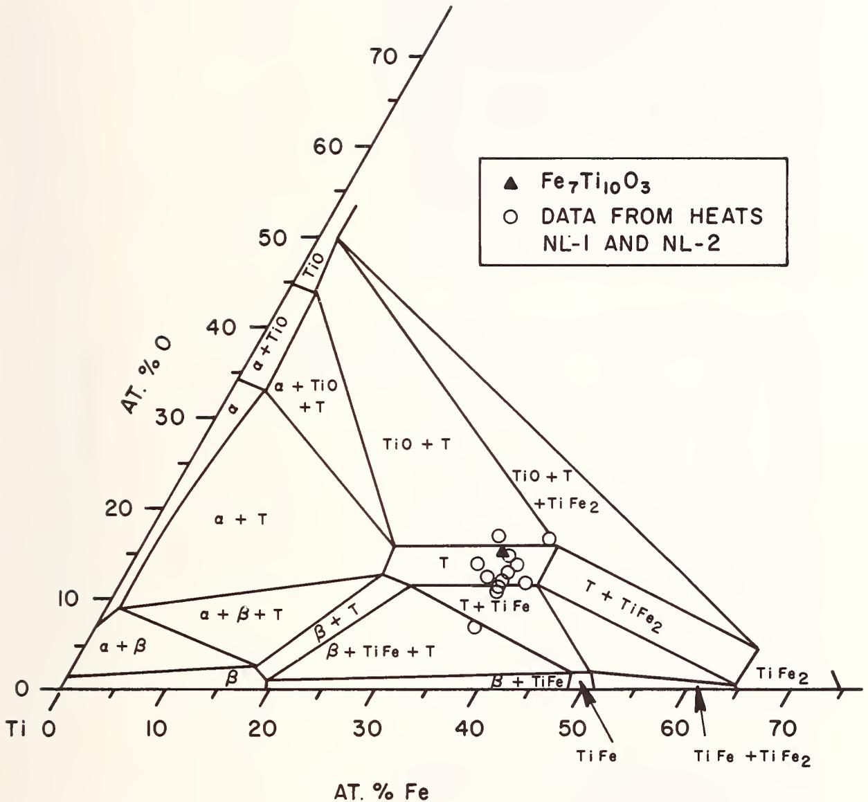
**FIGURE 6** - MICROPROBE DATA FOR O-RICH SECOND PHASE PARTICLES FOUND IN MICROSTRUCTURE OF O-CONTAINING FeTi HEATS COMPARED TO THE Ti-Fe-O TERNARY PHASE DIAGRAM OF ROSTOKER (REF. 9). HEATS STUDIED CORRESPOND TO FIG. 7b AND c.
