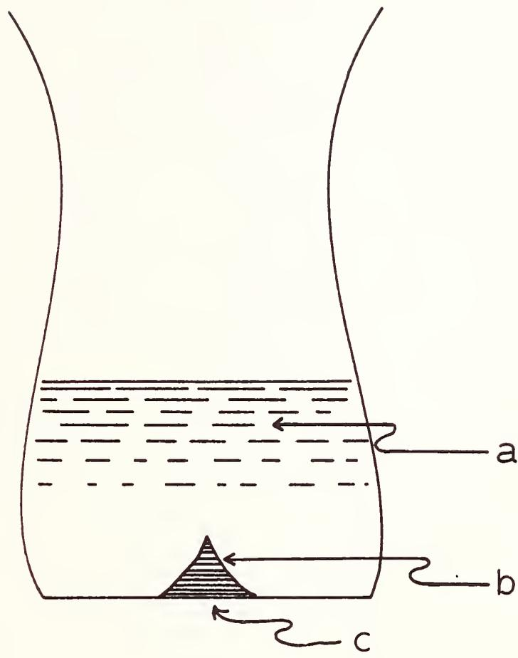
Fig. 3 Schematic representation of hot-wire thermocouple; (a) melt, (b) first crystal, and (c) thermocouple junction (Modified from Ref. 22).
