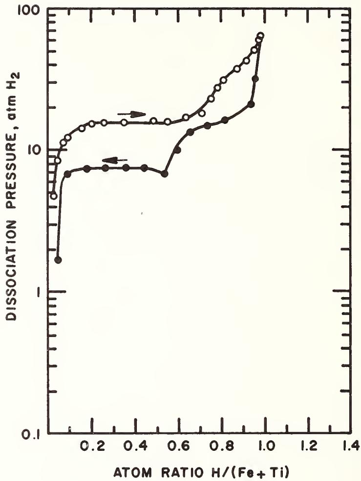
**FIGURE 3** - FeTi-H CHARGING AND DISCHARGING CURVES AT 40°C.
