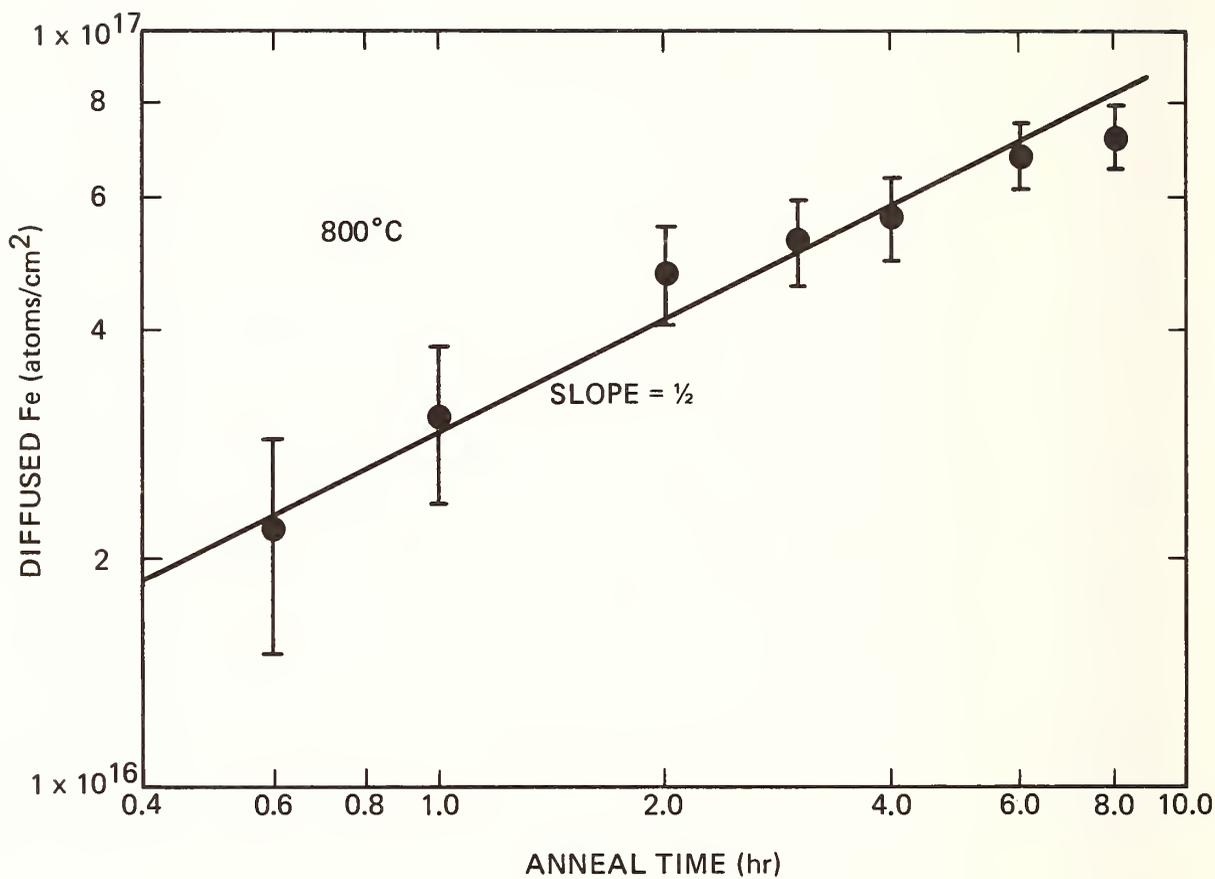
Figure 10. Time dependence of the amount of iron diffused into sample from implanted region during anneal at 800°C. Slope of 1/2, predicted from analysis, supports validity of assumptions.
