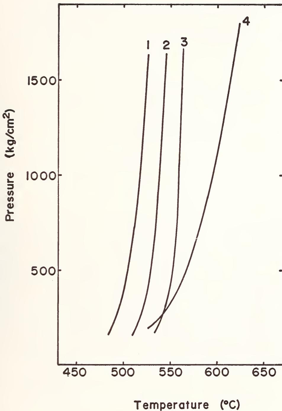
Fig.4 P-T diagram of the system MgO-Mg(OH)<sub>2</sub> in 5 mol% LiCl soln.(1), 5 mol% KCl soln. (2), 5 mol% NaCl soln.(3) and pure water (4).
