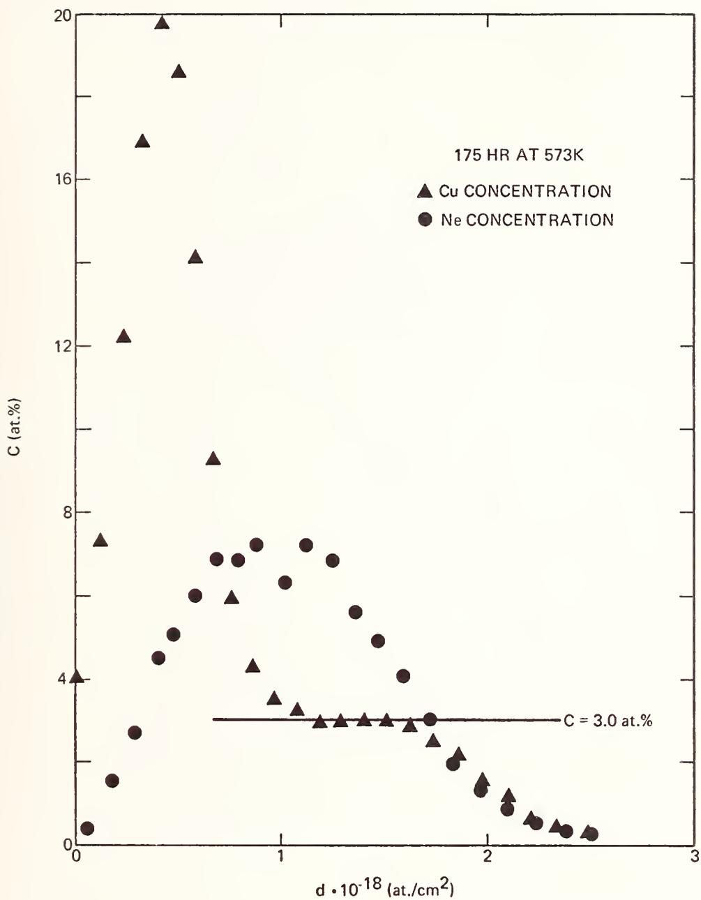
Figure 11. Concentration profile after annealing for enhanced diffusion experiment. Note overlays of plateau region of copper concentration and neon profile as implanted.
