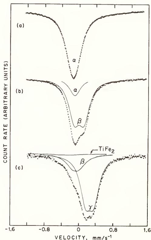
Fig. 3. Room temperature Mössbauer absorption spectra for TiFeH<sub>x</sub>. The line through the data points is a least-squares fit which is the sum of the contributions from the individual phases. (a) x = 0.1, 100%  $\alpha$  phase. (b) x = 0.9, 19%  $\alpha$  phase and 81%  $\beta$  phase. (c) x = 1.7, which consists of 23%  $\beta$  phase, 75%  $\gamma$  phase, and 2% of spurious TiFe<sub>2</sub>. (After Ref. 13).
