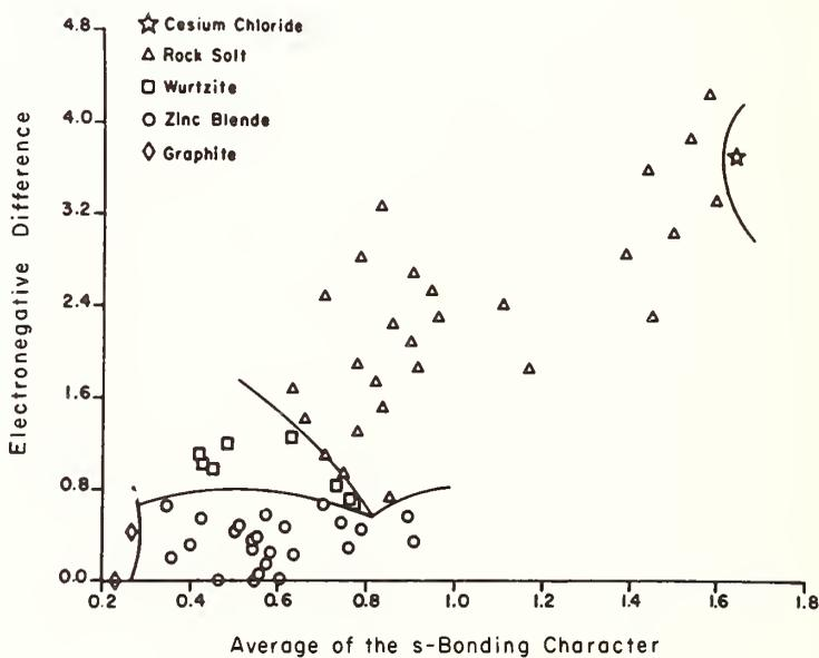
Fig. 11. Mapping of the structures of the  $AB_{8-N}$  "octet" compounds as a function of electronegativity difference and average s fraction of bonding as obtained by St. John and Bloch<sup>28</sup>.
