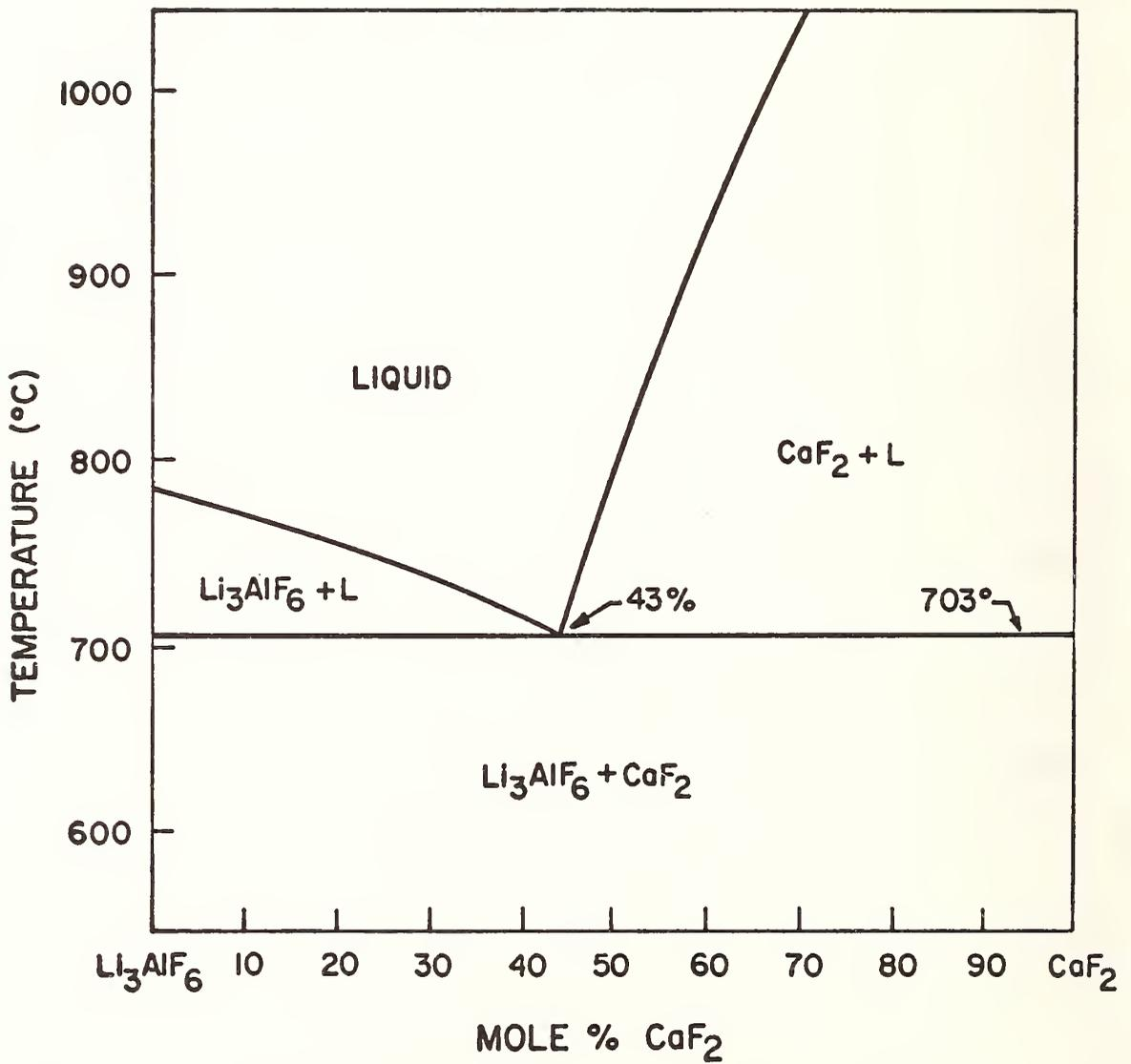
Figure 14. System  $\text{Li}_3\text{AlF}_6$ - $\text{CaF}_2$  <sup>(99)</sup>.
