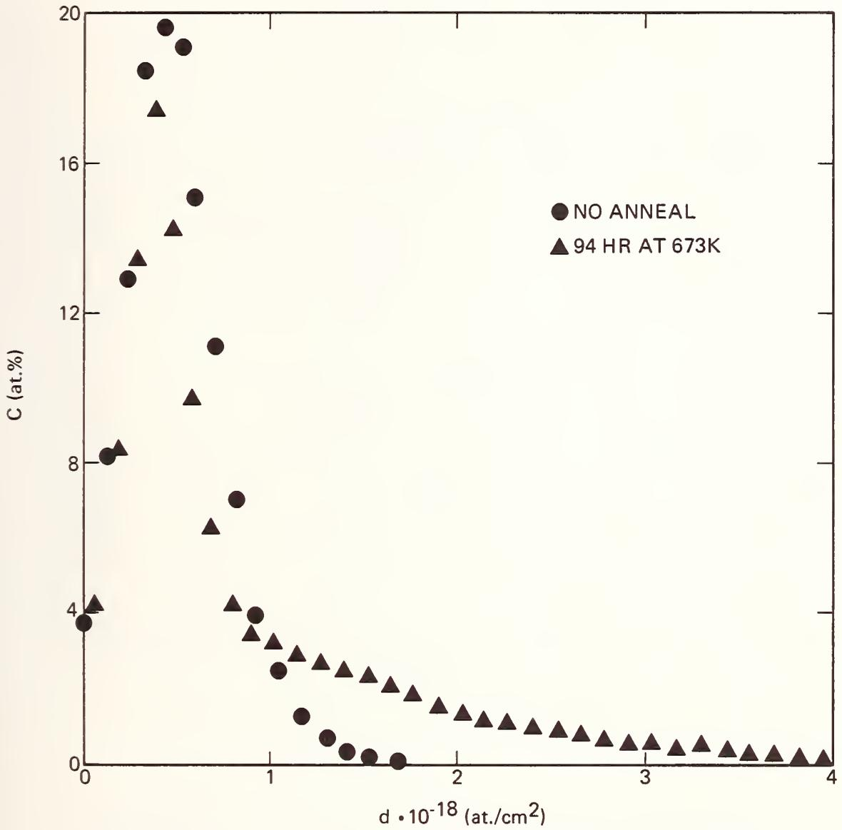
Figure 7. Concentration profile of copper implanted into beryllium before and after anneal, showing discontinuity in actual data.
