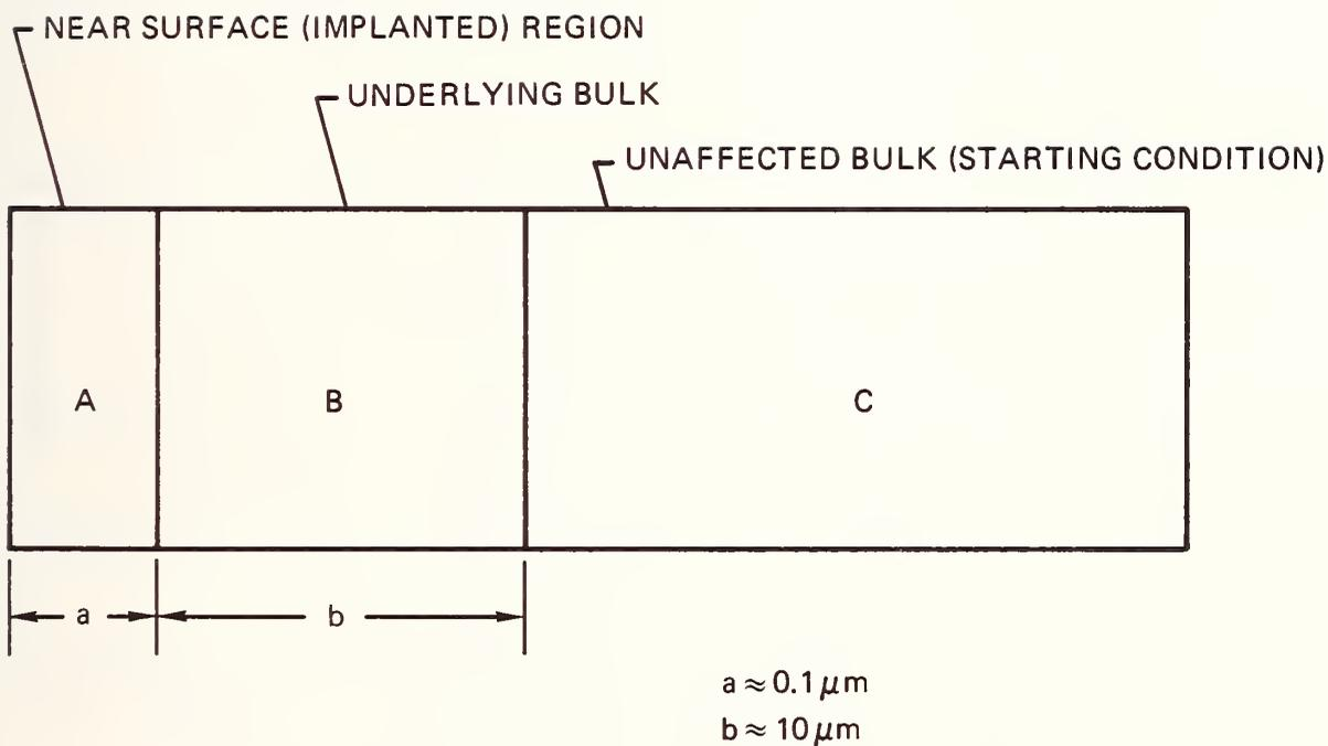
Figure 1. Schematic of sample showing implanted region (A), underlying bulk (B), and unaffected bulk (C). Diffusion of solute from region A occurs in region B during annealing.
