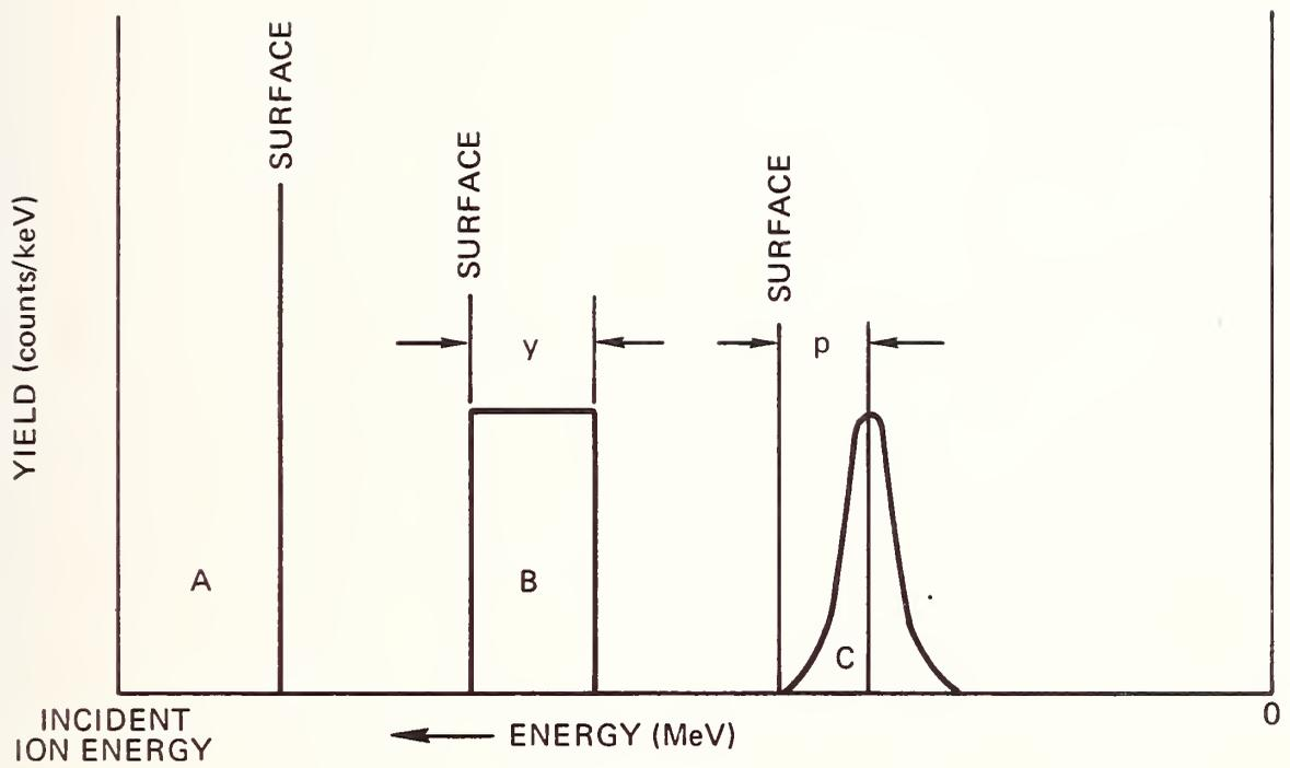
Figure 3. Schematic ion backscattering spectrum of sample containing three impurities: A, B, and C where  $m_A > m_B > m_C$ . In each case the impurity distribution is located near the surface.
