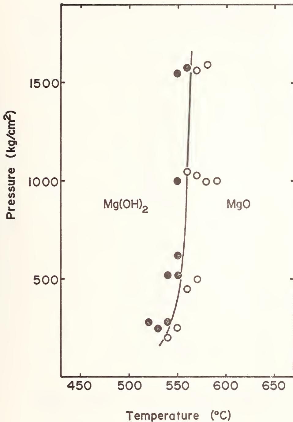
Fig.2 P-T diagram of the system MgO-Mg(OH)<sub>2</sub> in 5 mol% NaCl solution.
