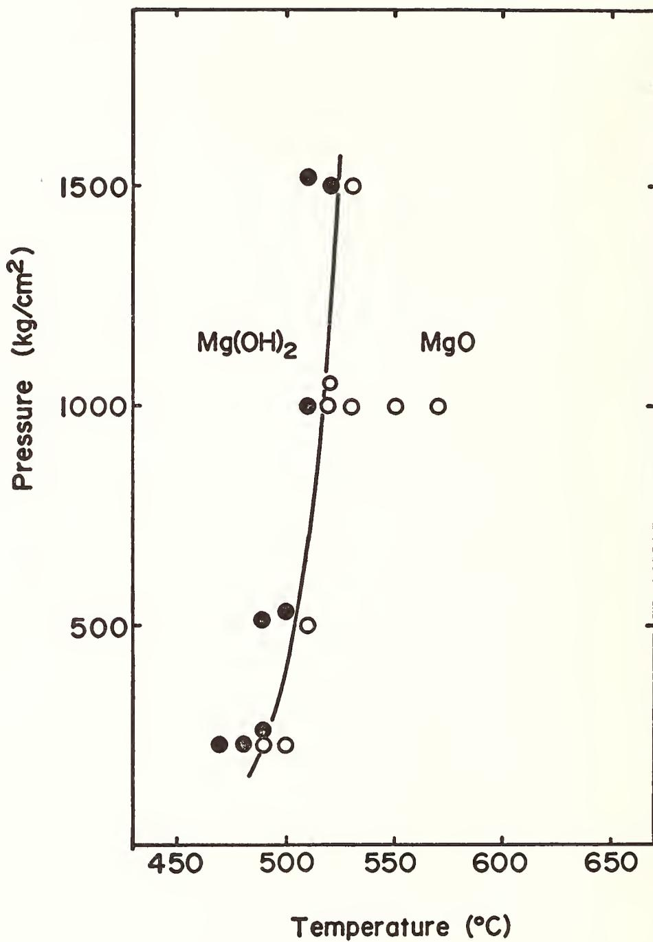
Fig.1 P-T diagram of the system MgO-Mg(OH)<sub>2</sub> in 5 mol% LiCl solution.
