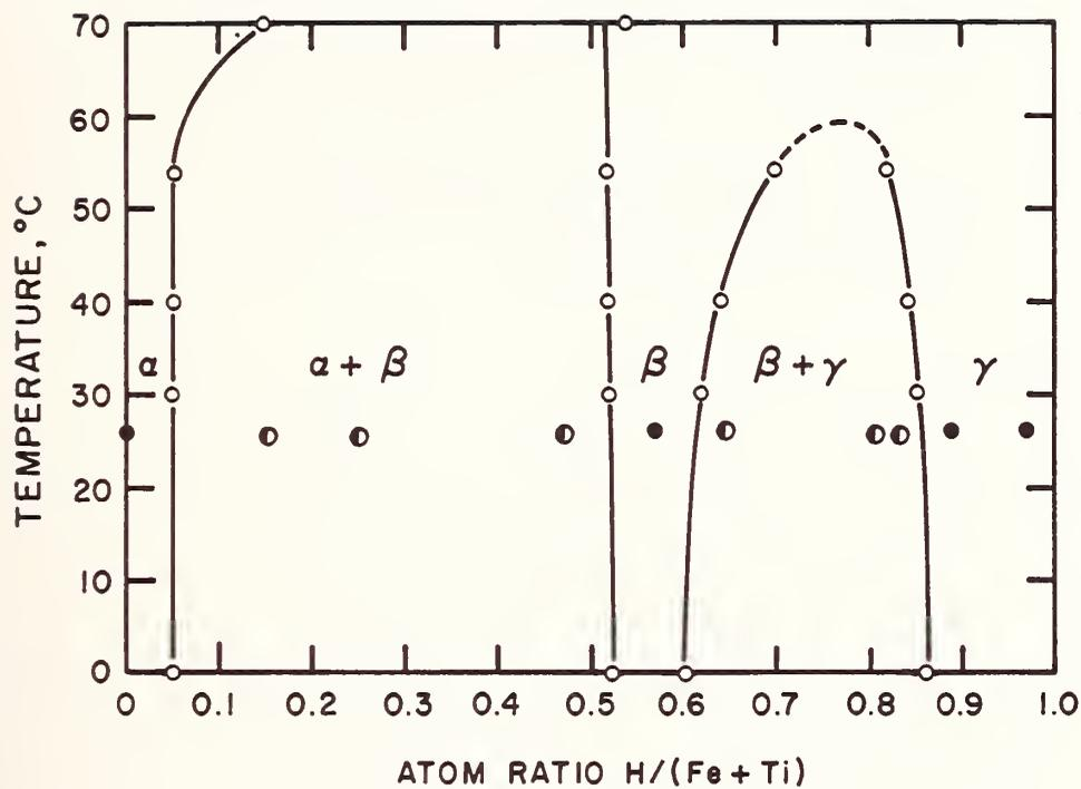
**FIGURE 12** - PHASE DIAGRAM OF THE FeTi-H SYSTEM AS DERIVED FROM PRESSURE - COMPOSITION DATA. X-RAY DIFFRACTION PATTERNS TAKEN AT COMPOSITIONS INDICATED: ●, ONE SOLID PHASE, ○, TWO SOLID PHASES.  $\alpha = \text{FeTi}$ ,  $\beta \approx \text{FeTiH}$ ,  $\gamma \approx \text{FeTiH}_2$ .
