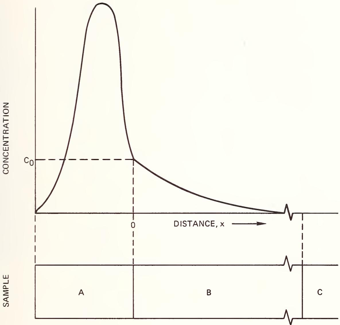
Figure 5. Schematic of diffused tail region showing discontinuity at  $C_0$  and the concentration profile for the regions of interest in the sample.
