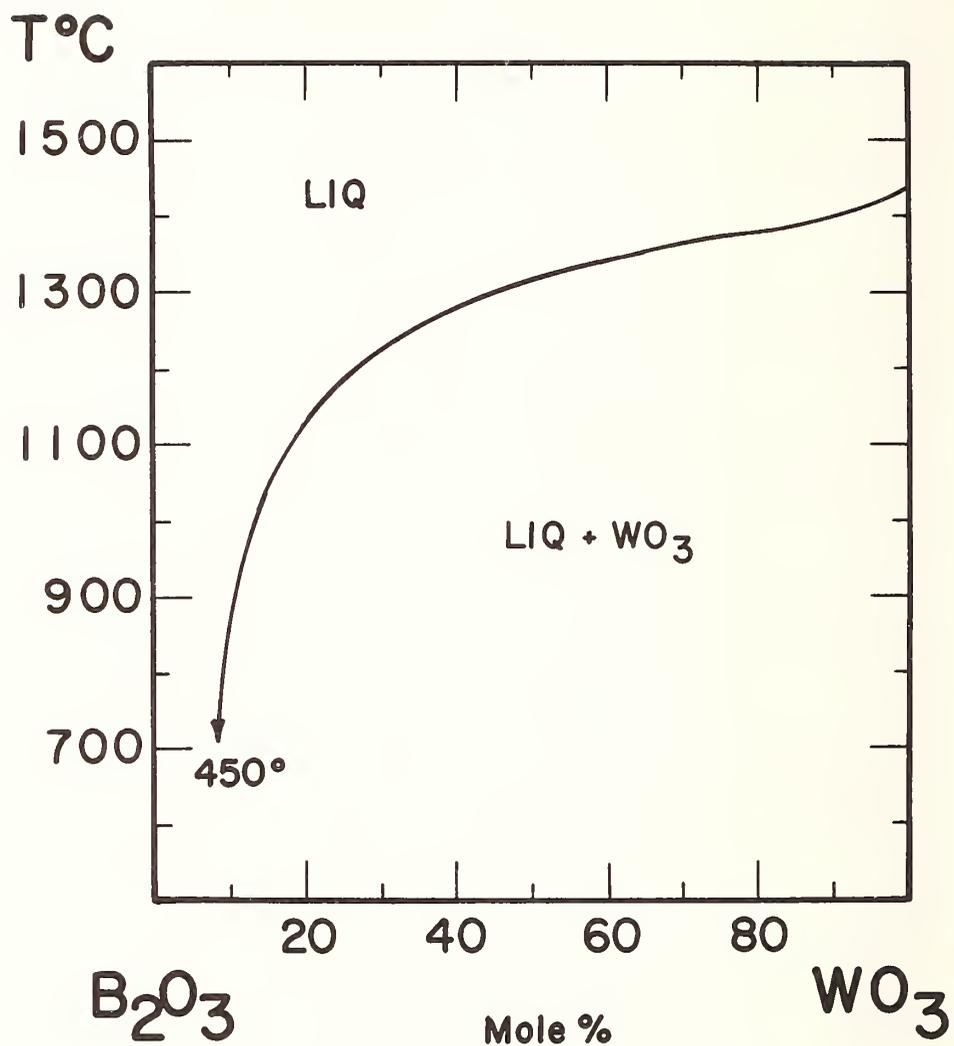
FIGURE 24. Phase relations in the system B<sub>2</sub>O<sub>3</sub>-WO<sub>3</sub>
