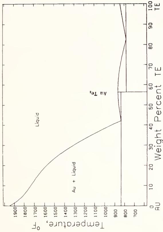
Fig. 4. (a) AuTe phase diagram as displayed on a graphics terminal, (b) AuTe diagram after software generated transformation to weight percent and degrees Fahrenheit. The scale lengths have also been altered slightly.
