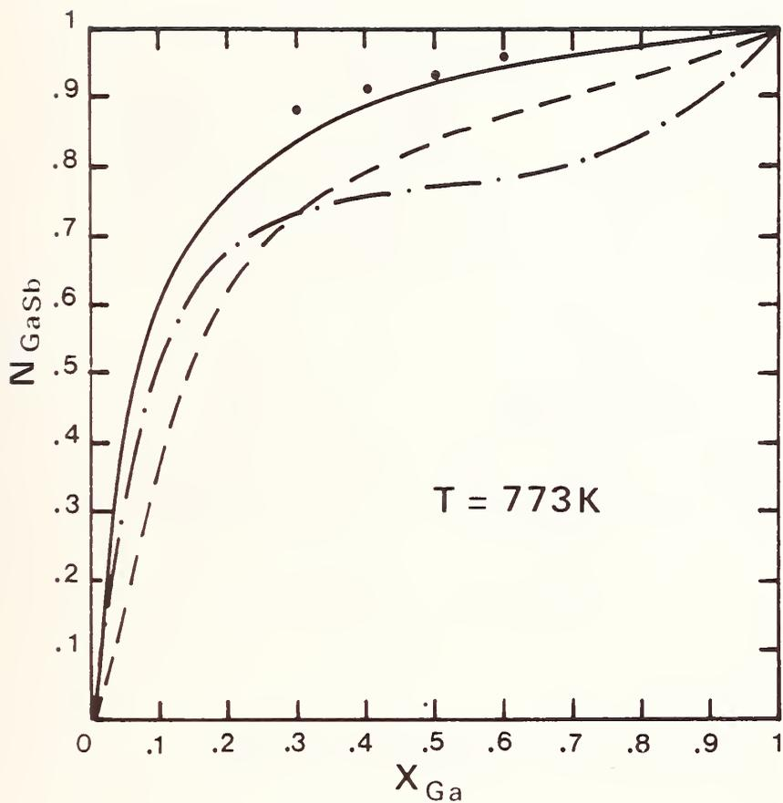
Fig. 6 : Variation of  $N_{GaSb}^S = f(x_{Ga}^1)$  at 773K. • Experimental values (G.A. Antypas, J. Electrochem. Soc., 1970, 8, 3, 259)
