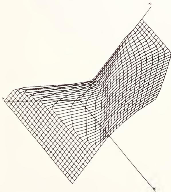
Fig. 2. Two views of a hypothetical pressure-composition-temperature plot of a metal-hydrogen system with properties similar to Pd-H. Vertical Y axis represents pressure, the Z axis composition, and the X axis temperature. The grid size is 30 points by 30 points.
