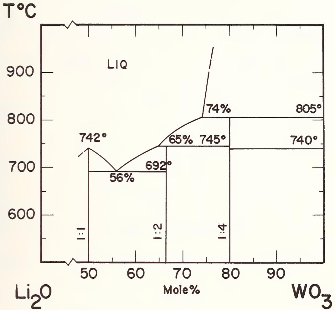
FIGURE 1. Phase relations in the system  $\text{Li}_2\text{O}\cdot\text{WO}_3-\text{WO}_3$
