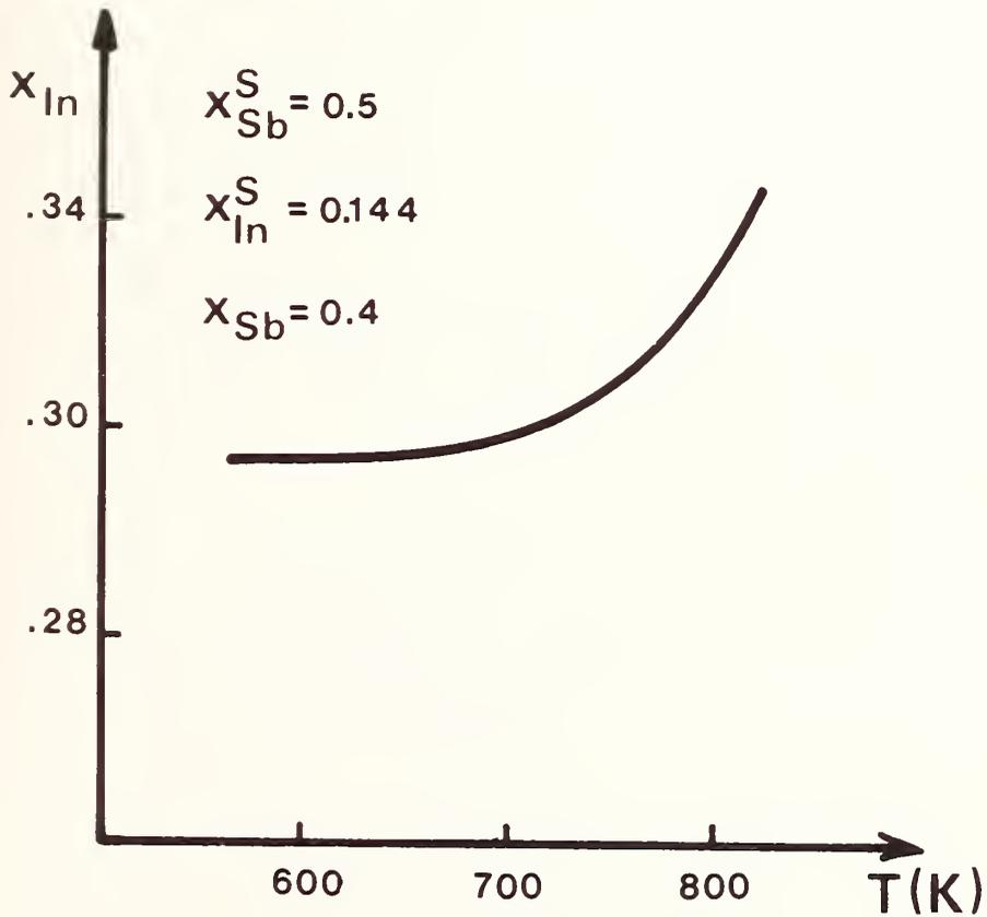
Fig. 4 : Variation of the molar fraction of In in the two phase region with respect to temperature.
