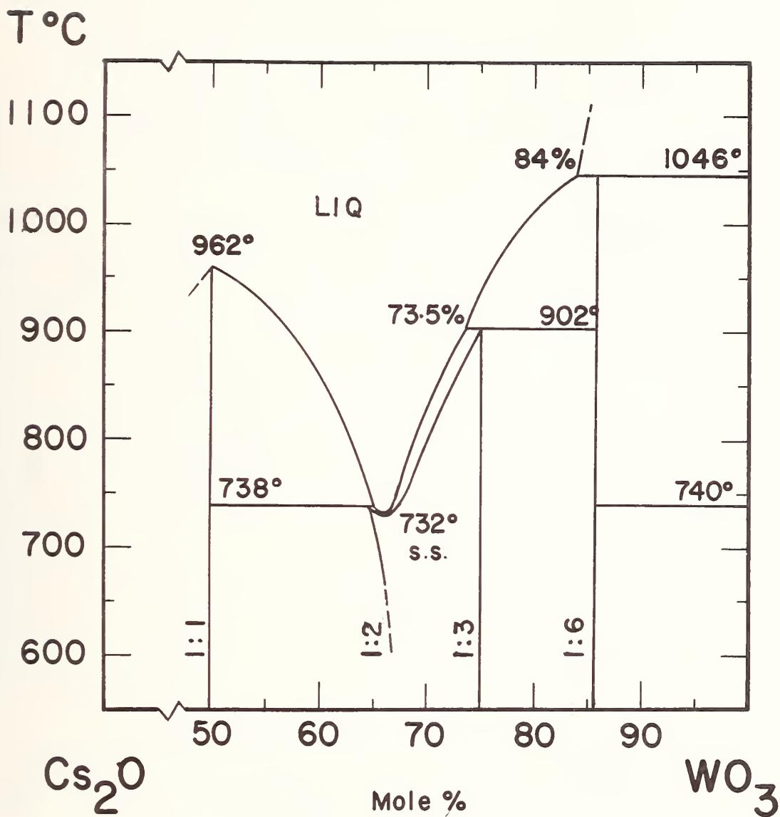
FIGURE 5. Phase relations in the system  $\text{Cs}_2\text{O}\cdot\text{WO}_3-\text{WO}_3$
