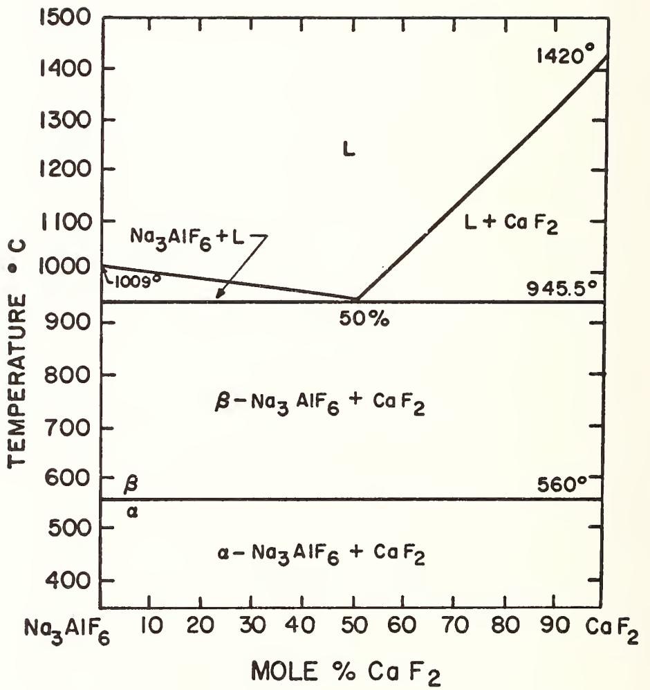
Figure 3. System Na<sub>3</sub>AlF<sub>6</sub>-CaF<sub>2</sub> <sup>(54)</sup>
