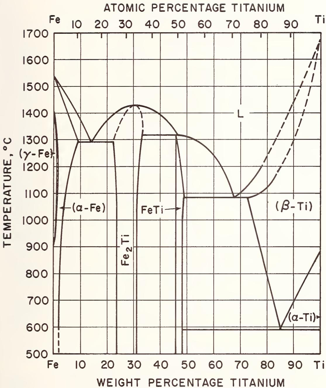
FIGURE 4 - Fe-Ti PHASE DIAGRAM. (AFTER REF. 8)
