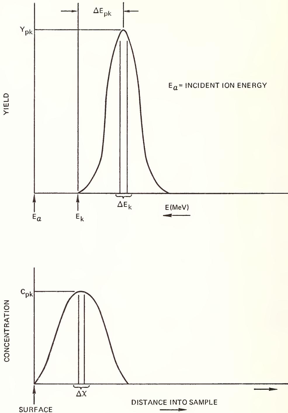
Figure 4. Schematic of ion backscattering spectrum of implanted region showing its transformation to a concentration profile. Note that  $E_k$  corresponds to element  $k$  present at the surface of the sample.
