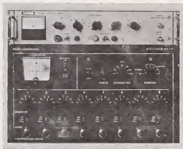
Fig. 7. — Front panel of the console containing the electronic circuitry used in the multichannel mode of operation (8).
