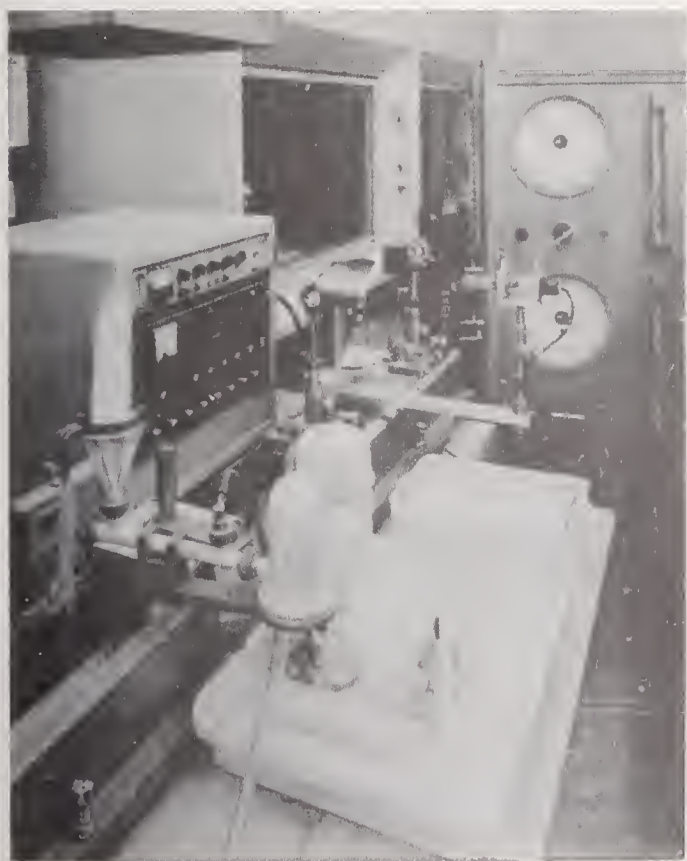
Fig. 4. — Light-tight enclosure located at the focal plane of the spectrometer. It contains seven photomultiplier tubes placed behind the exit slits carrying plate (?).
