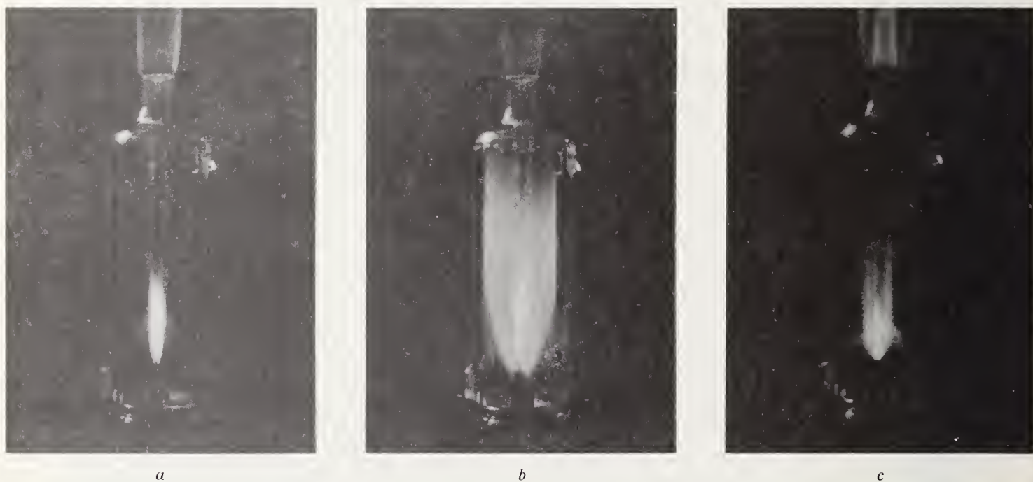
Fig. 25. — a , appearance of the dual hydrogen flame supplied with distilled water. b , same flame supplied with diluted sulfuric acid. c , same flame supplied with diluted phosphoric acid.
