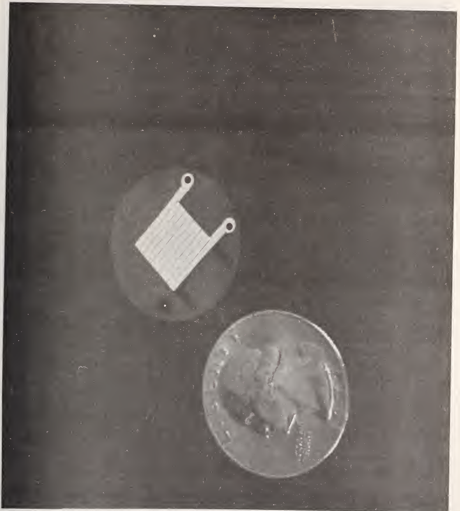
Figure 8 Complete Sensor of the RST-Meter Showing the Resistance Thermometer (on top) and Heating Element (underneath)
