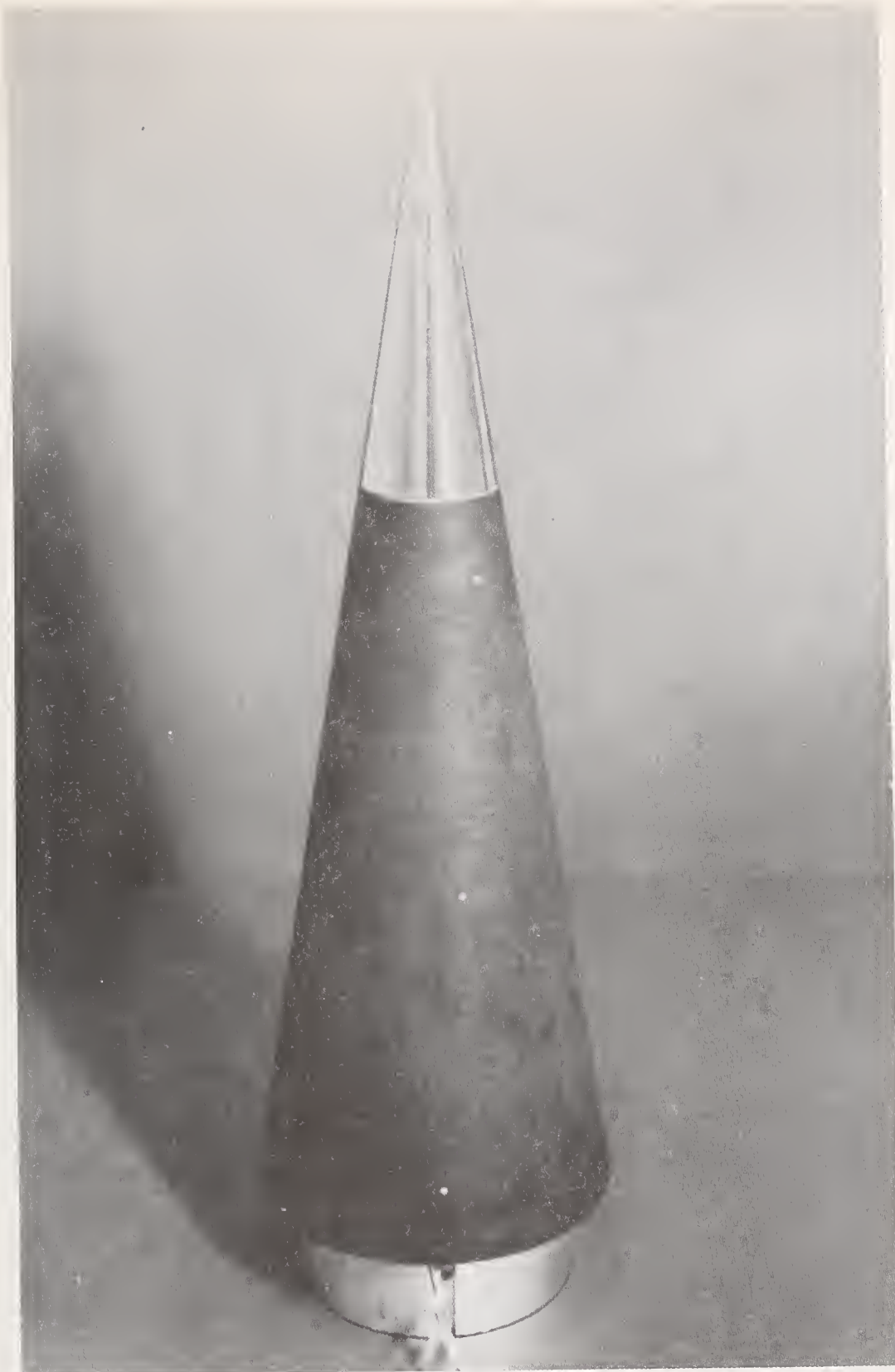
FIGURE 11 WIND TUNNEL TEST MODEL, \Delta t AND BLAM SENSORS
