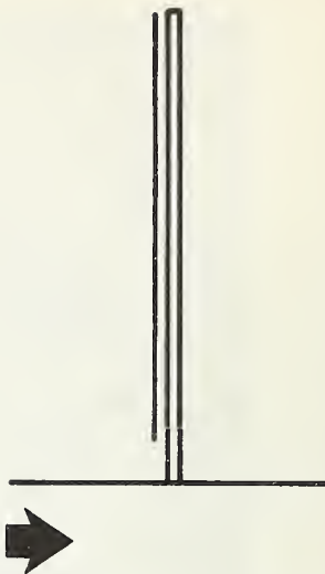
FIGURE 20. Fence Array No. 1 (7' fence) . The fastest penetration time with one man assisting, without the use of aids, was 2 seconds; the fastest penetration time with one man assisting, using canvas as an aid, was 6 seconds.
