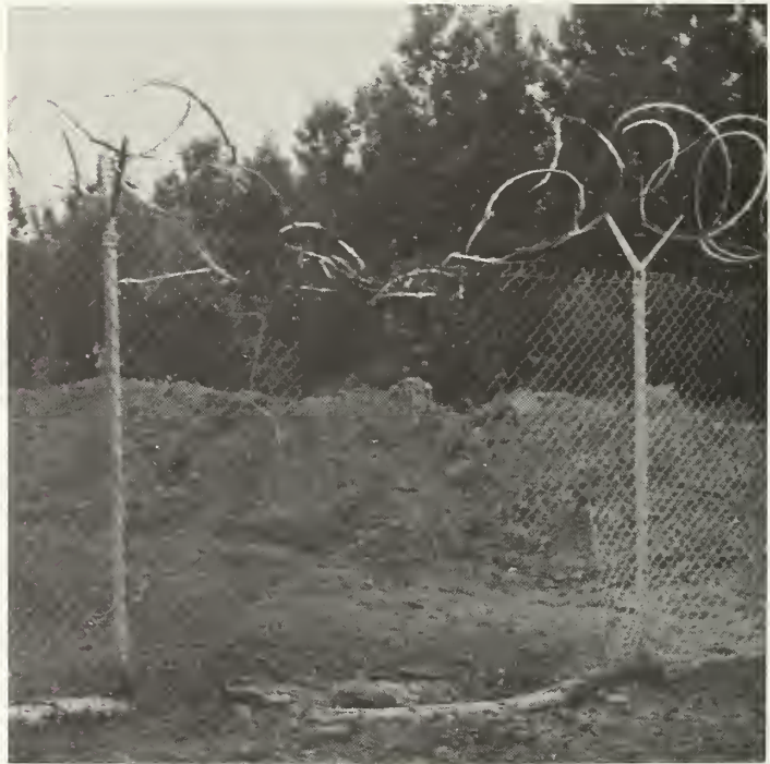
FIGURE 15B. Damage caused by bangalore torpedo .
