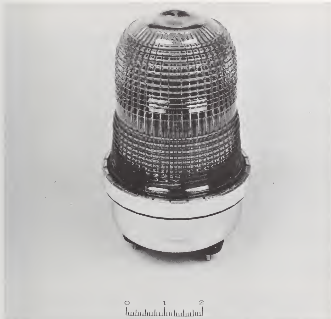
FIGURE 3.4e. Single, upright, nonreflectorized, stationary incandescent lamp is electrically flashed by current-interruption circuitry included in the unit. Colored dome contains built-in Fresnel lens (horizontal ridges) that acts as a uniform, wrap-around cylindrical lens, concentrating the light around the horizontal plane evenly over a full 360°. Dome also features superimposed straight vertical “ribs” that diffuse the light over the entire width of the dome.
