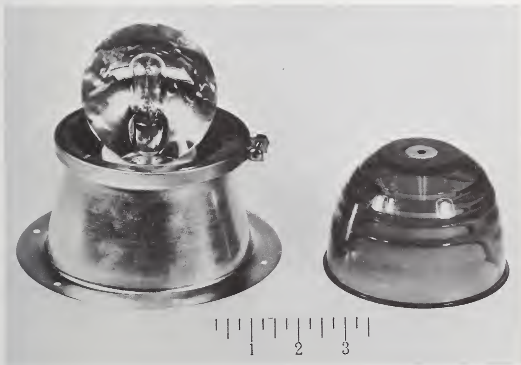
FIGURE 3.2e3. Parabolic mirror rotates around a fixed, nonreflectorized, clear incandescent lamp with its axis vertical. Unit shown has an upright lamp under a colored dome (shown removed for clarity) containing a Fresnel lens (ridges) that further adjusts the vertical spread of the beam.
