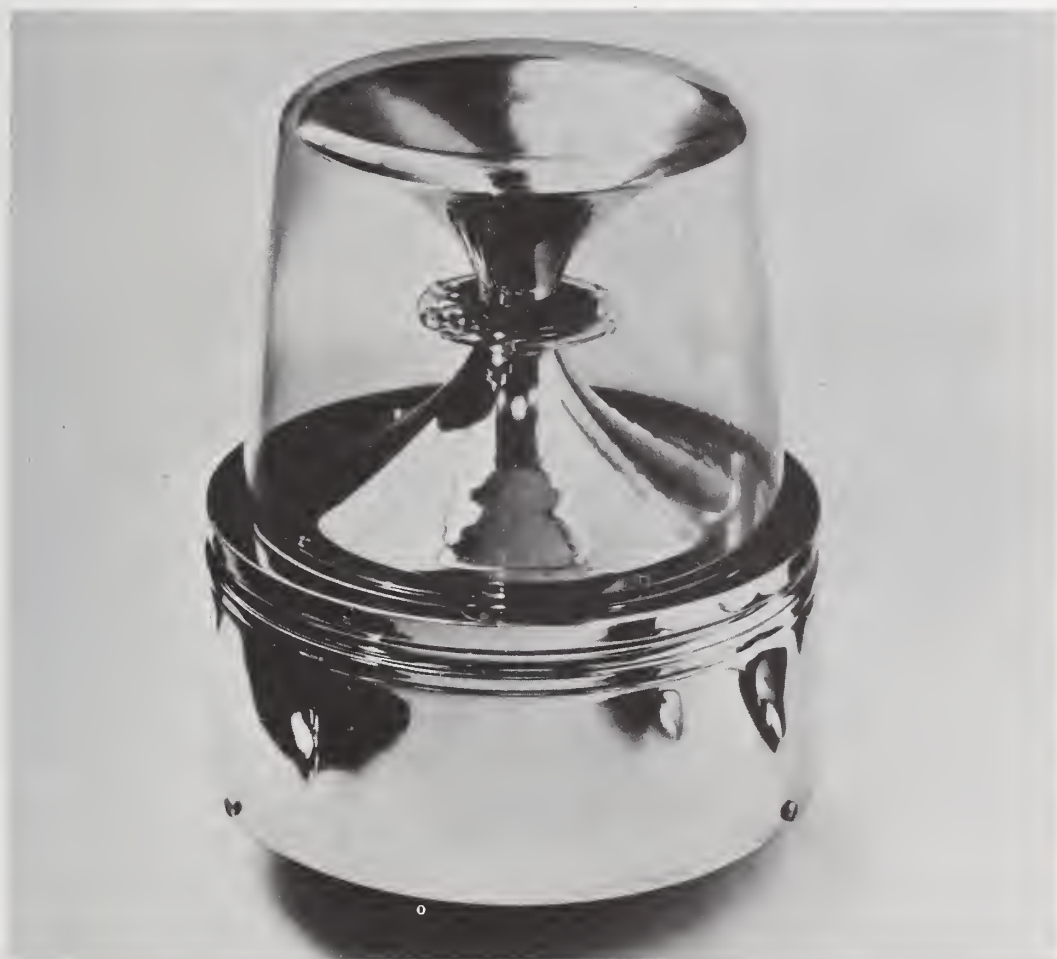
FIGURE 3.4i. Single ring-shaped xenon flashtube is energized through built-in, high-voltage, condenser-discharge circuitry, in base. Flashtube ring coincides with the focal circle of a mirror in the shape of a paraboloid of revolution, thus concentrating the light around the horizontal plane, over 360°. Clear dome is shown for clarity.
