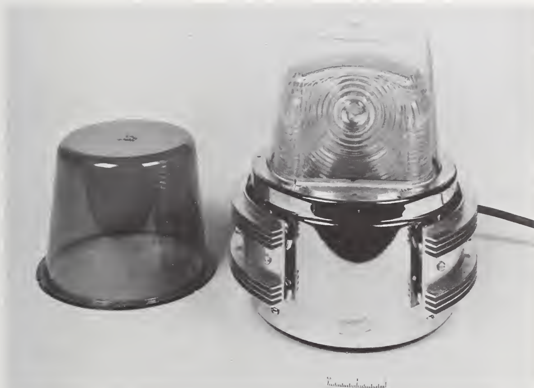
FIGURE 3.4g. Single xenon flashtube is energized through built-in, high-voltage, condenser-discharge circuitry, in base. Inner clear dome is flattened, with "hull's-eye" Fresnel lenses on both front and rear surfaces. Light emerges over 360°, but these lenses concentrate the light more strongly around the front and rear horizontal directions. The narrow side surfaces of the inner dome contain cylindrical Fresnel lenses (horizontal ridges) that concentrate the light emitted sideways around the horizontal plane. Smooth outer dome is clear, with substitutable colored outer dome also shown on the left. Also mounted under the inner dome are two small, upright, nonreflectorized incandescent lamps, one on each side. These are hurned steadily to permit continuous visibility of the unit at close ranges at night.
