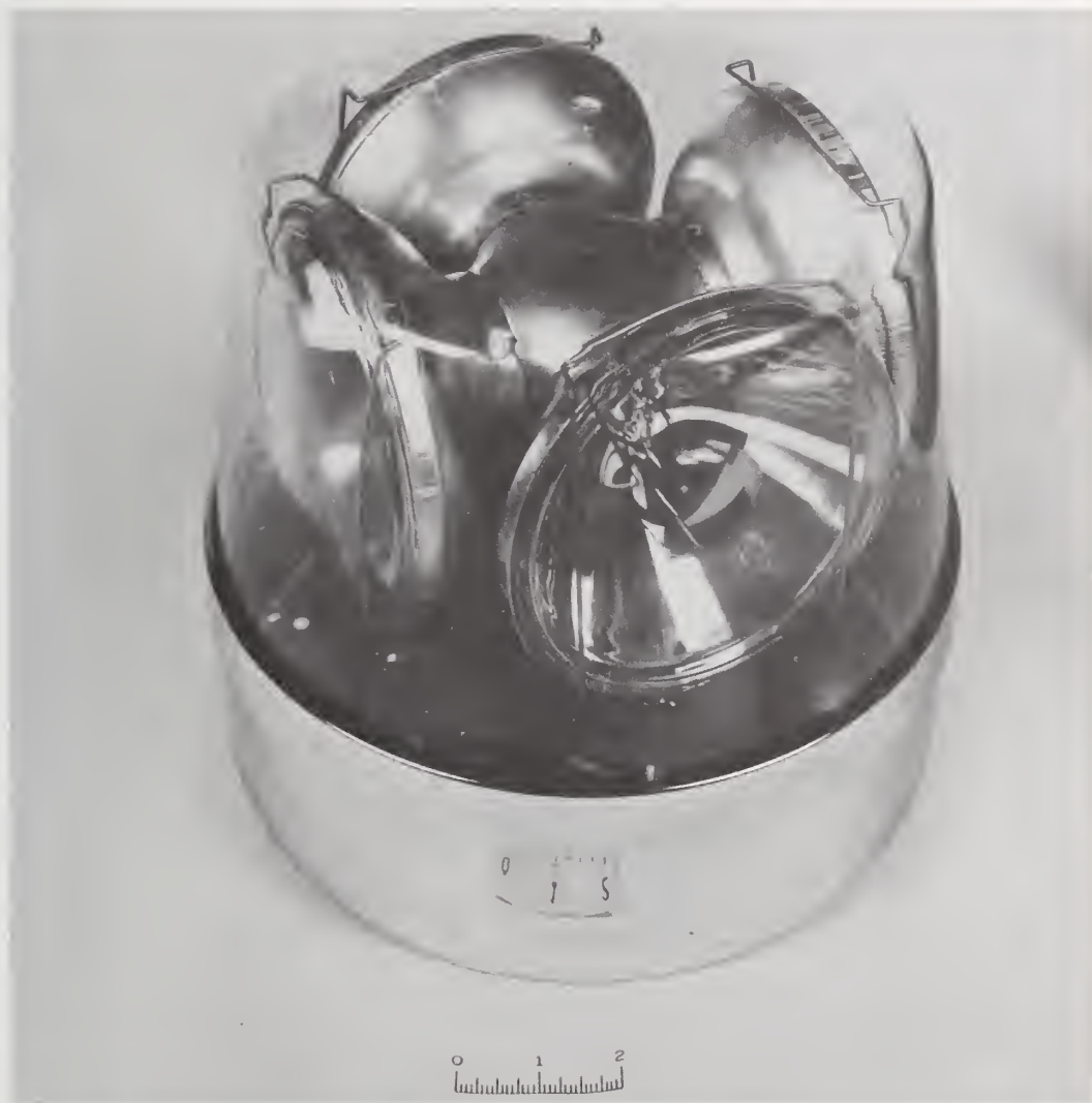
FIGURE 3.2a4. Rotating base carries four sealed beam (PAR) incandescent lamps. Unit is shown with four clear lamps under a clear dome for clarity. The units in the three preceding figures (3.2a1 through 3.2a3) contain PAR-36 lamps having a diameter of 4 1/2 in. (11.4 cm). This unit uses larger, brighter, PAR-46 lamps with a diameter of 5 3/4 in. (14.6 cm).
