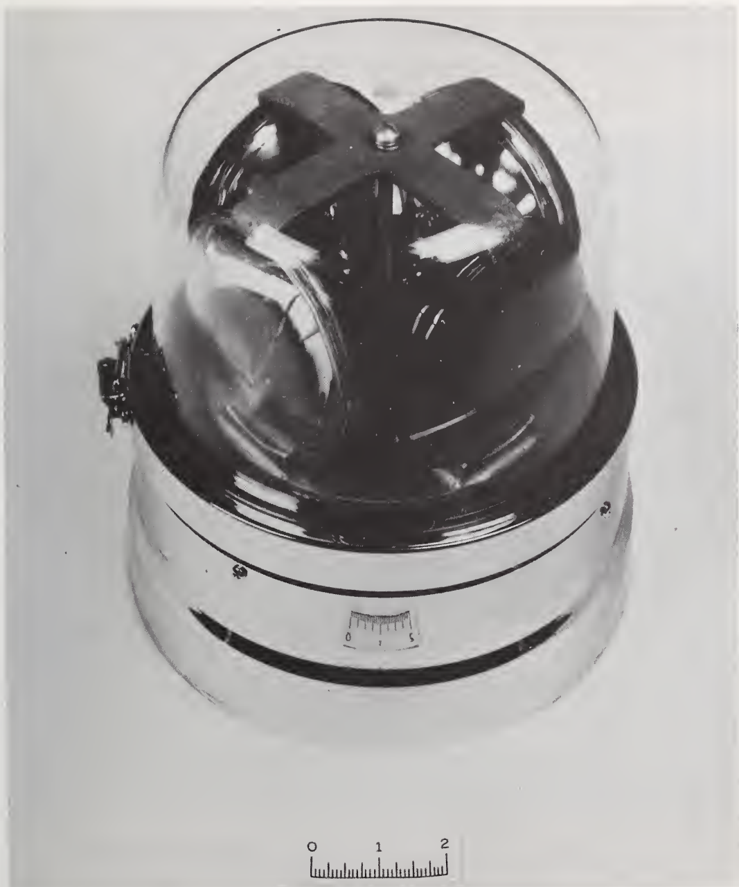
FIGURE 3.3a. Base carrying four outward-facing sealed beam (PAR) incandescent lamps oscillates horizontally back and forth over about 90^\circ . Return sweep is much faster than initial sweep. Unit shown has lamps with colored faces, under a clear dome.
