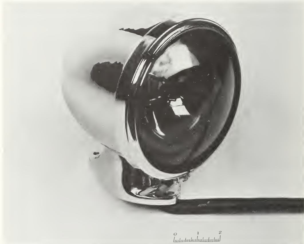
FIGURE 3.3c. Single sealed beam (PAR) incandescent lamp oscillates synchronously in both the horizontal and vertical directions, around a fixed horizontal axis. The result is a double “figure 8” pattern ( ∞∞∞ : four full up-and-down vertical oscillations to each full back-and-forth horizontal oscillation). Bullet-shaped housing is oriented horizontally, with clear (or interchangeably, colored) lens in front.
