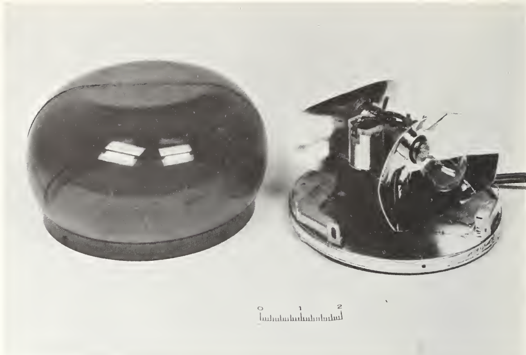
FIGURE 3.2f. Rotating base carries two nonreflectorized incandescent lamps with attached external parabolic reflectors. Unit is shown with colored dome removed for clarity. This low-profile unit is intended for use on the dashboards of part-time emergency vehicles (plugging into the cigarette lighter).
