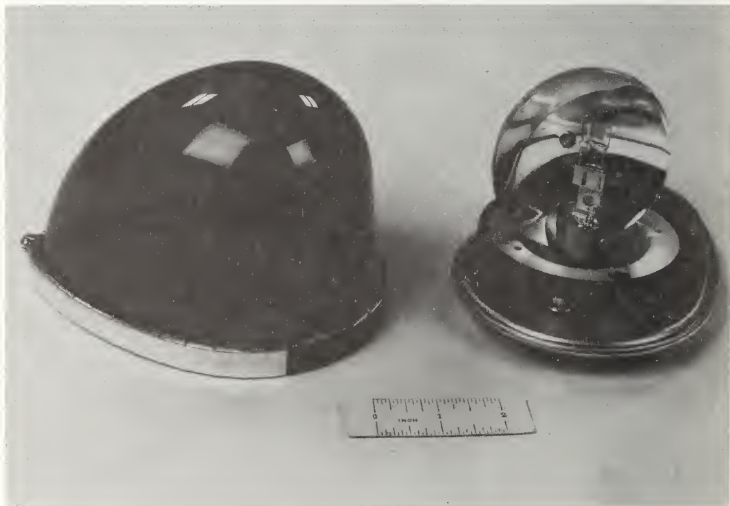
FIGURE 3.2g. Parabolic mirror rotates around a fixed, nonreflectorized, clear, tungsten quartz halogen lamp with its axis vertical. Unit shown has an upright lamp under a teardrop-shaped colored dome (shown removed for clarity) that is presumably meant to cut air resistance at high speeds. This unit is similar to that shown in figure 3.2e2, except for the lamp type.
