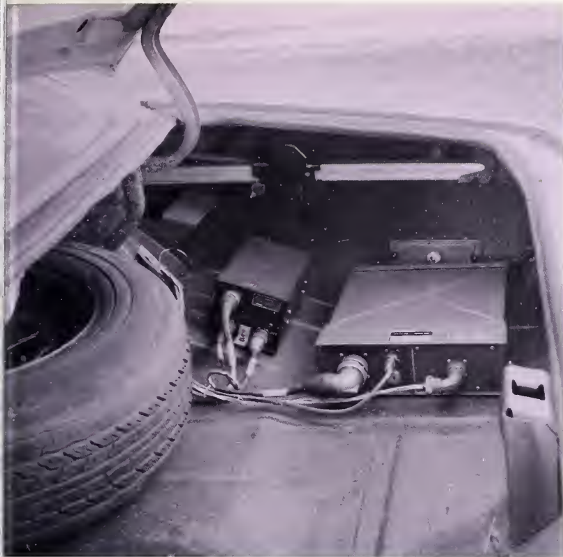
Figure 10. In a dead-reckoning system, a data processor (left) is used in conjunction with a transceiver (right) to send location information to the computer at the base station. (Photograph courtesy of the Boeing Co.).
