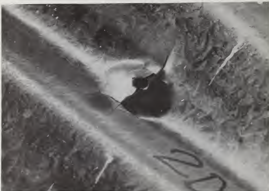
Fig. 32. Typical fatigue failure of CGI cladding
