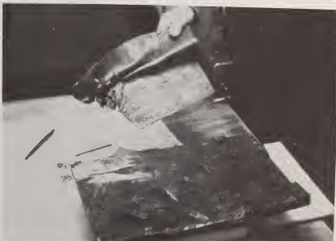
Figure 29 Incienso Dislodged Neoprene Bearing Pad
