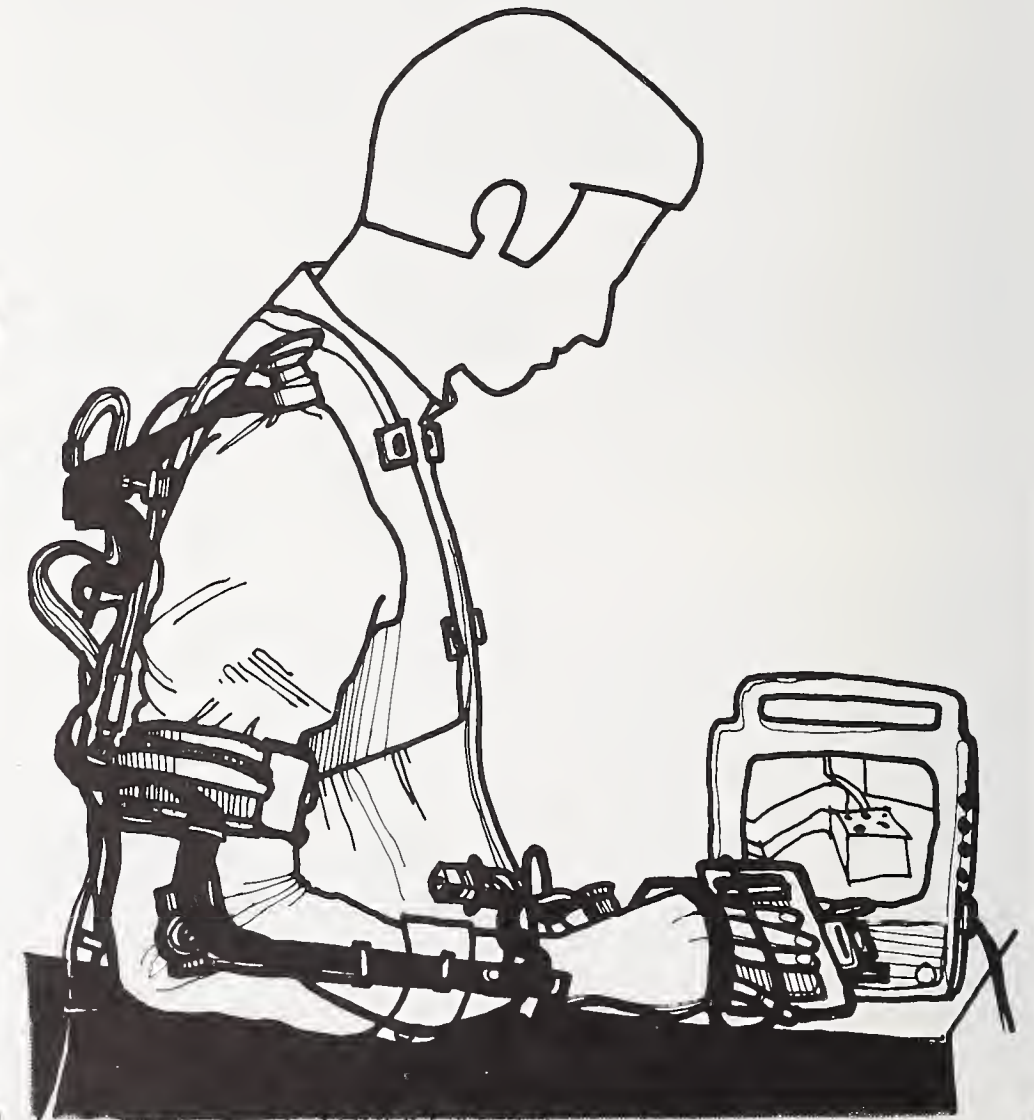
Array of airjets, connecting tubes, and hand holder used to present tactile dot patterns.
