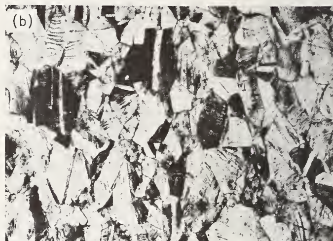
Figure 2. Microstructure of two identical 180° stainless steel spline plates. Note the highly cold worked structure of one plate (a) in contrast to the annealed and cold finished structure of the other (b). The plate whose microstructure is shown in (b) failed via a fatigue mode.
