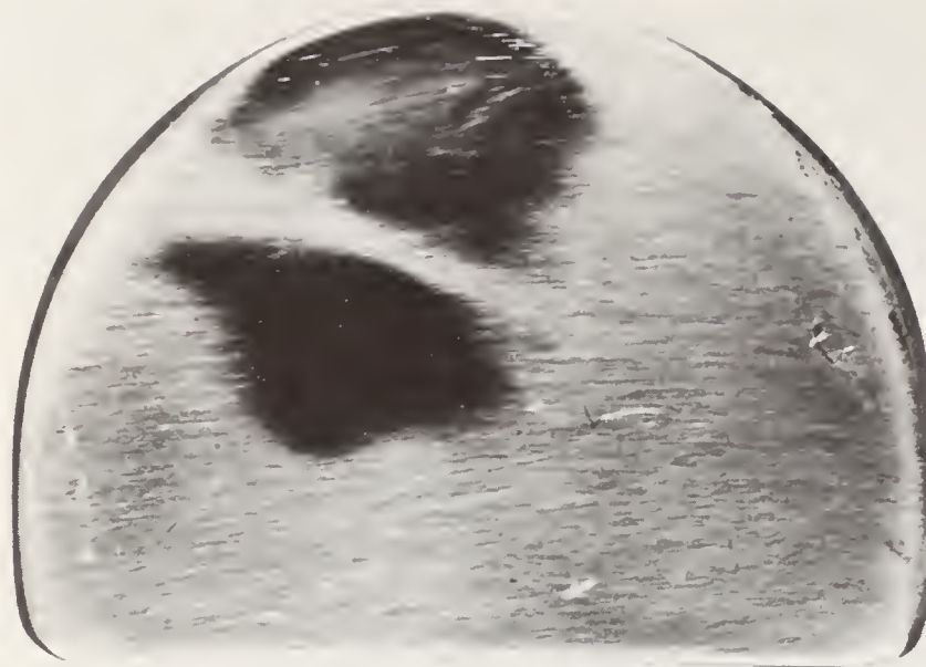
Figure 1. Wear on the surface of a titanium tibial plateau prosthesis.
