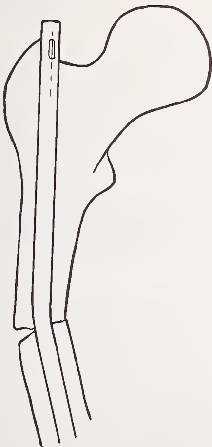
Figure 3. This tracing of an x-ray shows the bend suffered by a 9 mm cloverleaf nail when the patient put on his pants while standing up at 3 weeks post-operatively.
