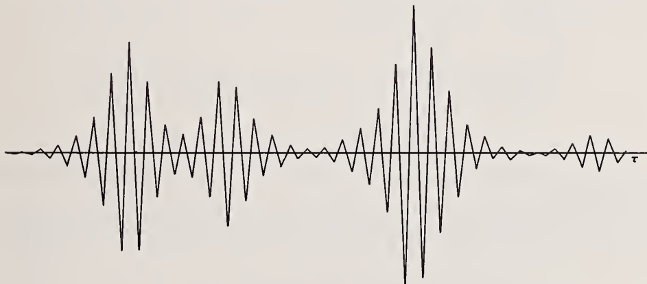
Figure 4a. Representation of R_{xy}(\tau) , the cross-correlation function.
