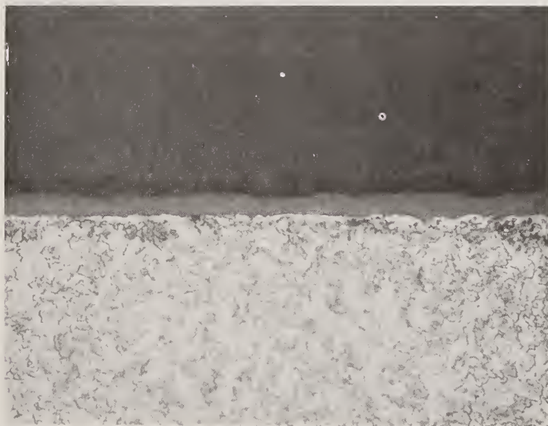
FIGURE 9. PHOTOMICROGRAPH OF VAPOR DEPOSITED ALUMINA COATING ON EXTRUSION PARTS
