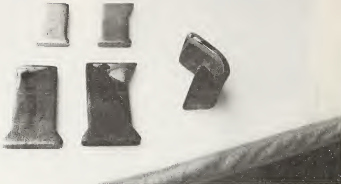
Figure 17 : Stamped Hammers with and without the Stellite hard facing. The bent hammer shows the ductility of stainless 316.
