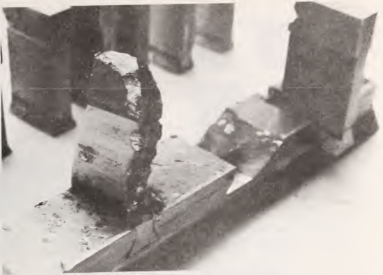
Figure 15 : Damage done to the knife bar and other hammers because of breakage.
