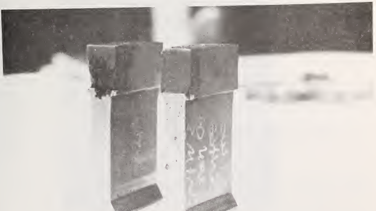
Figure 16 : Failure of the hammers with carbide insert.
