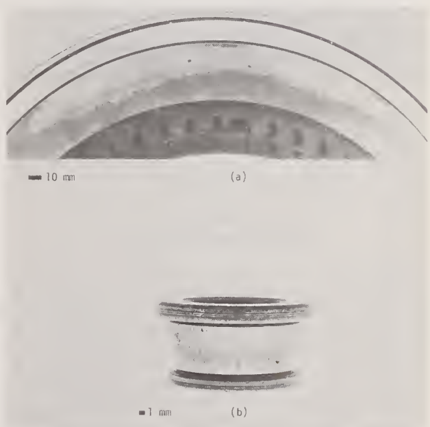
FIGURE 24. Microspalling (peeling) on a 12 in (305 mm) O.D. double cup in (a) and a 3/4 in (19 mm) bore cone in (b).
