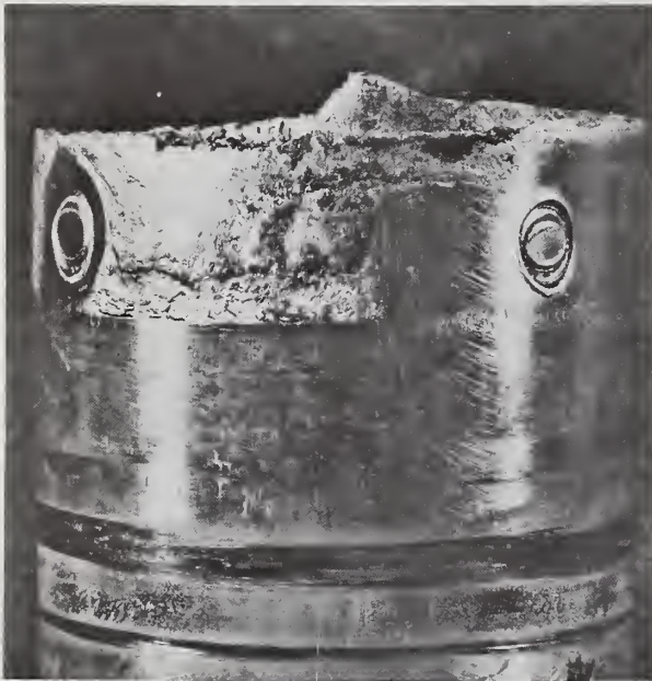
FIGURE 23. Severe fretting on a 10 cm diameter fan drive shaft where a collar contacted the shaft.
