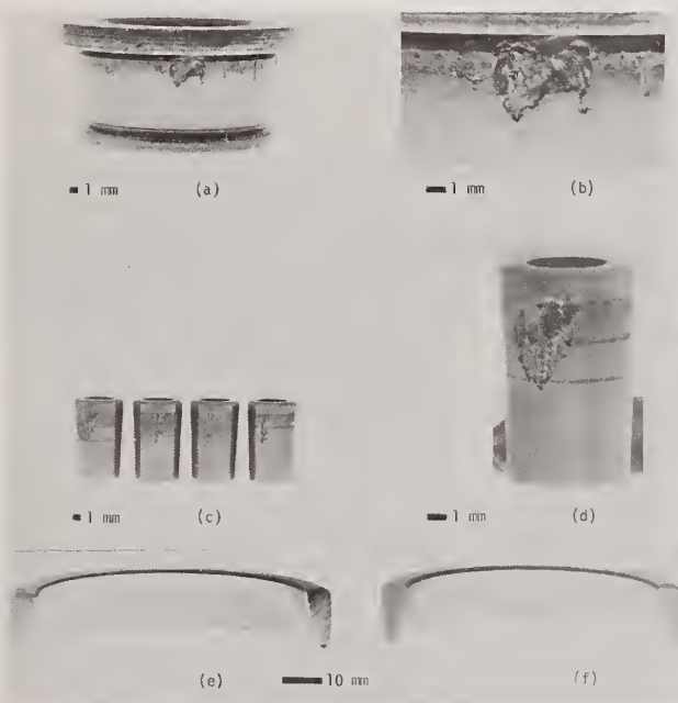
FIGURE 20. Geometric stress concentration fatigue. (a, b) Cone (inner race) with GSC fatigue at the undercut. (c, d) Rollers from the cone in (a, b) with GSC where the roller contacted the edge of the cone race. (e) Cup or outer race with load zone typical of misaligned cup with microspalling at the edge of the raceway. (f) Another cup with the same amount of misalignment (0.007 in/in) but with twice the load as in (e).
