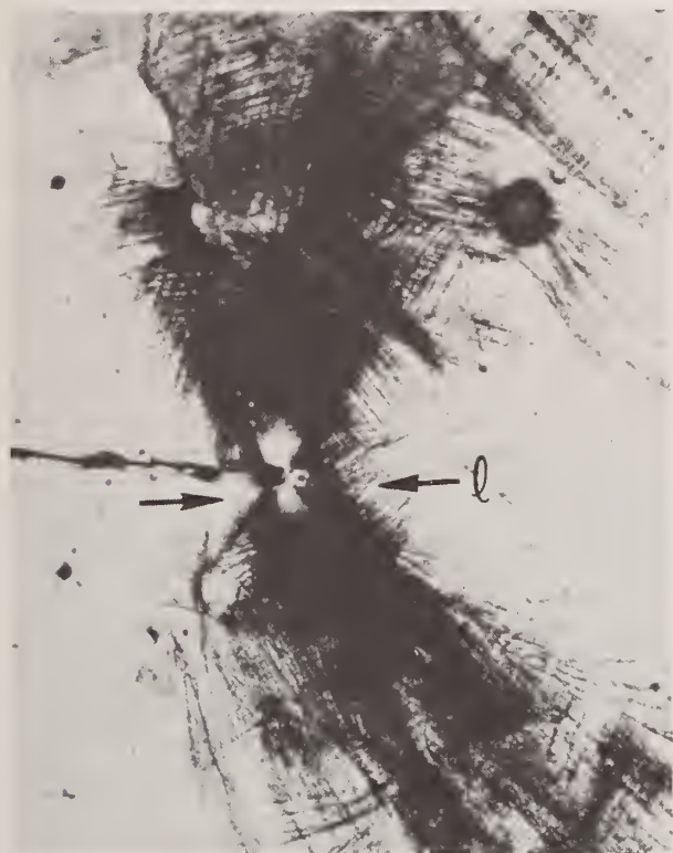
FIGURE 2. Plastic zone at a sharp crack tip in an iron-3 percent silicon alloy revealed by etch-pitting of sample loaded to (K_I/Y)=0.38 \sqrt{\text{in.}} , \times 200 .
