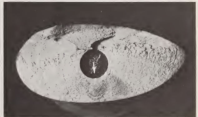
FIGURE 9. Surface of the fracture of figure 8 showing that the fatigue cracks started at the surface of the central hole.
