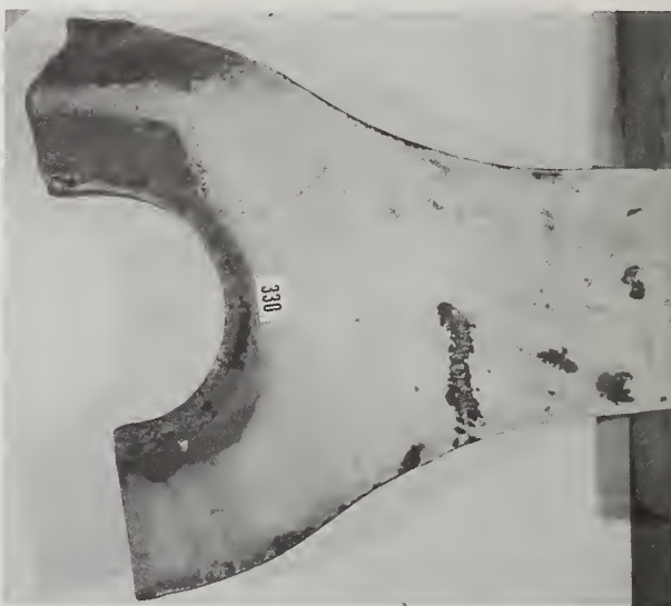
FIGURE 4. Portion of an eyebar from the Point Pleasant, W. Va. bridge. This fracture caused the collapse of the bridge.
