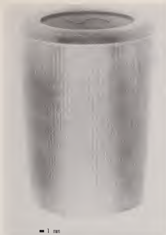
FIGURE 10. Fretting damage on a roller that closely resembles fluting damage caused by electrical current. The mechanism suggested is excessive vibration under thin EHD film conditions.
