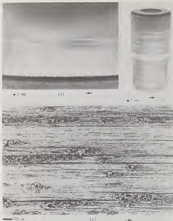
FIGURE 4. Adhesive wear caused by high speed skidding on a cone race in (a) and (c).
