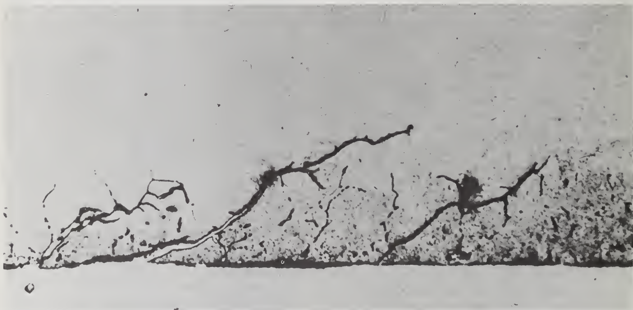
FIGURE 9. Micrograph of typical cracks originating at surface of gear teeth.
