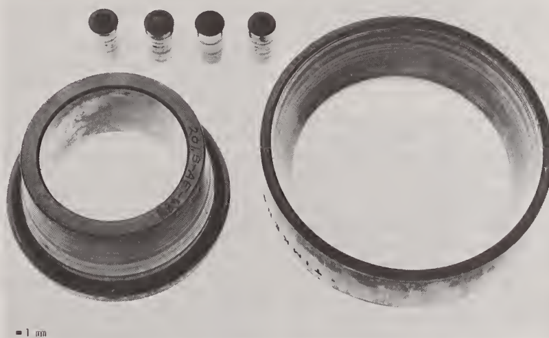
FIGURE 3. Abrasive wear caused by third particles. Natural diamond dust (0.5 \mu\text{m} size) was deliberately introduced into the lubricant in a controlled test. Damage consisted of grooving of the raceway contacts and excessive wear of the rib and roller ends.
